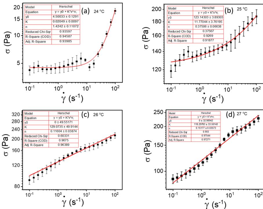
Fig. 3 (a–d) represents HB model fitting of flow curves for 20% PF127 at temperatures varying from 23 to 27 °C, respectively.
