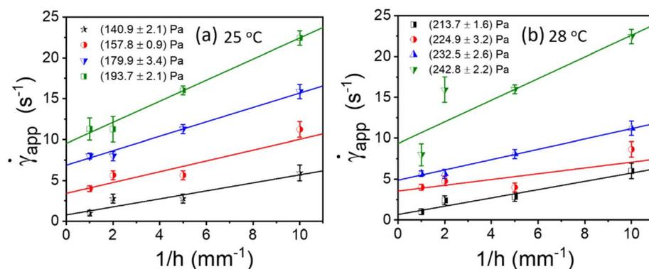
Fig. 5 (a and b) Mooney's plots for PP-40 geometry between apparent shear ( $\dot{\gamma}_{app}$ ) rate and reciprocal of the gap between two parallel plates ( $1/h$ ) for different shear stress at different temperatures from 25 to 28 °C, respectively. Different colour lines represent the straight line fit to each data set for different shear stress values, and the symbols and error bars represented here are the mean and standard deviation of three sets of measurements in each gap size.
