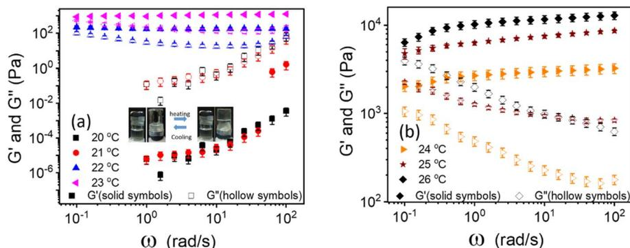
Fig. 1 (a and b) Frequency-dependent moduli storage modulus ( $G'$ ) and loss modulus ( $G''$ ) in the linear viscoelastic region (shear strain ( $\gamma = 0.1\%$ )) for 20 wt% PF127 at varying temperatures from 20 to 26 °C.
