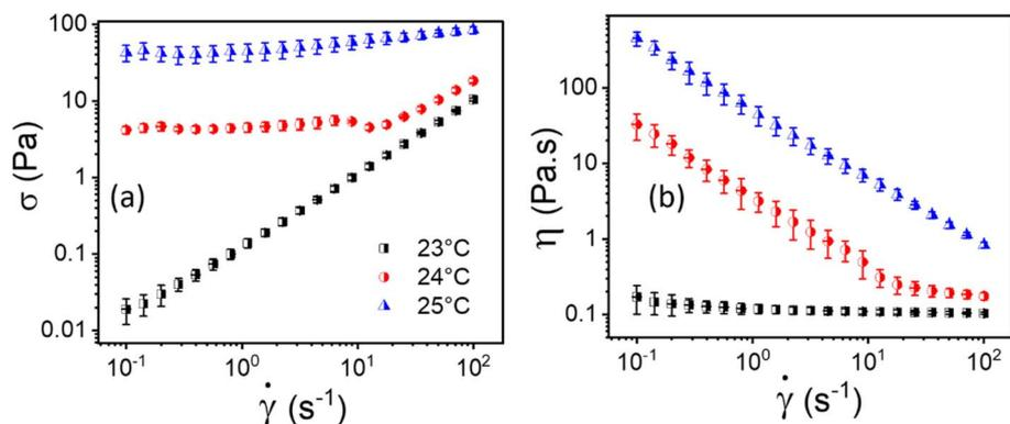
Fig. 2 Flow curves, *i.e.*, (a and b) represents shear stress ( $\sigma$ ) and viscosity ( $\eta$ ) as a function of shear rate ( $\dot{\gamma}$ ), respectively, for 20% PF127 at varying temperatures of 23 °C, 24 °C and 25 °C.
