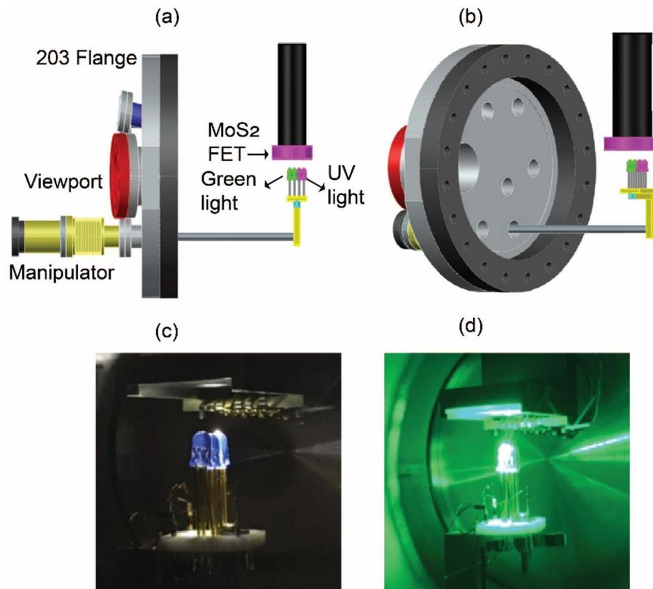
Fig. 1 Illustration of UV and green light irradiation system inside the *in situ* chamber: (a) side view, (b) angle view, (c) UV light irradiation of the MoS<sub>2</sub>-FET, and (d) green light irradiation of the MoS<sub>2</sub>-FET.
