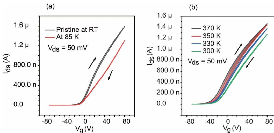
**Fig. 3** Series of  $I_{ds}$ - $V_g$  curves for  $V_{ds} = 50$  mV in dark conditions at various temperatures. (a) RT (black) to 85 K (red) for the cooling experiment. (b) 370 (black) to 300 K (green) after the baking procedure. The  $V_g$  sweep started from  $-70$  V and was ramped at a rate of  $5$  V s<sup>-1</sup>. The sweep directions of  $V_g$  are indicated by the arrows.
