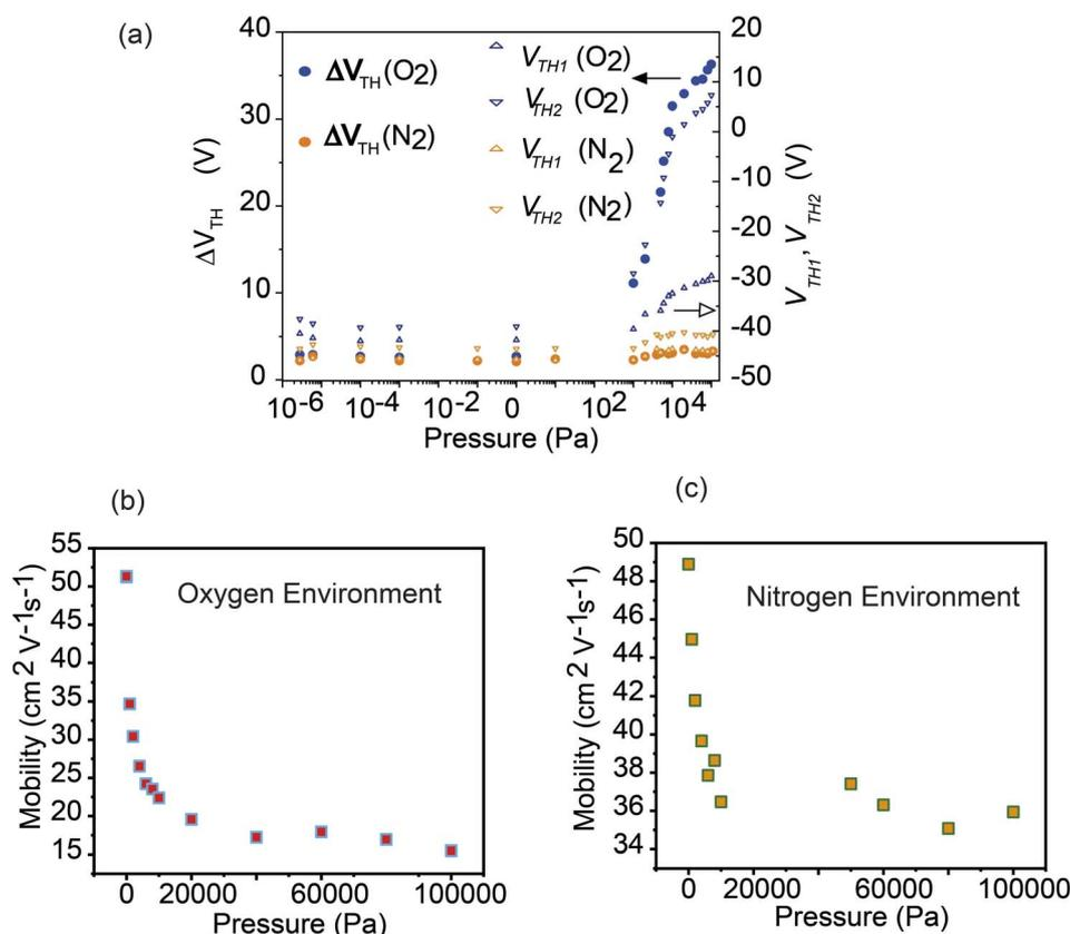
Fig. 6 (a) The threshold gate voltages  $V_{\text{th1}}$ ,  $V_{\text{th2}}$  (open triangles) and  $\Delta V_{\text{th}} = V_{\text{th2}} - V_{\text{th1}}$  (filled circles) as functions of relative gas pressure. (b) Mobility as a function of oxygen pressure. (c) Mobility as a function of nitrogen pressure.
