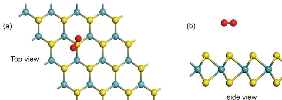
Fig. 8 Optimized model of the interaction between MoS<sub>2</sub> and oxygen: (a) top view; (b) side view.
