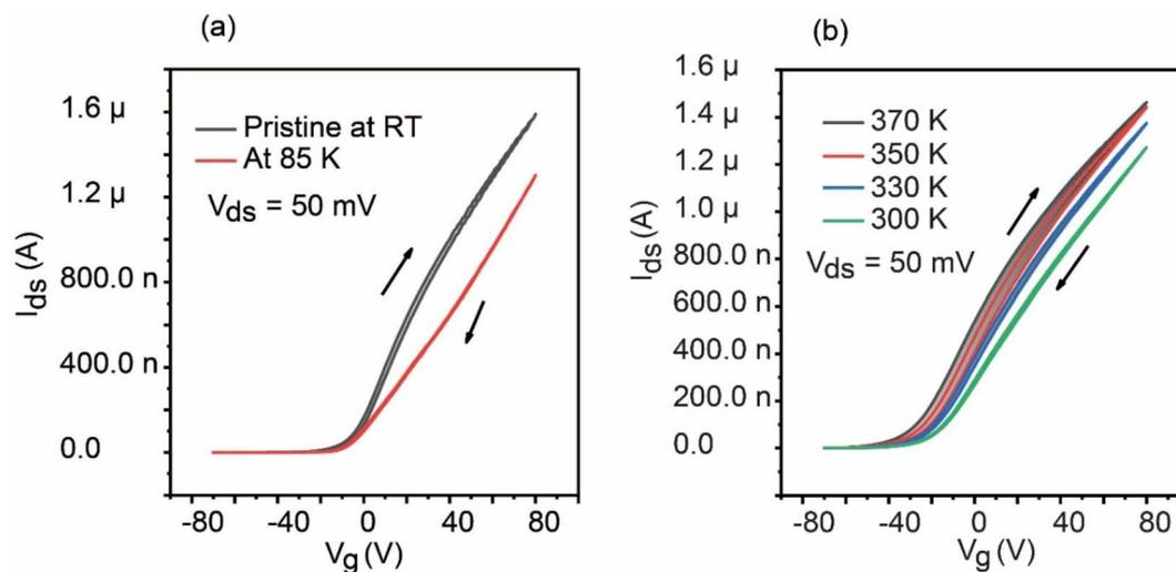
**Fig. 3** Series of  $I_{ds}$ - $V_g$  curves for  $V_{ds} = 50$  mV in dark conditions at various temperatures. (a) RT (black) to 85 K (red) for the cooling experiment. (b) 370 K (black) to 300 K (green) after the baking procedure. The  $V_g$  sweep started from  $-70$  V and was ramped at a rate of  $5$  V s<sup>-1</sup>. The sweep directions of  $V_g$  are indicated by the arrows.
