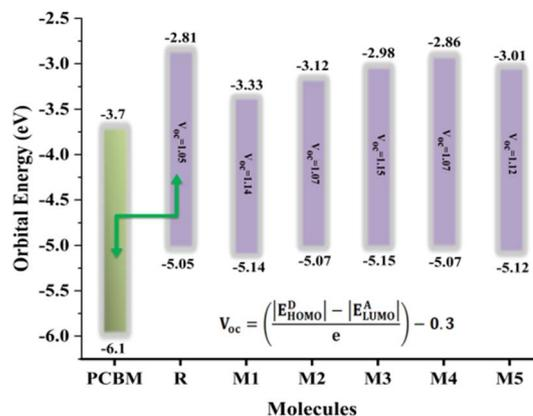
**Fig. 4**  $V_{oc}$  values of reference molecule R and all designed molecules (M1–M5) calculated with regard to the PCBM.
