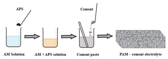
Fig. 15 Synthetic scheme for the preparation of the PAM-Portland cement electrolyte.
