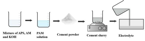
Fig. 17 Schematic diagram of the cement electrolyte
