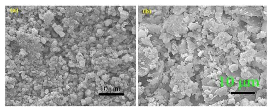
Fig. 9 SEM micrographs of (a) Portland cement and (b) Portland cement with Na<sub>2</sub>SO<sub>4</sub> alkali salt. Reproduced from ref. 45 with permission from Elsevier, copyright 2024.
