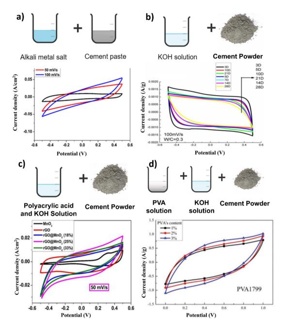
Fig. 8 Schematic methods of synthesis of concrete-based electrolyte and its CV graphs. Reproduced from ref. 45, 96, 111 and 112 with permission from (a) Elsevier, (b) IOP, (c) RSC, (d) SAGE, copyright 2024.
