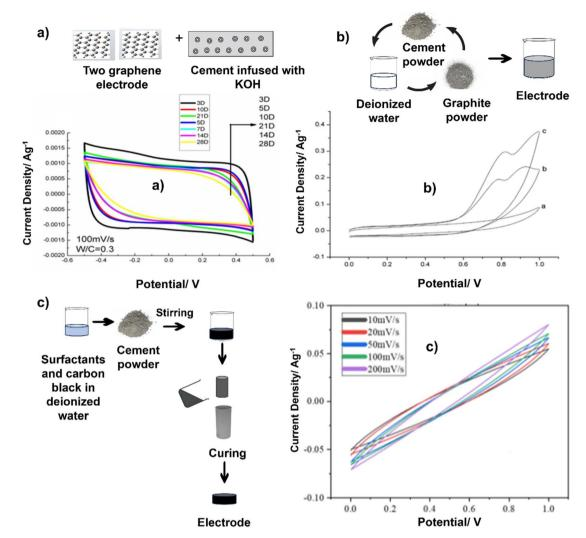
Fig. 4 Schematic methods of synthesis of the concrete-based electrodes and their CV graphs. Reproduced from ref. 96–98 with permission from (a) IOP, (b and c) Elsevier, copyright 2024.
