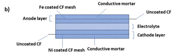
Fig. 3 A visual representation depicting the conceptual design of an energy storage device created through (a) the powder mixing process and (b) the metal coating process.
