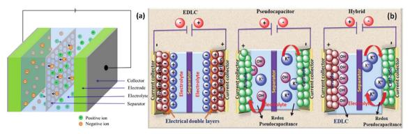
Fig. 2 Schematic representations showing (a) components of supercapacitor. Reproduced from ref. 10 with permission from Elsevier, copyright 2024 and (b) types of supercapacitors. Reproduced from ref. 11 with permission from RSC, copyright 2024.
