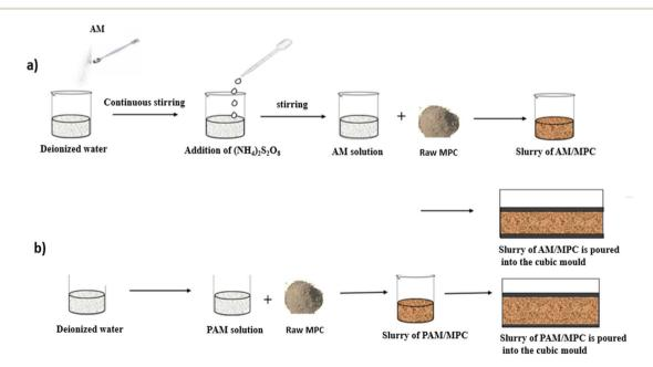
Fig. 19 Two distinct methods were utilized for the fabrication of PAM/MPC composite electrolytes. (a) *In situ* Polymerized Solid Electrolyte (IPSE) and (b) Directly Added Solid Electrolyte (DASE).
