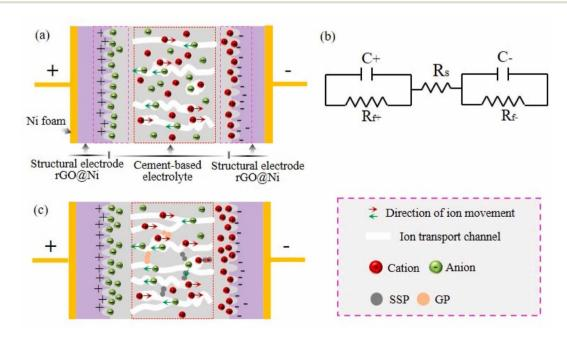
Fig. 21 Schematic diagrams of (a) the SSCs with pure cement-based electrolyte paste, (b) equivalent circuit model, and (c) the SSCs with the cement-based electrolyte pastes containing SSP and GP. Reproduced from ref. 156 with permission from Elsevier, copyright 2024.
