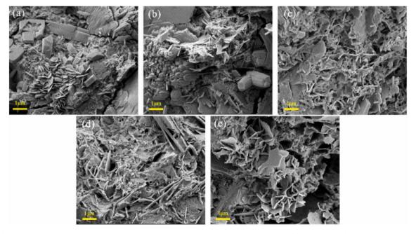
Fig. 13 (a) SEM images of various redox-active cement composites (a) KFCN-0, (b) KFCN-0.02, (c) KFCN-0.04, (d) KFCN-0.06, (e) KFCN-0.08. Reproduced from ref. 125 with permission from Elsevier, copyright 2024.
