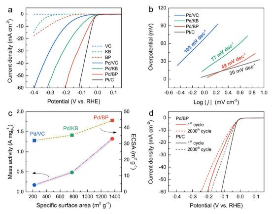
Fig. 4 Electrochemical tests in an  $N_2$ -saturated 0.5 M  $H_2SO_4$  solution towards HER of the Pd/VC, Pd/KB, Pd/BP, and commercial Pt/C; (a) LSV curves, (b) Tafel plots, (c) mass activity at an overpotential of 200 mV and ECSA versus specific surface area (circle and square symbols represent mass activity and ECSA, respectively), and (d) stability tests of Pd/BP and Pt/C: LSV curves before and after 2000 cycles.
