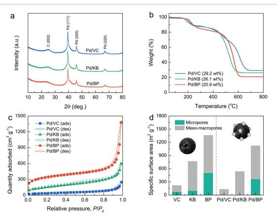
Fig. 3 (a) XRD patterns and (b) TGA curves measured at 50-800 °C under  $O_2$  atmosphere, (c)  $N_2$  adsorption–desorption isotherms (solid and open symbols represent the adsorption and desorption isotherms, respectively), and (d) the specific surface areas contributed by micropores (internal pores) and meso–macropores (external pores) of Pd/VC, Pd/KB, and Pd/BP.
