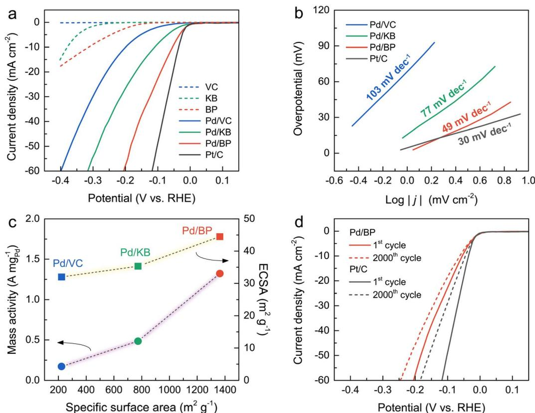
Fig. 4 Electrochemical tests in an N<sub>2</sub>-saturated 0.5 M H<sub>2</sub>SO<sub>4</sub> solution towards HER of the Pd/VC, Pd/KB, Pd/BP, and commercial Pt/C: (a) LSV curves, (b) Tafel plots, (c) mass activity at an overpotential of 200 mV and ECSA versus specific surface area (circle and square symbols represent mass activity and ECSA, respectively), and (d) stability tests of Pd/BP and Pt/C: LSV curves before and after 2000 cycles.
