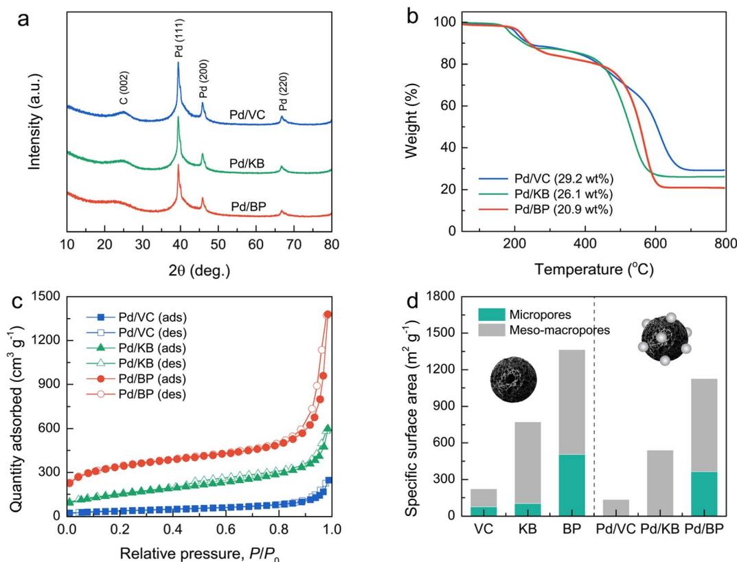
Fig. 3 (a) XRD patterns and (b) TGA curves measured at 50–800 °C under O<sub>2</sub> atmosphere, (c) N<sub>2</sub> adsorption-desorption isotherms (solid and open symbols represent the adsorption and desorption isotherms, respectively), and (d) the specific surface areas contributed by micropores (internal pores) and meso-macropores (external pores) of Pd/VC, Pd/KB, and Pd/BP.
