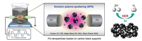
Fig. 1 A schematic of the experimental setup of SPS for preparation of Pd nanoparticles loaded on CB supports in this work.
