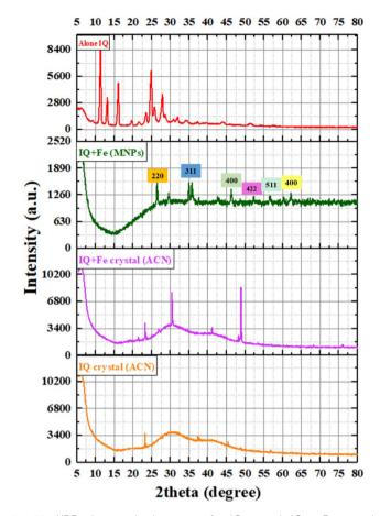
Fig. 35 XRD characterisation curve for IQ crystal, IQ + Fe crystal, MNPs, and alone IQ.
