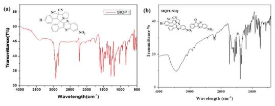
Fig. 2 FT-IR spectra for stretching and bending (a) SIQPI alone (b) SIQPI + NIQ.
