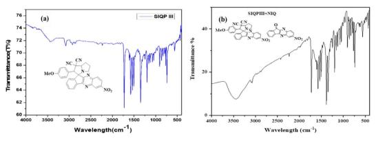
Fig. 4 FT-IR spectra for stretching and bending (a) SIQPIII alone and (b) SIQPIII + NIQ.
