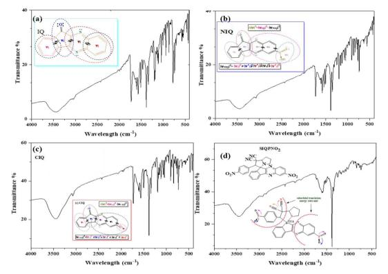
Fig. 1 FT-IR spectra for stretching and bending of (a) IQ, (b) NIQ, (c) CIQ, and (d) SIQPNO<sub>2</sub>.
