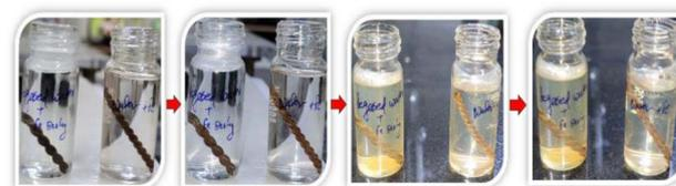
Fig. 38 Effect in degassed and distilled water on rusting with Fe scrap.
