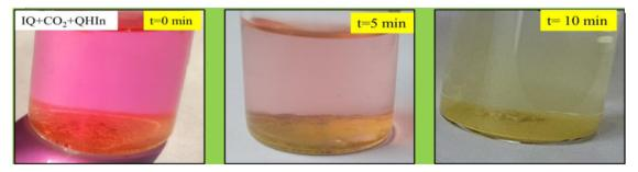
Fig. 16 QHIn PCR using IQ with  $CO_2$  at t = 0, 5, and 10 min.
