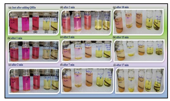
Fig. 39 Images of (i) IQ + Fe in aq, (ii) aq IQ only, (iii) IQ + Fe in degassed water, (iv) IQ in ACN, (v) IQ + Fe in ACN (a) initial and after (b) 1, (c) 2, (d) 3, (e) 5, (f) 7, (g) 10, (h) 15, and (i) 17 min.
