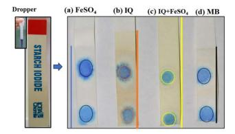
Fig. 37 Starch-iodide paper detect the absence of oxidizing agents. (a) MB + FeSO $_4$  on starch paper. (b) MB + IQ on starch paper. (c) MB + IQ + FeSO $_4$  on starch paper. (d) Only MB on starch paper.
