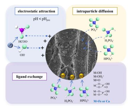
Fig. 5 Mechanism of phosphorus adsorption by FCBC
