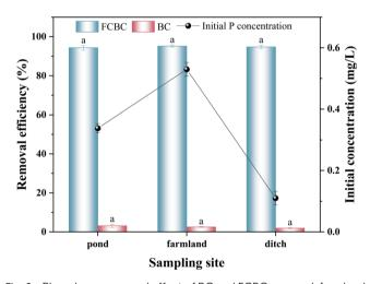
Fig. 6 Phosphorus removal effect of BC and FCBC on pond, farmland, and ditch water, different letters for the same type of biochar indicate significant differences in removal efficiency at different sampling sites (P < 0.05, Duncan's test).
