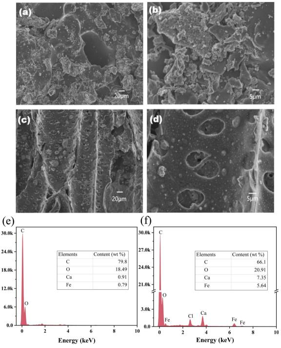
Fig. 1 SEM images of BC (a and b), and FCBC (c and d) at different magnifications; EDS analysis of BC (e) and FCBC (f).
