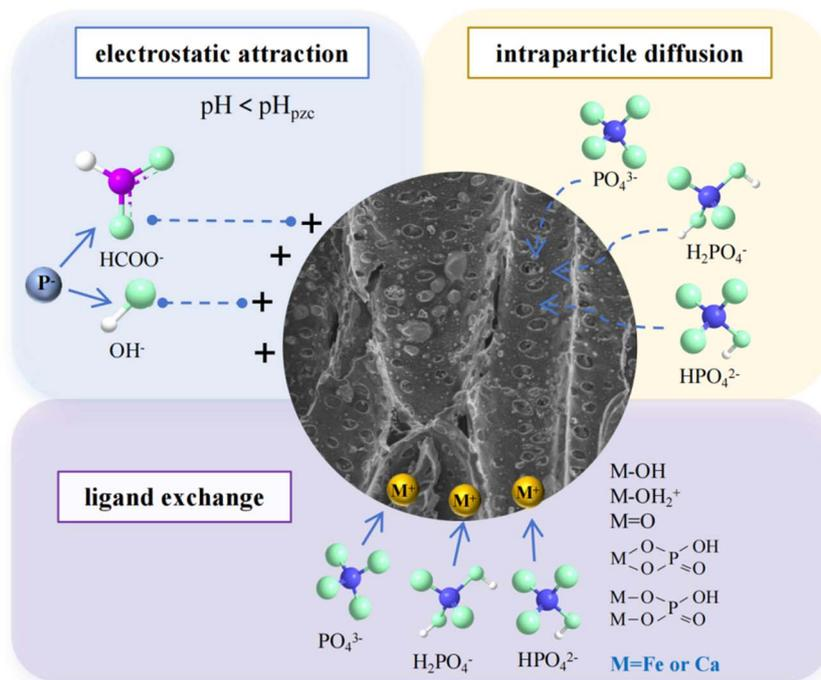
Fig. 5 Mechanism of phosphorus adsorption by FCBC.
