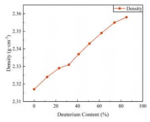
Fig. 7 Density of  $K(D_xH_{1-x})_2PO_4$  crystals at 30.2 °C.
