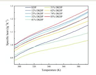
Fig. 8 Temperature dependence of the specific heat of DKDP crystals with different deuteration contents.
