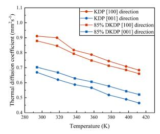
Fig. 9 Thermal diffusion coefficient of KDP crystal and 85% DKDP crystal.
