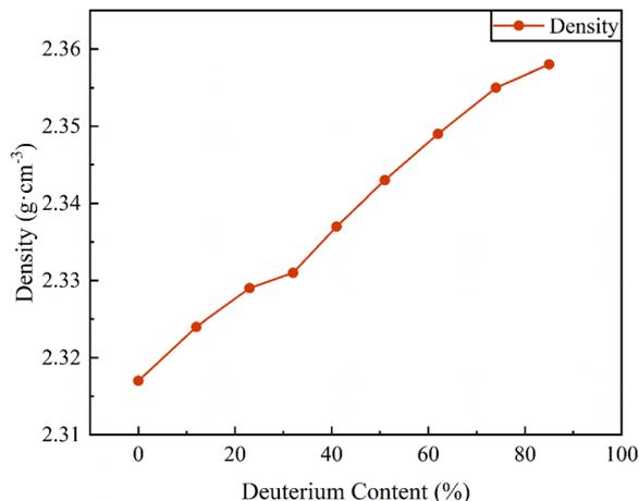
Fig. 7 Density of  $K(D_xH_{1-x})_2PO_4$  crystals at 30.2 °C.
