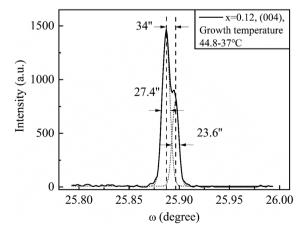
Fig. 5 Rocking curves of 12% DKDP crystal.
