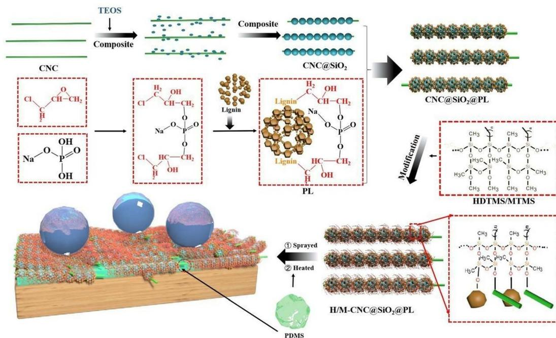
Fig. 18 Scheme for preparation of superhydrophobic coatings using cellulose nanocrystals (CNC)–SiO<sub>2</sub>–phosphorylated lignin (PL) rods.<sup>113</sup> Reproduced from ref. 113 with permission from *Polymers*, copyright 2023.
