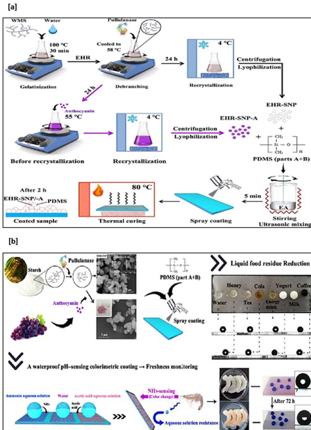
Fig. 26 (a) Schematic representation of fabricating process of EHR-SNP, EHR-SNP-A, and nano-starch-based superhydrophobic coatings. (b) Evaluation of superhydrophobicity of the coating on different consumable liquids and for acid and basic liquids enabling pH sensing property.<sup>147</sup> Reproduced from ref. 147 with permission from ACS Sustainable Chemistry & Engineering, copyright 2021.
