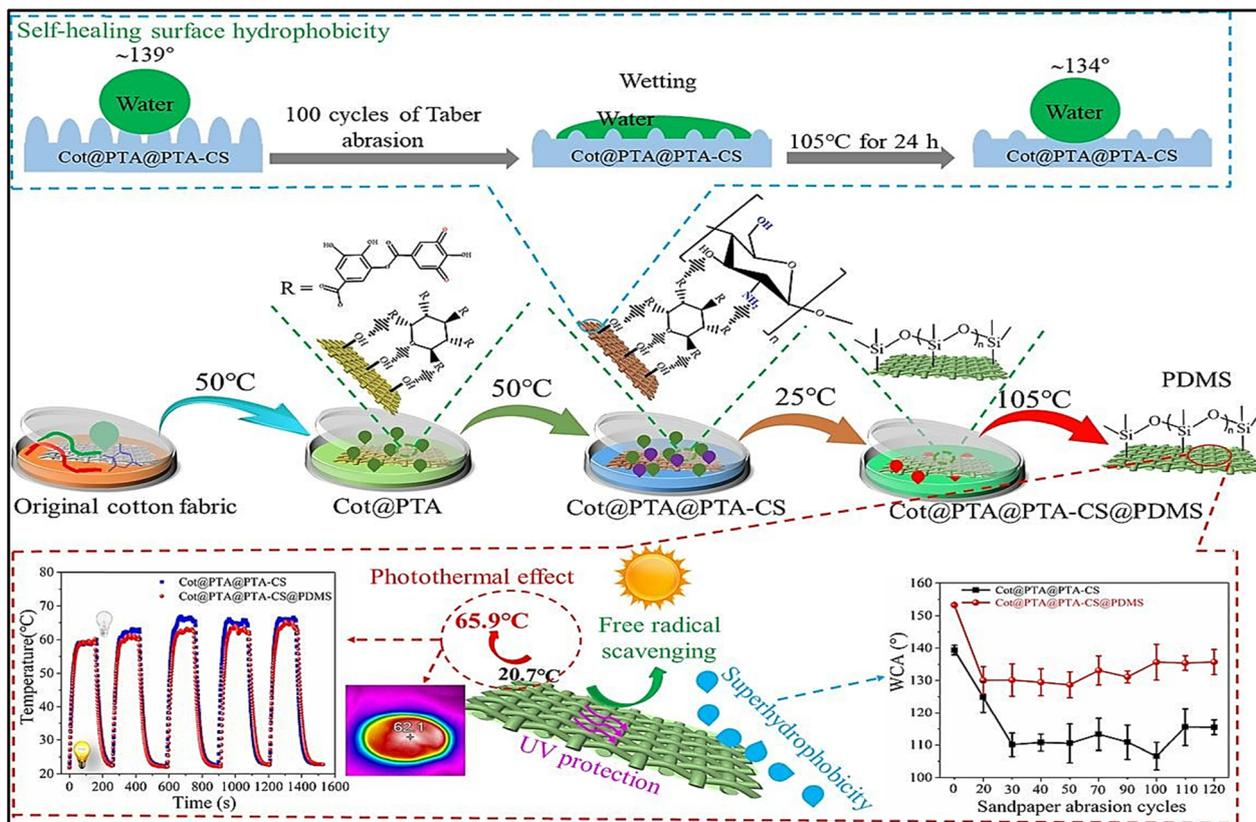
Fig. 22 Preparation demonstration of SH coating on cotton fabric using chitosan, tannic acid and polydimethylsiloxane.<sup>135</sup> Reproduced from ref. 135 with permission from *Chemical Engineering Journal*, copyright 2023.
