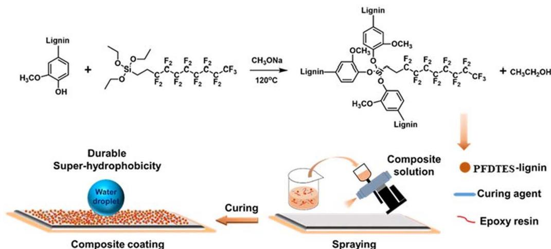
Fig. 15 Diagrammatic representation of the modification of lignin and the process of fabricating a durable superhydrophobic coating.<sup>103</sup> Reproduced from ref. 103 with permission from *Molecules*, copyright 2022.
