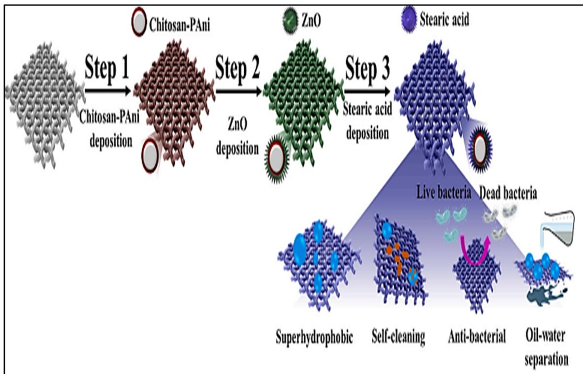
Fig. 23 Schematic preparation of superhydrophobic cotton using chitosan-PANI-ZnO-STA composite coating.<sup>136</sup> Reproduced from ref. 136 with permission from *International Journal of Biological Macromolecules*, copyright 2023.
