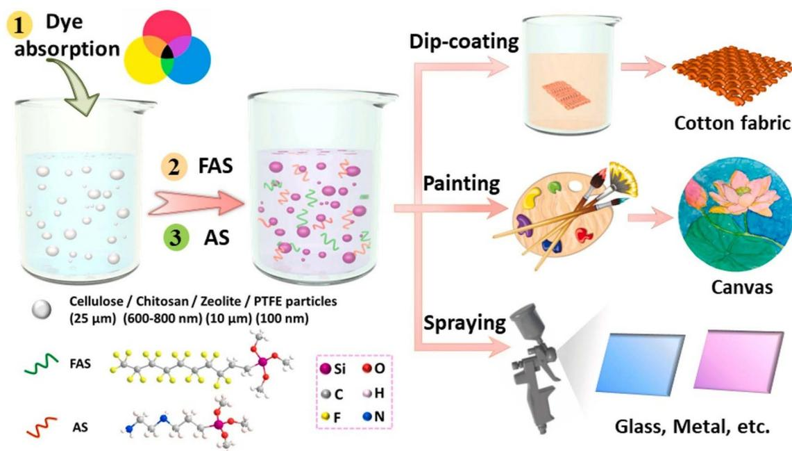
Fig. 20 A schematic representation of preparation procedure of multi-coloured superhydrophobic coatings.<sup>121</sup> Reproduced from ref. 121 with permission from *Carbohydrate Polymers*, copyright 2021.
