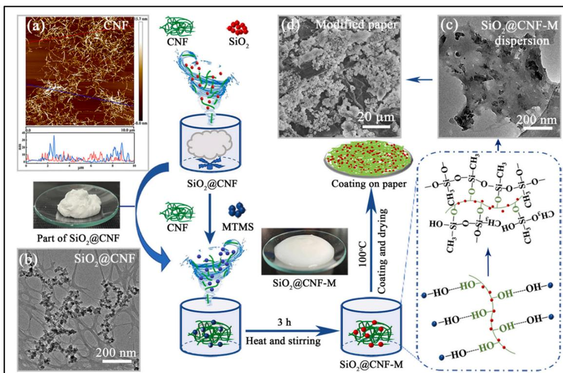
Fig. 19 Schematic representation of fabricating SiO<sub>2</sub>@CNF-M water dispersion and the coating. (a) The AFM morphology of CNF. (b) The SiO<sub>2</sub>@CNF and (c) SiO<sub>2</sub>@CNF-M water dispersion's TEM morphology. (d) SiO<sub>2</sub>@CNF-M coated on paper SEM morphology.<sup>115</sup> Reproduced from ref. 115 with permission from *Carbohydrate Polymers*, copyright 2022.
