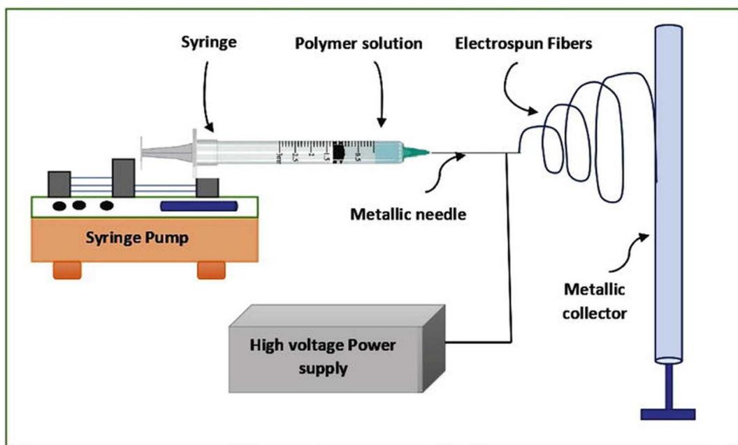
Fig. 5 Electrospinning technique.<sup>17</sup> Reproduced from ref. 17 with permission from IntechOpen, copyright 2023.
