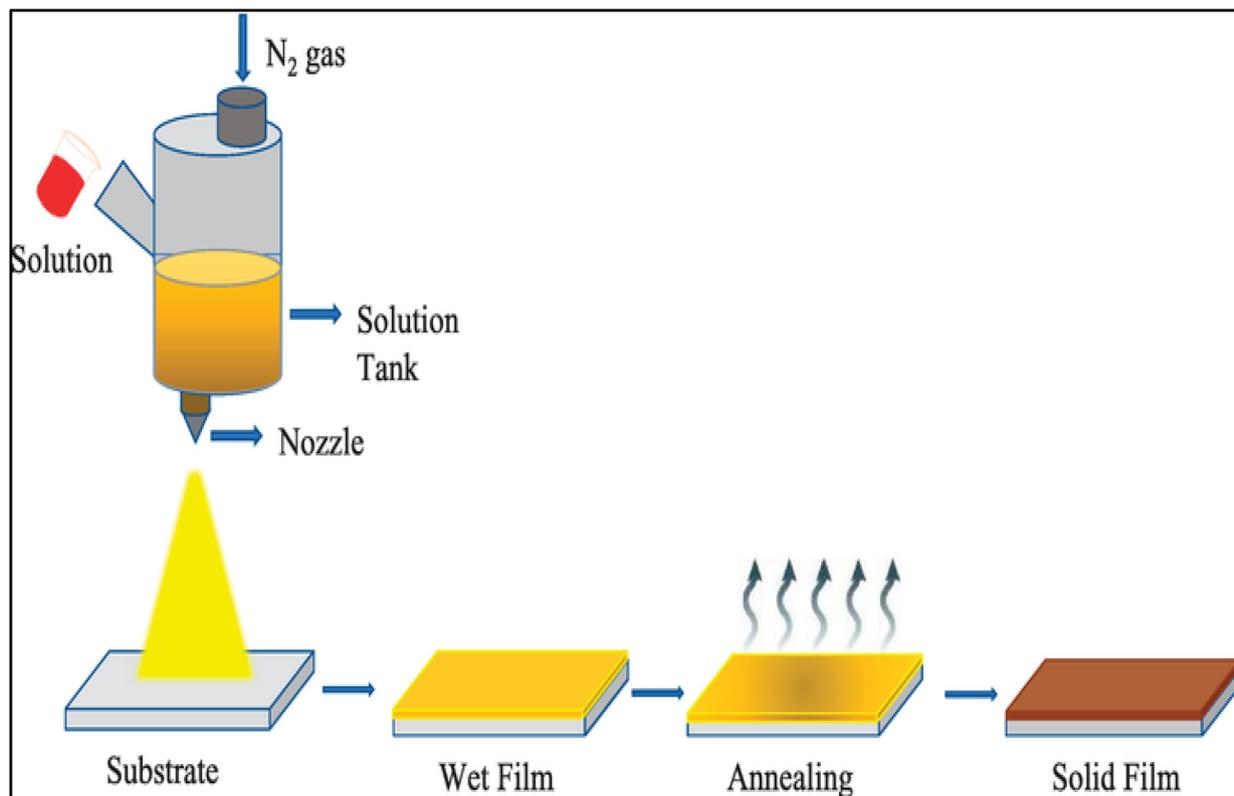
Fig. 9 Spray coating.<sup>67</sup> Reproduced from ref. 67 with permission from IntechOpen, copyright 2022.
