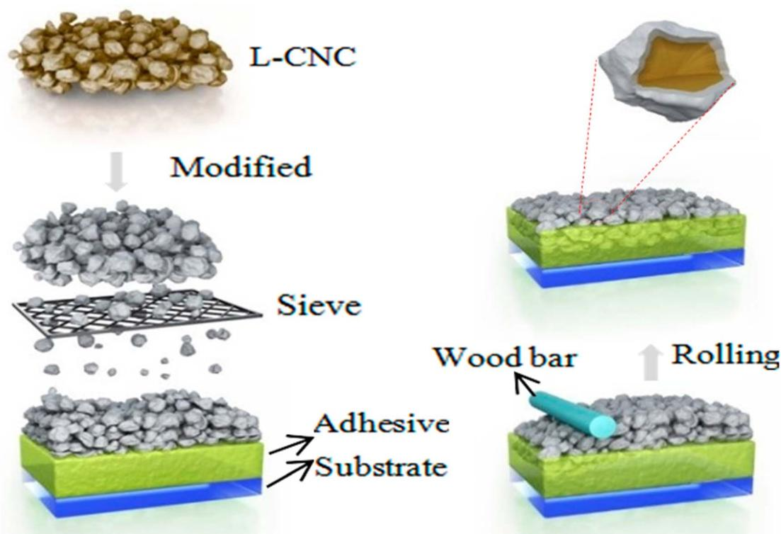
Fig. 12 Illustration displaying the procedure for developing the composite superhydrophobic coating.<sup>95</sup> Reproduced from ref. 95 with permission from *Materials*, copyright 2017.
