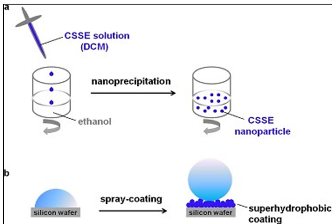
Fig. 21 (a) Demonstration of one pot method used for preparation of SH coatings using chitosan stearyl ester (CSSE). (b) Demonstration of superhydrophobic characteristics on silicon wafer.<sup>131</sup> Reproduced from ref. 131 with permission from *Carbohydrate Polymers*, copyright 2018.
