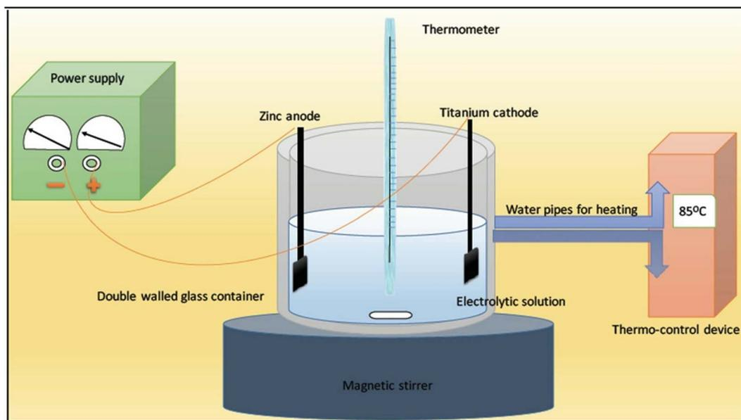
Fig. 4 Electrochemical deposition technique.<sup>31</sup> Reproduced from ref. 31 with permission from *International Journal of Implant Dentistry*, copyright 2017.
