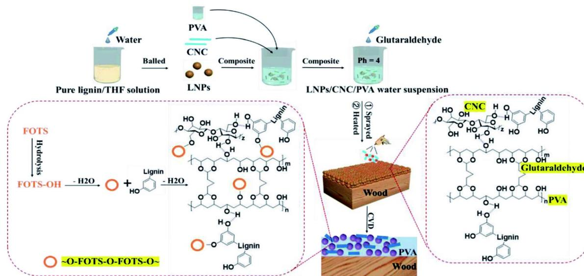
Fig. 13 Schematic representation of the steps required for developing a superhydrophobic surface based on LNPs and the possible chemical reactions that may occur (FOTS).<sup>101</sup> Reproduced from ref. 101 with permission from *RSC Advances*, copyright 2022.
