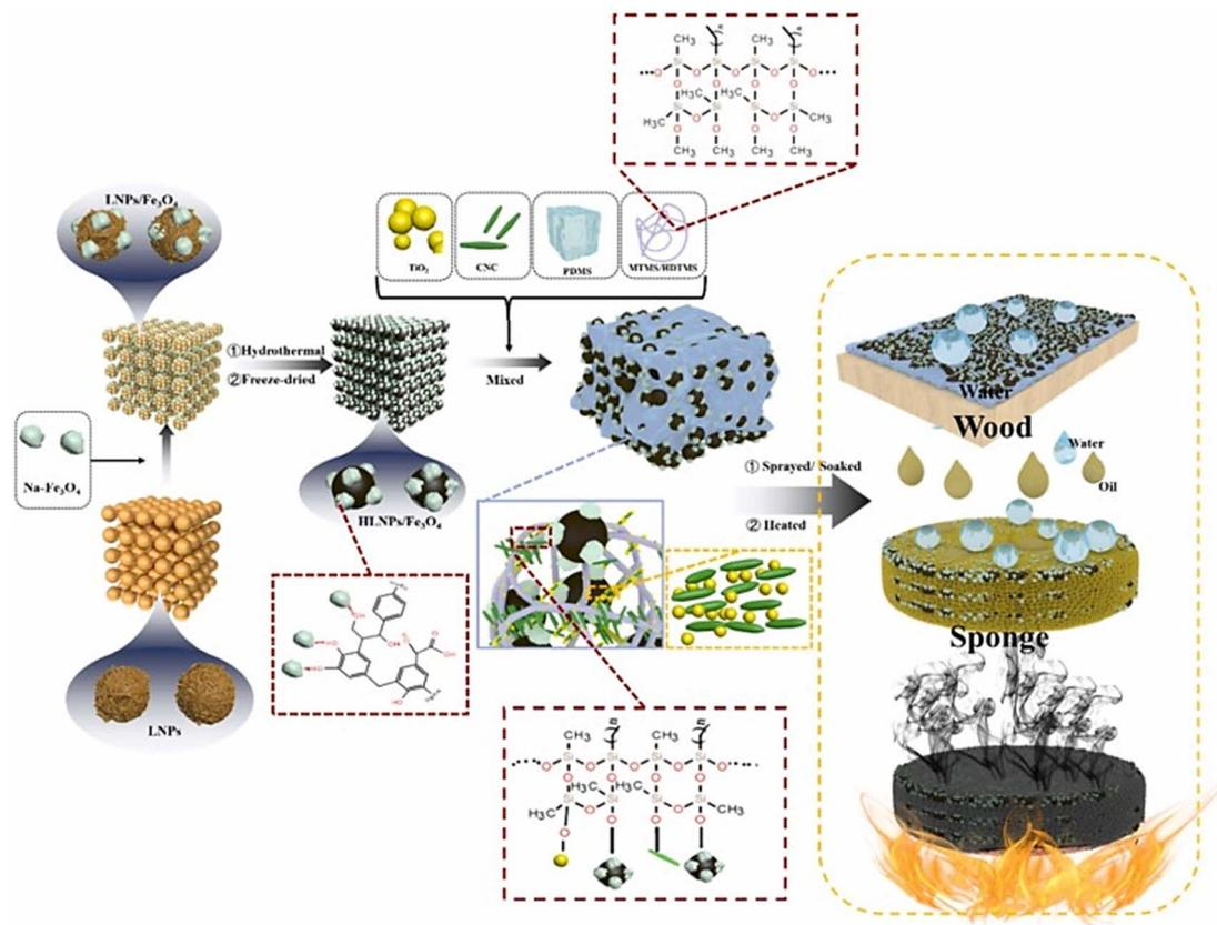
Fig. 14 Diagram illustrating the superhydrophobic coating's fabrication procedure using HLNPs and  $\text{Fe}_3\text{O}_4$ .<sup>102</sup> Reproduced from ref. 102 with permission from *Journal of Environmental Chemical Engineering*, copyright 2023.
