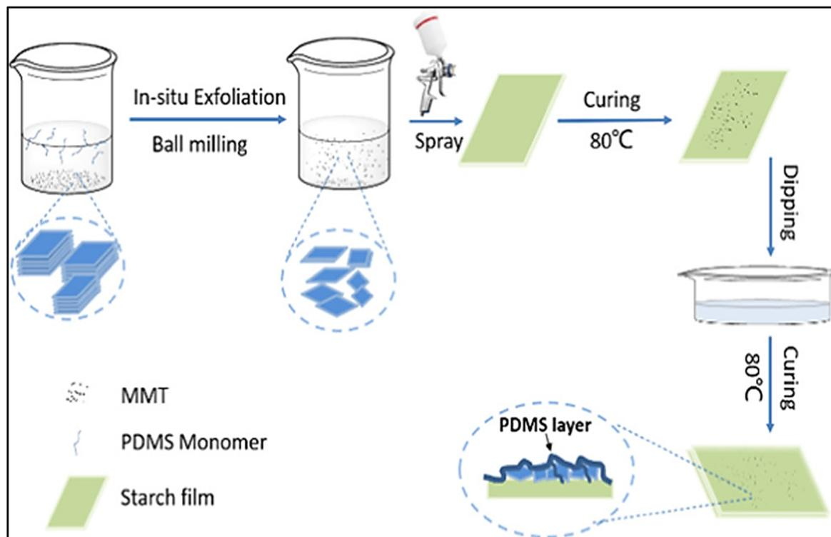
Fig. 25 Schematic representation of process used for preparing eco-friendly self-cleaning starch-based films.<sup>146</sup> Reproduced from ref. 146 with permission from *ACS Sustainable Chemistry & Engineering*, copyright 2020.
