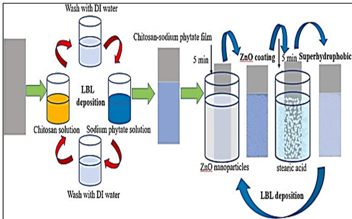
Fig. 24 Schematic preparation process using chitosan by layer-by-layer assembly.<sup>140</sup> Reproduced from ref. 140 with permission from *International Journal of Biological Macromolecules*, copyright 2023.
