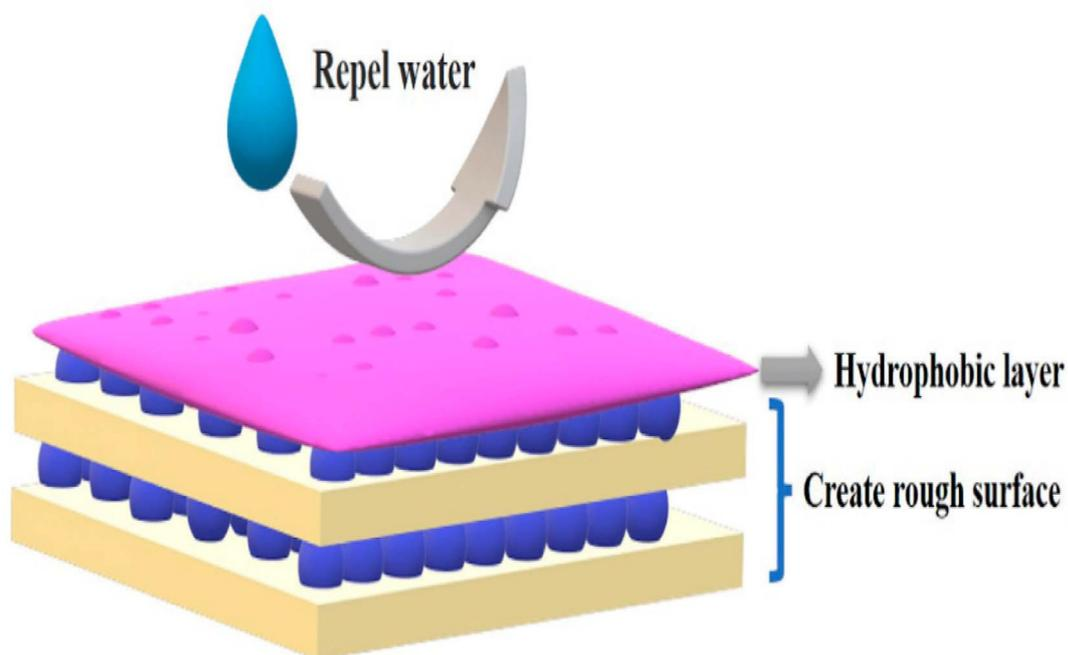
Fig. 10 Self-assembly technique and layer by layer deposition technique.<sup>72</sup> Reproduced from ref. 72 with permission from *Molecules*, copyright 2022.
