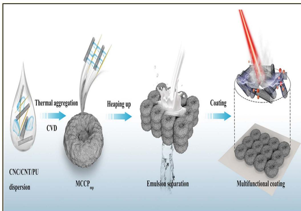
Fig. 16 A schematic illustration of the multipurpose, durable, superhydrophobic coating's preparation procedure for swift and intelligent water removal.<sup>111</sup> Reproduced from ref. 111 with permission from *Carbohydrate Polymers*, copyright 2020.
