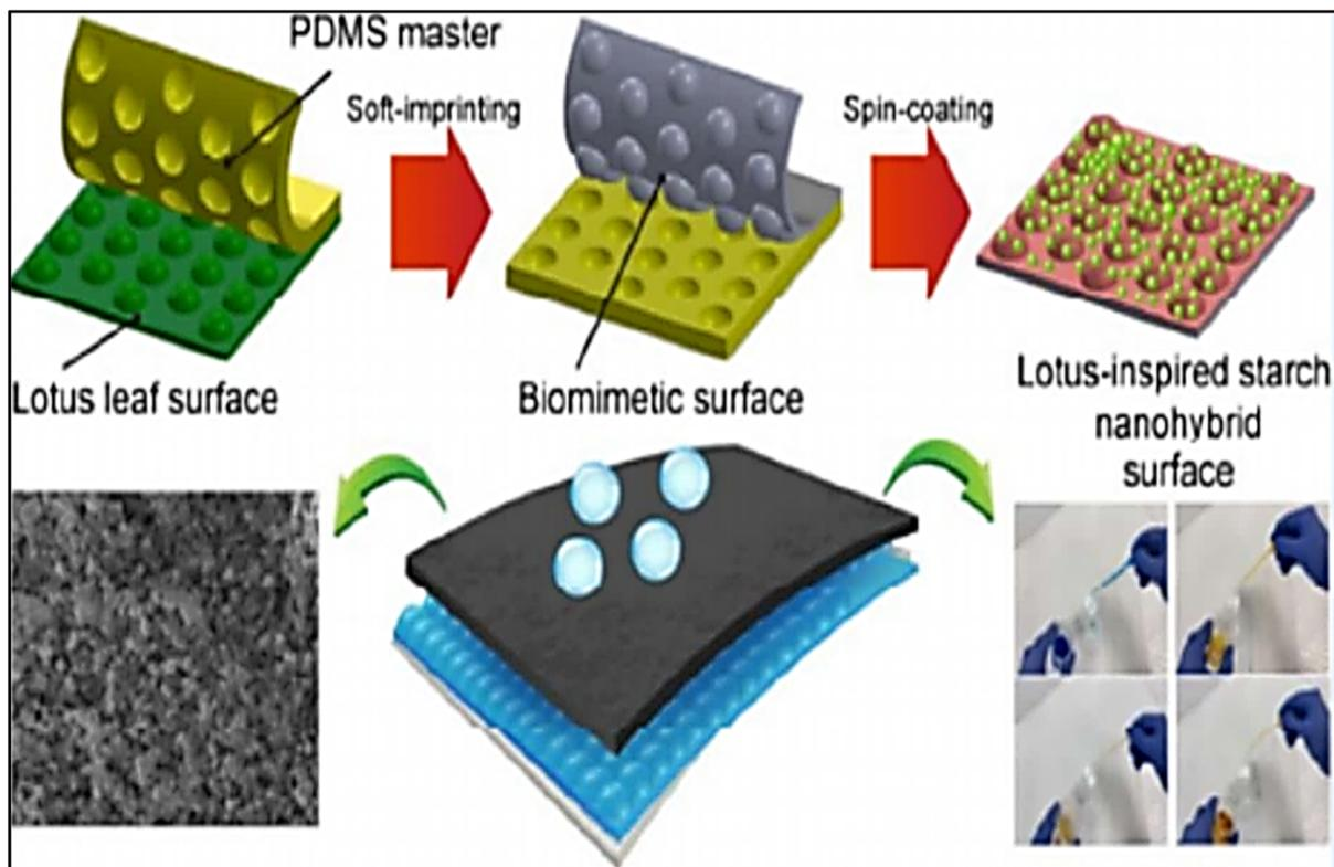
Fig. 27 Illustration of fabrication procedure of superhydrophobic coatings using starch–polyhydroxyurethane–cellulose nanocrystals (SPC).<sup>149</sup> Reproduced from ref. 149 with permission from ACS Applied Materials & Interfaces, copyright 2021.
