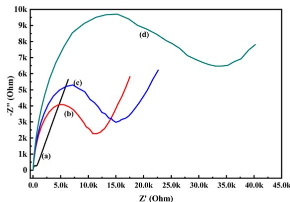
Fig. 15 EIS responses of (a) GCE, (b) PoPD/Ag hybrid-modified GCE towards and PoPD/Ag hybrid-modified GCE towards (c)  $10 \mu\text{L}$ , (d)  $50 \mu\text{L}$  blood sample in  $25 \text{ mL}$  aqueous KCl ( $1 \text{ M}$ ) electrolytes containing the  $10^{-3} \text{ M}$   $[\text{Fe}(\text{CN})_6]^{3-/4-}$  redox couple.
