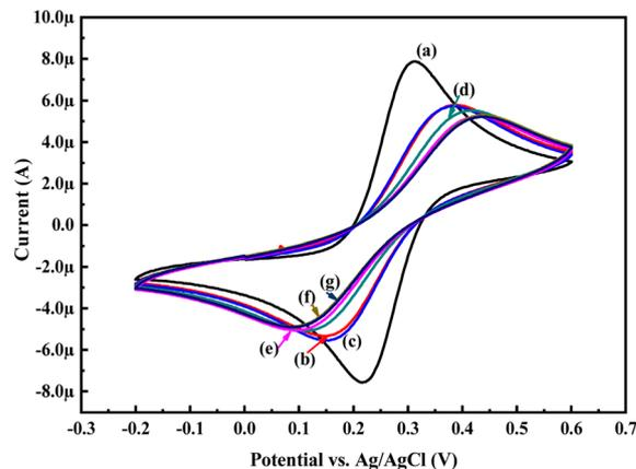
Fig. 8 CV responses of (a) GCE, (b) PoPD/Ag hybrid-modified GCE and PoPD/Ag hybrid-modified GCE towards (a) 10, (b) 20, (c) 30, (d) 40, and (e) 50  $\mu\text{L}$  of 72 mg per dL aqueous glucose at a scan rates of 50  $\text{mV s}^{-1}$  in 25 mL aqueous KCl (1 M) electrolytes containing the  $10^{-3}$  M  $[\text{Fe}(\text{CN})_6]^{3-/4-}$  redox couple.
