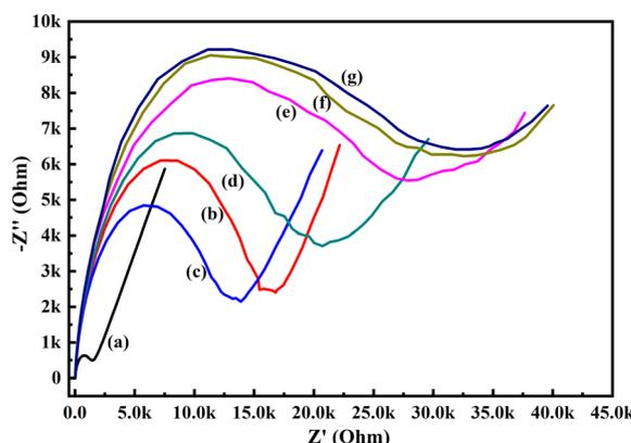
Fig. 9 EIS responses of (a) GCE, (b) PoPD/Ag hybrid-modified GCE and PoPD/Ag hybrid-modified GCE towards (c) 10, (d) 20, (e) 30, (f) 40, and (g) 50  $\mu\text{L}$  of 72 mg per dL aqueous glucose in 25 mL aqueous KCl (1 M) electrolytes containing the  $10^{-3}$  M  $[\text{Fe}(\text{CN})_6]^{3-/4-}$  redox couple.
