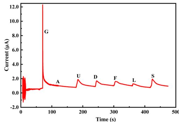
Fig. 14 Chronoamperometric response of the PoPD/Ag hybrid-modified GCE towards  $10 \mu\text{L}$  of  $0.1 \text{ mM}$  glucose (G), ascorbic acid (A), uric acid (U), dopamine (D), fructose (F), lactose (L) and sucrose (S) in  $25 \text{ mL}$  aqueous KCl ( $1 \text{ M}$ ) electrolytes containing the  $10^{-3} \text{ M}$   $[\text{Fe}(\text{CN})_6]^{3-/4-}$  redox couple.
