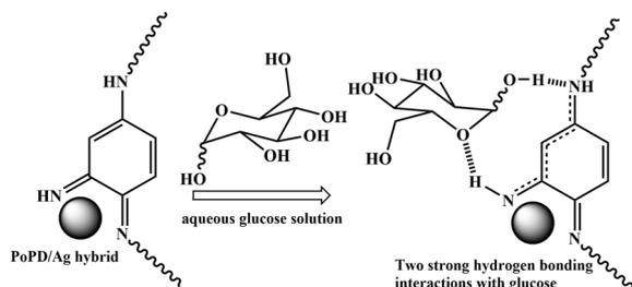
Fig. 10 Glucose sensing mechanism on PoPD/Ag-modified GCE electrode.
