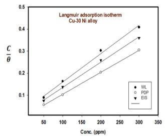
Fig. 6 Langmuir isotherm plot for the corrosion of Cu–Ni alloys in 3.5% NaCl solution in the absence and presence of different doses of LSE at 25 °C.
