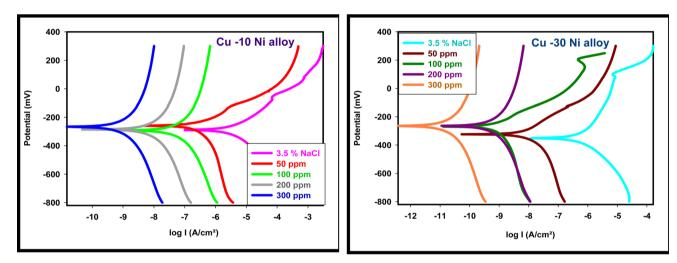
Fig. 3 PDP curves for used alloys in 3.5% NaCl with and without altered doses of LSE.
