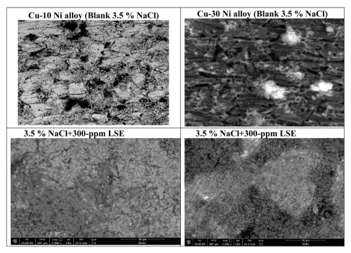
Surface morphology for Cu-Ni alloys exposed to 3.5% NaCl solution with inhibitor.
