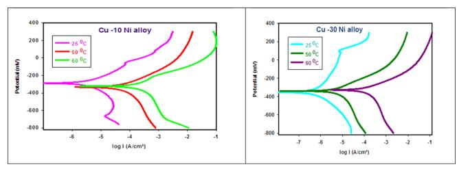
Fig. 7 PDP curves for Cu-Ni alloys in 3.5% NaCl solution at different temperatures.
