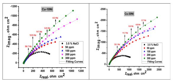
Nyquist plot for used alloys in 3.5% NaCl solution in the absence and presence of different doses of LSE at 25 °C
