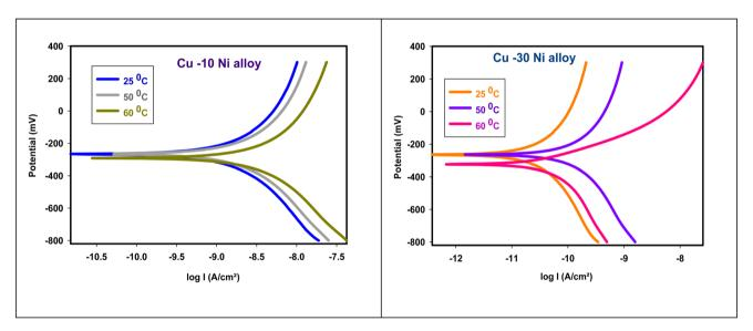
Fig. 8 PDP plots for used alloys in 3.5% NaCl solution in attendance of 300 ppm LSE at altered temperatures.
