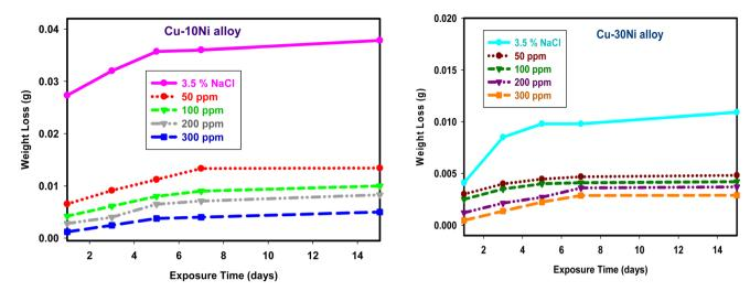
Fig. 2 WL-time curves for used alloys dipped in 3.5% NaCl with and without different doses of LSE.
