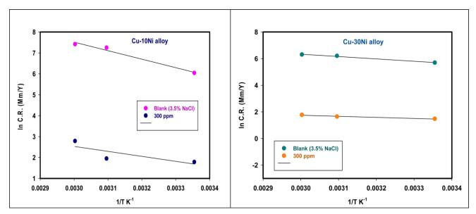
Fig. 9 A plot of Ln CR versus 1/T for Cu-Ni alloys in 3.5% NaCl containing 300 ppm LSE altered temperatures.
