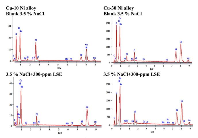
Fig. 11 EDX spectra for the used alloys exposed to 3.5% NaCl with LSE.
