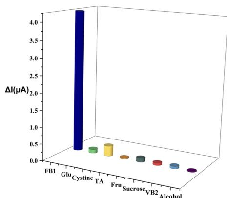
Fig. 5 Detection of multiple compounds by the AuNPs-SPE. The concentration of FB1 was 1 μg mL<sup>-1</sup>.
