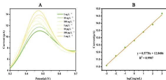
Fig. 4 (A) DPVs of FB1 with different concentrations of the AuNPs-SPE. FB1 concentrations ranged from 1 ng L<sup>-1</sup> to 1 mg L<sup>-1</sup>. The concentration of the next one is 10 times that of the previous one. (B) Linear relationship between current intensity and the concentration of FB1.
