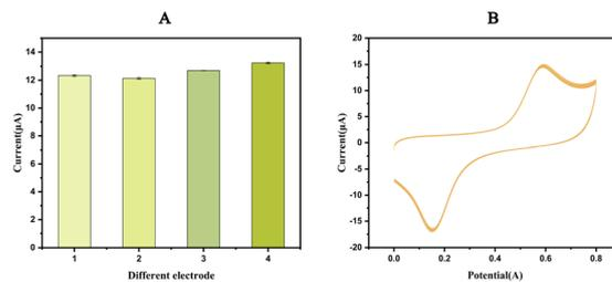
Fig. 6 (A) Bar plots of the cathodic peak current of four different AuNPs-SPEs. (B) Thirty CV results of the AuNPs-SPE in PBS.
