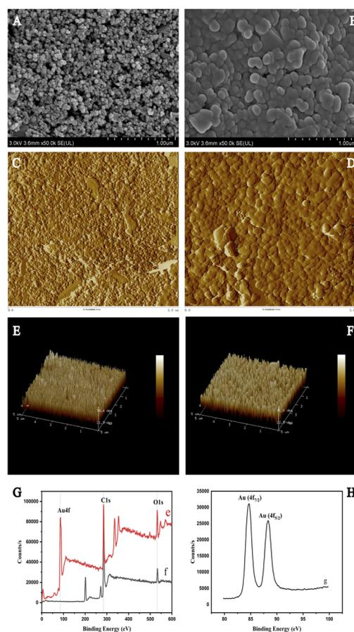
Fig. 1 SEM images of bare SPE ( $\times 50 \text{ k}$ ; A) and of AuNPs-SPE ( $\times 50 \text{ k}$ ; B). The AFM 2D and 3D surface morphology of bare SPE (C and E) and of AuNPs-SPE (D and F). XPS images of the AuNPs-SPE sensor (G), Au 4f (H); AuNPs-SPE (E), bare SPE (F), AuNPs-SPE (G).
