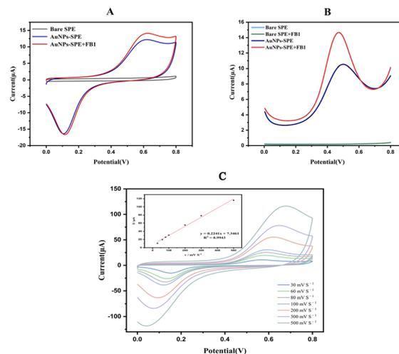
Fig. 3 (A) CVs of FB1 (0.1 mg L<sup>-1</sup>) in 0.1 M PBS (pH = 7.4) of the bare SPE and AuNPs-SPE. (B) DPVs of FB1 (0.1 mg L<sup>-1</sup>) in 0.1 M PBS (pH = 7.4) of the bare SPE and AuNPs-SPE. The blue line coincides with the green line. (C) The CV of 10 mL PBS in 0.1 M FB1 on the AuNPs-SPE.
