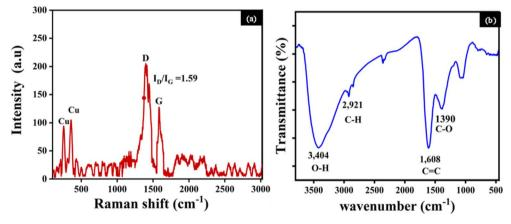
Fig. 3 (a) Raman and (b) FTIR spectra of the fabricated Cu/C NPs.
