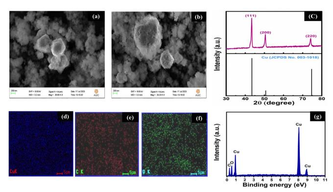
Fig. 1 (a and b) FESEM images, (c) XRD pattern (with a slandered index of Cu, C, O) of the synthesized material, (d-f) EDX elemental mapping, and (g) the corresponding EDX spectrum.
