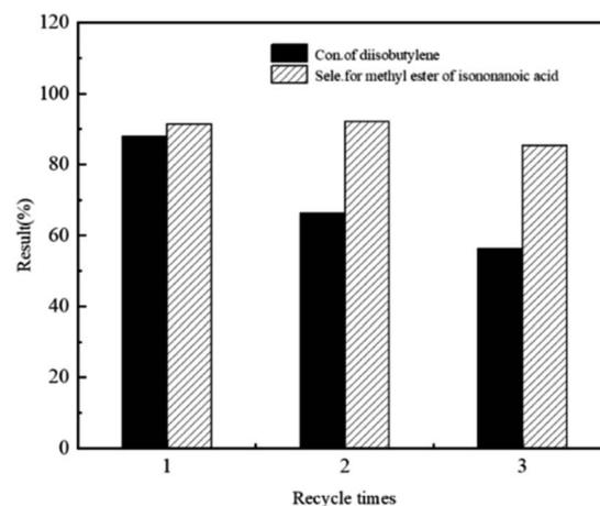
Fig. 7 Reusability of HVIMI-VPy-DVB (1 : 1)@ $\text{Co}_2(\text{CO})_8$  in the methoxycarbonylation reaction of DIB and CO.  $\text{Co}_2(\text{CO})_8$ : 4 wt%, N : Co = 2 : 1 (mol ratio), 150 °C, 8.0 MPa, 12 h.
