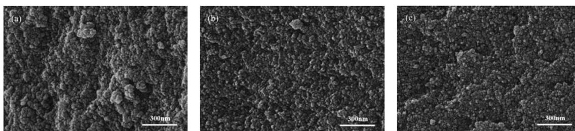
Fig. 5 SEM images of poly(ionic liquids). (a) EVIMI-VPy-DVB (1 : 1), (b) BVIMI-VPy-DVB (1 : 1), and (c) HVIMI-VPy-DVB (1 : 1).
