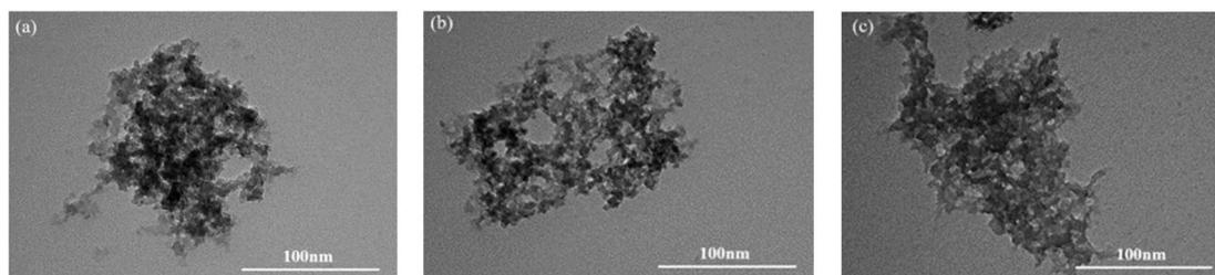
Fig. 6 TEM images of poly(ionic liquids). (a) EVIMI-VPy-DVB (1 : 1), (b) BVIMI-VPy-DVB (1 : 1), and (c) HVIMI-VPy-DVB (1 : 1).
