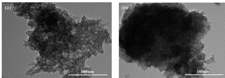
Fig. 8 The TEM images of HVIMI-VPy-DVB (1 : 1) @Co<sub>2</sub>(CO)<sub>8</sub> catalyst before and after use. (a) Before use and (b) after use.
