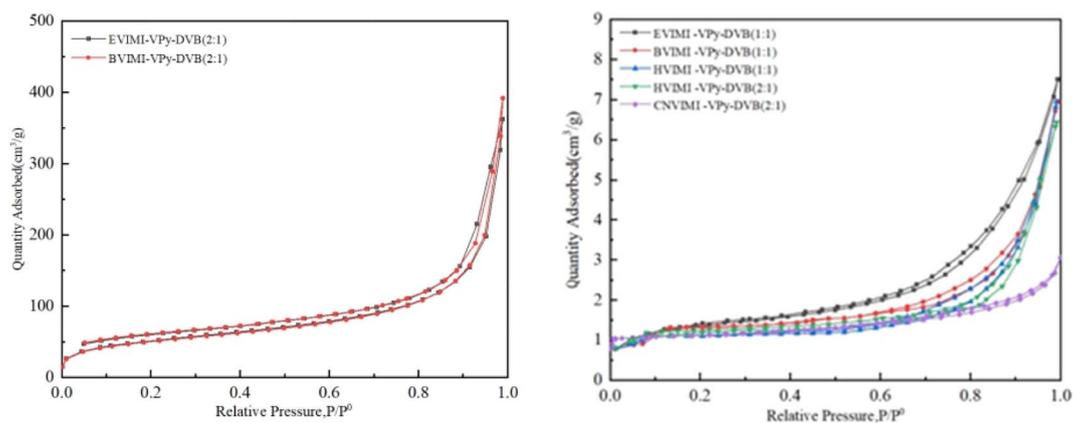
Fig. 4  $N_2$  adsorption–desorption isotherms of poly(ionic liquids).
