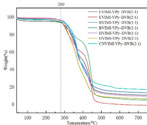
Fig. 3 TG analysis curves of poly(ionic liquids).
