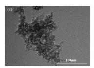
Fig. 6 TEM images of poly(ionic liquids). (a) EVIMI-VPy-DVB (1:1), (b) BVIMI-VPy-DVB (1:1), and (c) HVIMI-VPy-DVB (1:1).
