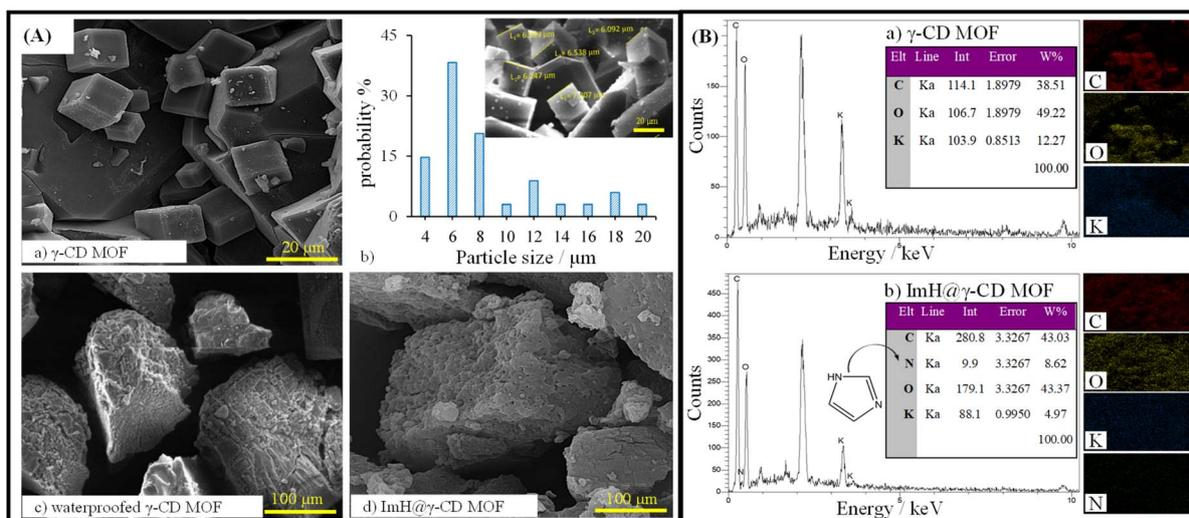
Fig. 1 (A) Scanning electron microscope (SEM) images of (a)  $\gamma$ -CD MOF, (b) size distribution of  $\gamma$ -CD MOF, (c) waterproofed  $\gamma$ -CD MOF, and (d) ImH@ $\gamma$ -CD MOF. (B) Energy dispersive X-ray spectroscopy (EDS) and elemental scattering map of (a)  $\gamma$ -CD MOF and (b) ImH@ $\gamma$ -CD MOF.
