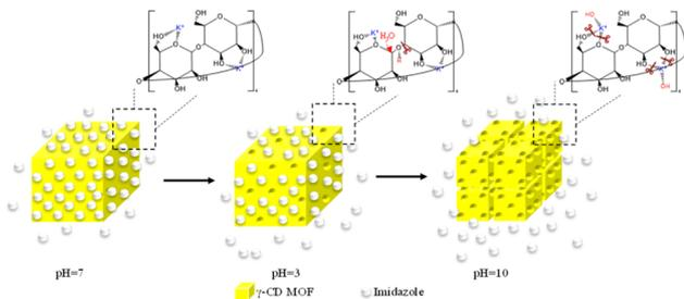
Scheme 1 Schematic representation of the pH-responsive release of imidazole at different pH.
