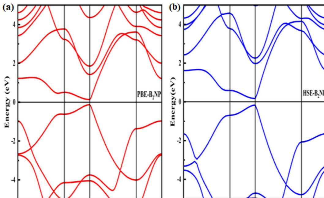
Fig. 3 Electronic band structures of (a) PBE-B<sub>2</sub>NP and (b) HSE-B<sub>2</sub>NP monolayer systems.
