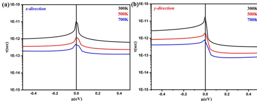
Fig. 6 Relaxation time as a function of the chemical potential of monolayer systems at 300 K, 500 K and 700 K in (a) the X-direction and (b) Y-direction.
