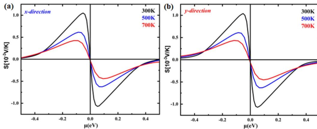
Fig. 5 The calculated Seebeck coefficient as a function of chemical potential at 300 K, 500 K and 700 K temperatures of (a) B<sub>2</sub>NP monolayer in the X-direction and (b) B<sub>2</sub>NP monolayer in the Y-direction.
