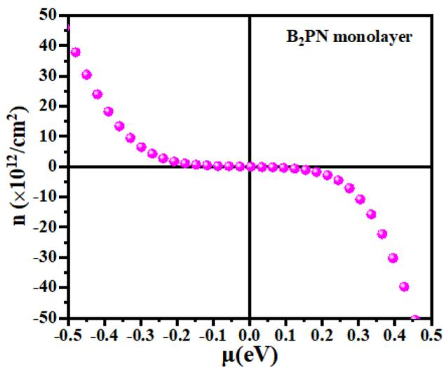
Fig. 4 The calculated carrier concentration as a function of the chemical potential of the B<sub>2</sub>NP monolayer system.
