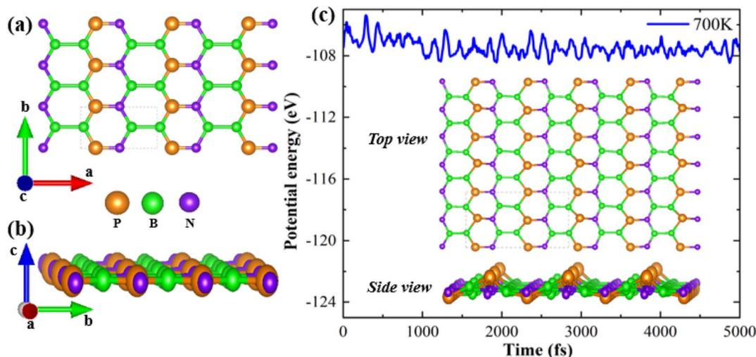
Fig. 1 (a) Top view and (b) side view of the optimized crystal structure of B<sub>2</sub>PN, and (c) evolution of potential energy with a simulation time for B<sub>2</sub>PN. The inset shows the top and side views of the structure with molecular dynamics at 700 K.
