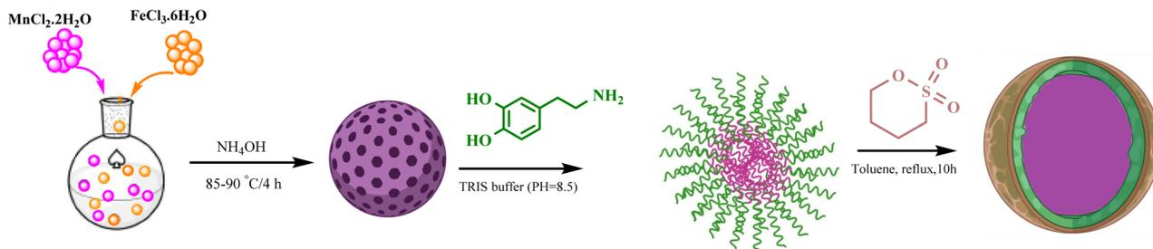
Scheme 1 Synthesis of  $MFe_2O_4@PDA@BuSO_3H$  MNPs as a new heterogeneous catalyst.
