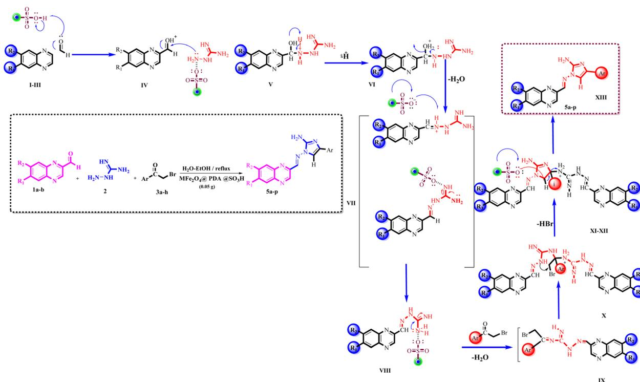
Scheme 3 The proposed mechanism for preparing 2-benzopyrazine-aminoimidazole hybrid derivatives (5a-p) using  $\text{MFe}_2\text{O}_4@\text{PDA}@\text{BuSO}_3\text{H}$  MNPs (0.05 g) as catalyst in  $\text{H}_2\text{O}-\text{EtOH}$  (1 : 1), reflux.
