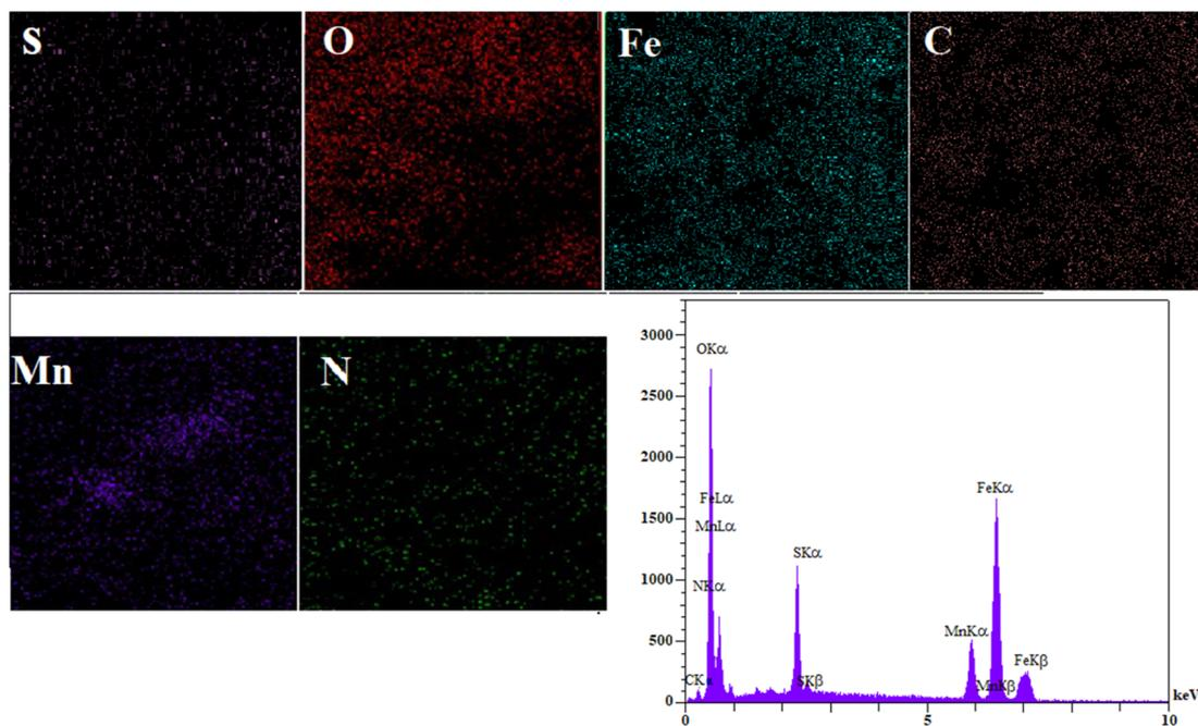
Fig. 3 EDS spectra of  $MFe_2O_4@PDA@BuSO_3H$  MNPs.
