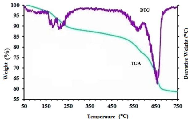
Fig. 4 TGA spectra of  $\text{MFe}_2\text{O}_4@PDA@BuSO_3H$  MNPs.
