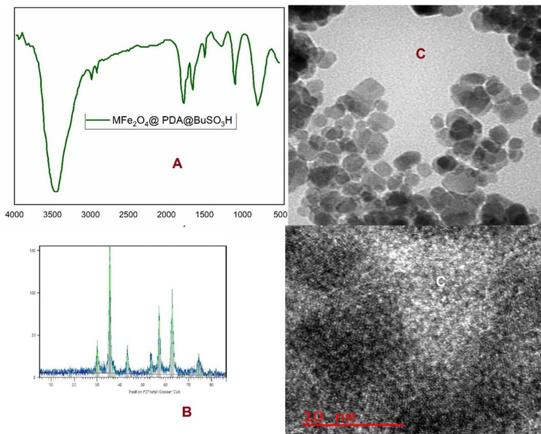
Fig. 8 A) FT-IR, (B) XRD, and (C) TEM analysis of the recovered MFe<sub>2</sub>O<sub>4</sub>@PDA@BuSO<sub>3</sub>H MNPs (0.05 g) as a catalyst in H<sub>2</sub>O–EtOH (1 : 1), reflux.
