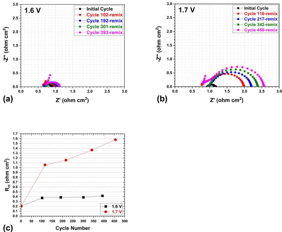
Fig. 5 Typical Nyquist plots at the top of charge (TOC) after remixing (at every  $\sim 100$  cycles), with an upper cut-off voltage of (a) 1.6 V and (b) 1.7 V; and (c) the charge transfer resistances ( $R_{ct}$ ) of the 1.6 V and 1.7 V cells by EIS curves (5a and 5b) analysis using the Zview program (Scribner).
