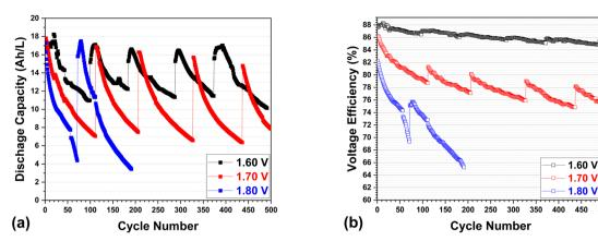
Fig. 2 (a) Specific discharge capacity (A h  $L^{-1}$ ) and (b) voltage efficiency (%) of a VRFB as a function of cycle number at different upper limit voltages of 1.6, 1.7, and 1.8 V.
