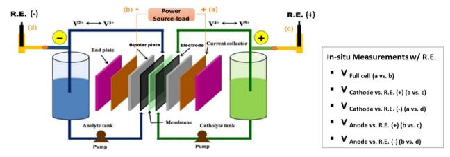
Fig. 1 In situ measurement setup of a vanadium redox flow battery with the reference electrodes (R.E.) in the inlet tubing of the catholyte and anolyte respectively.
