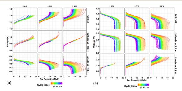
Fig. 3 Voltage profiles of full cell and its individual electrodes (cathode or anode vs. RE+) vs. specific capacity (A h  $L^{-1}$ ) for initial 70 cycles: during (a) charge and (b) discharge process, at different upper limit voltages of 1.6 V, 1.7 V, and 1.8 V.
