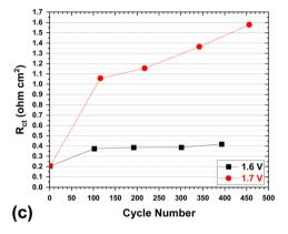
Fig. 5 Typical Nyquist plots at the top of charge (TOC) after remixing (at every ~100 cycles), with an upper cut-off voltage of (a) 1.6 V and (b) 1.7 V; and (c) the charge transfer resistances ( $R_{ct}$ ) of the 1.6 V and 1.7 V cells by EIS curves (5a and 5b) analysis using the Zview program (Scribner).
