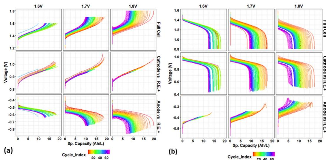
Fig. 3 Voltage profiles of full cell and its individual electrodes (cathode or anode vs. RE+) vs. specific capacity ( $\text{A h L}^{-1}$ ) for initial 70 cycles: during (a) charge and (b) discharge process, at different upper limit voltages of 1.6 V, 1.7 V, and 1.8 V.
