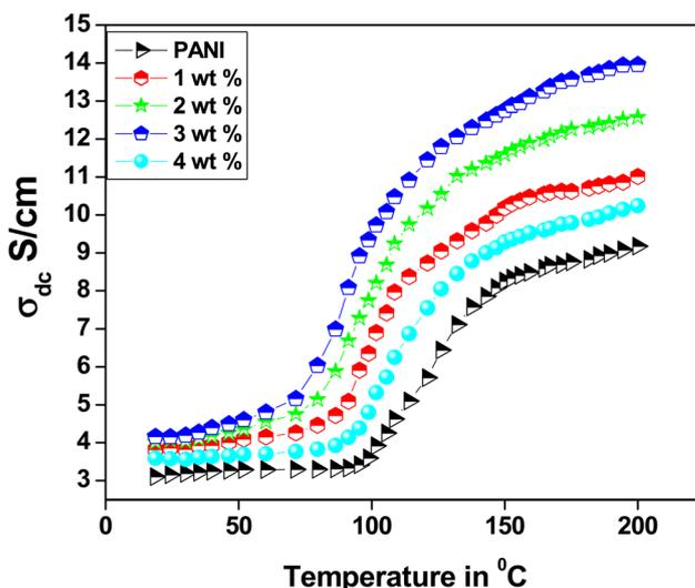
Fig. 7 DC conductivity of PANI and its nanocomposites.
