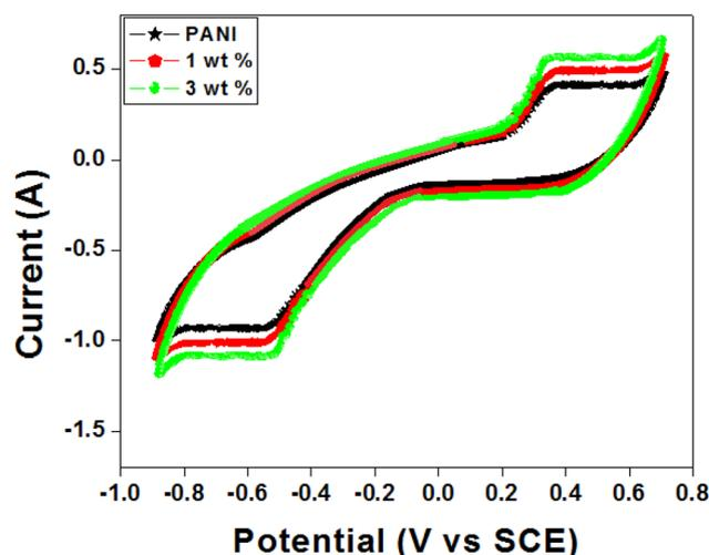
Fig. 8 Cyclic voltammetry (CV) curves of PANI and PANI-Zn/V<sub>2</sub>O<sub>5</sub> nanocomposites.
