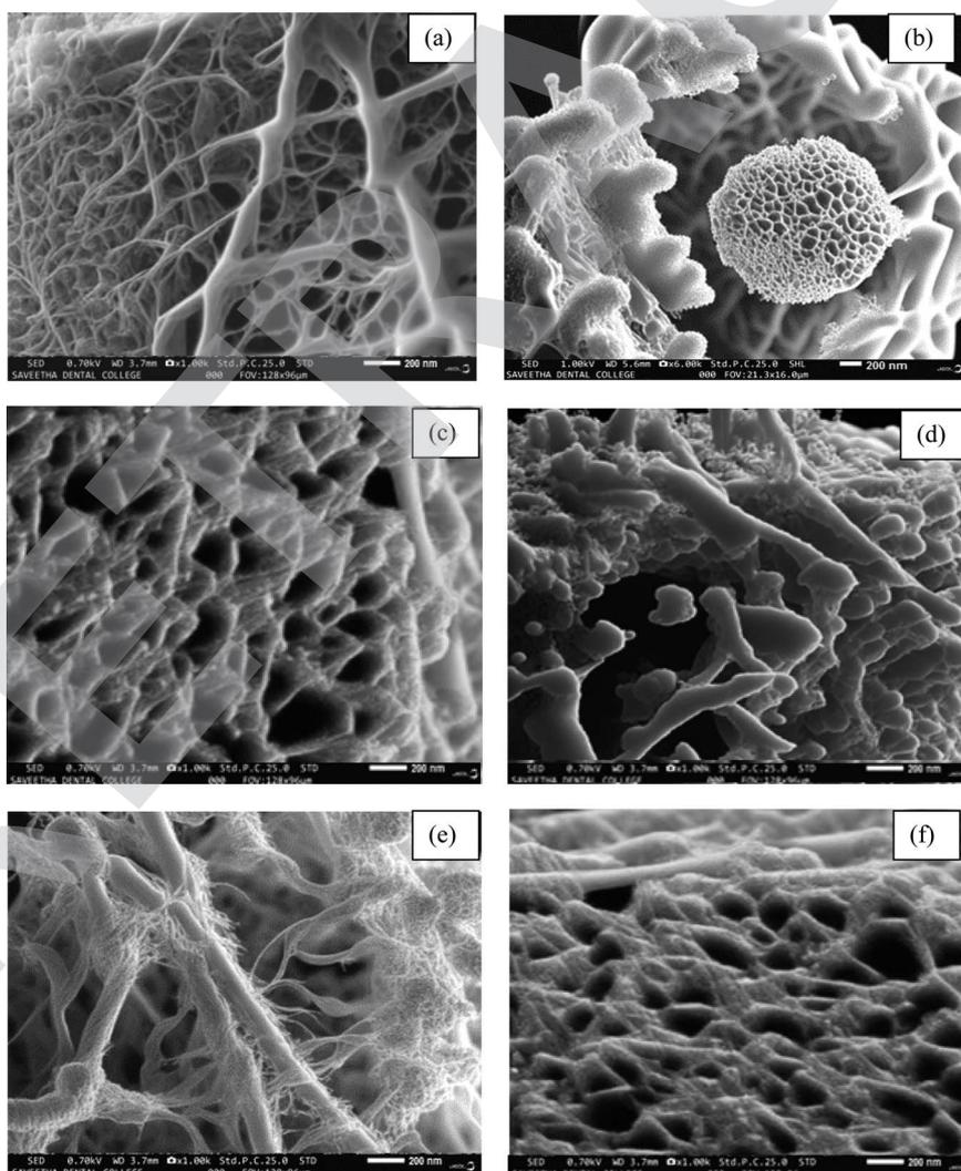
Fig. 4 SEM image of (a) PANI, (b) porous Zn/V<sub>2</sub>O<sub>5</sub> nanoparticles, and (c–f) 1 wt%, 2 wt%, 3 wt% and 4 wt% of PANI-Zn/V<sub>2</sub>O<sub>5</sub> nanocomposites.
