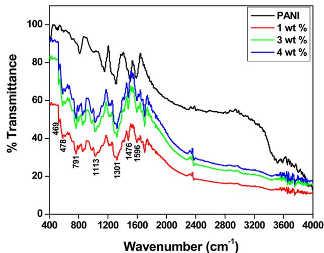
Fig. 2 FTIR spectra of PANI, Zn/V<sub>2</sub>O<sub>5</sub> nanoparticles and 3 wt% of PANI-ZVO nanocomposites.
