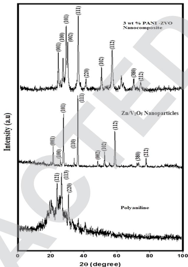
Fig. 3 XRD of PANI, Zn/V<sub>2</sub>O<sub>5</sub> nanoparticles and 3 wt% of PANI-ZVO nanocomposites.
