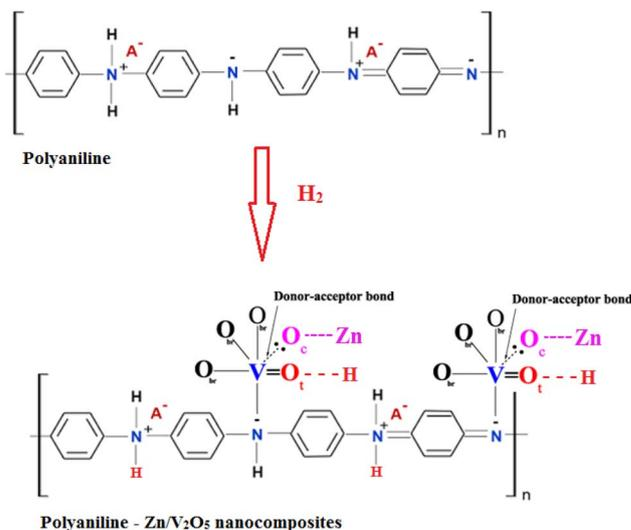
Fig. 10 Hydrogen absorption mechanism of the PANI-Zn/V<sub>2</sub>O<sub>5</sub> nanocomposites.
