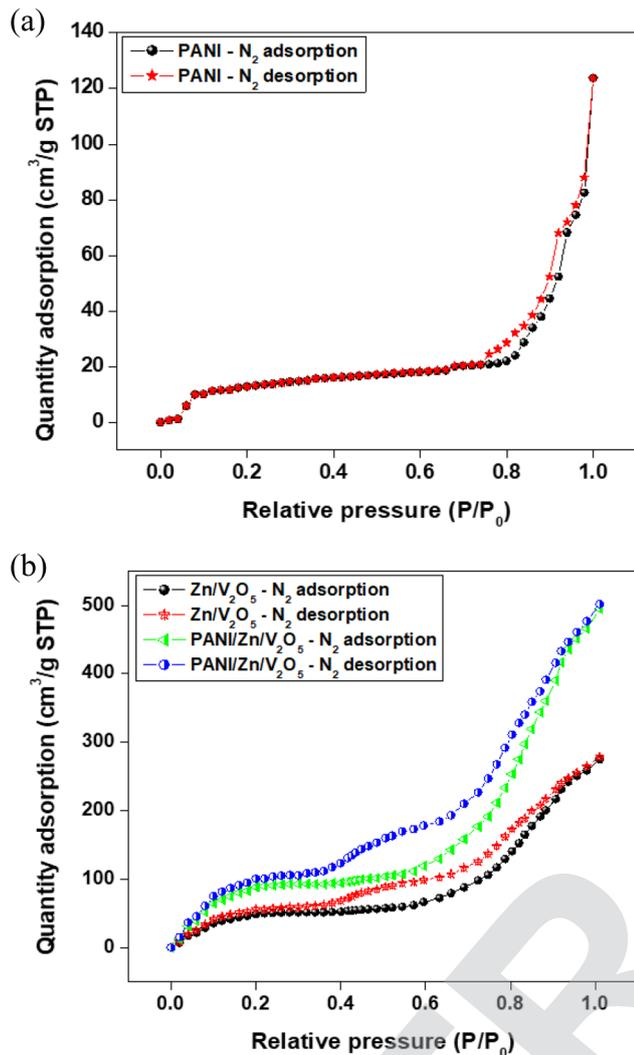
Fig. 5 Surface area analysis using Brunauer–Emmett–Teller (BET) analysis: N<sub>2</sub> adsorption–desorption isotherm of (a) PANI, Zn/V<sub>2</sub>O<sub>5</sub> and (b) 3 wt% of the PANI-Zn/V<sub>2</sub>O<sub>5</sub> nanocomposite.
