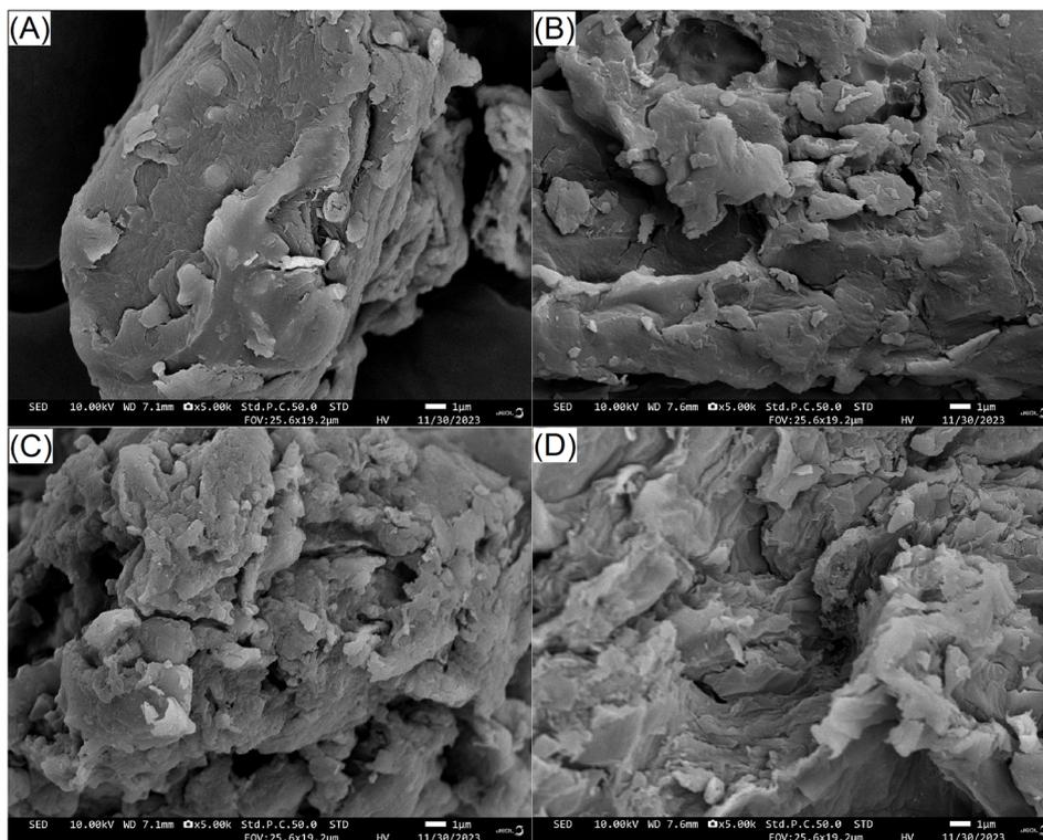
**Fig. 1** Scanning electron microscopy images of JKF (A), JKF-E (B), JKF-EA (C), and JKF-EC (D) with a magnification of 5000 $\times$  at 1  $\mu$ m. JKF, jujube kernel fibre; JKF-E, JKF modified via mixed enzymatic hydrolysis; JKF-EA, JKF treated via mixed enzymatic hydrolysis and acetylation; and JKF-EC, JKF treated via mixed enzymatic hydrolysis combined with carboxymethylation.
