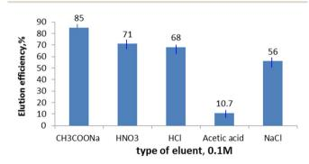
Effect of the eluent type on uranium elution efficiency.
