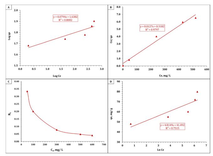
Fig. 6 (A) Freundlich isotherm plot, (B) Langmuir isotherm plot, (C) separation factor  $R_{\rm L}$ , and (D) Temkin isotherm plot for the adsorption of uranium on EPMPS.
