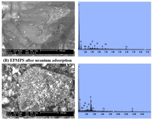
Fig. 3 SEM images and EDX spectra of EPMPS (A) before and (B) after uranium adsorption.
