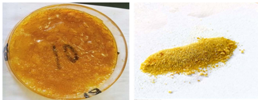
Fig. 1 Photographs of the cured created polymeric material of epoxy-modified phosphorus pentasulfide (EPMPs) formulation, and the material after grinding.
