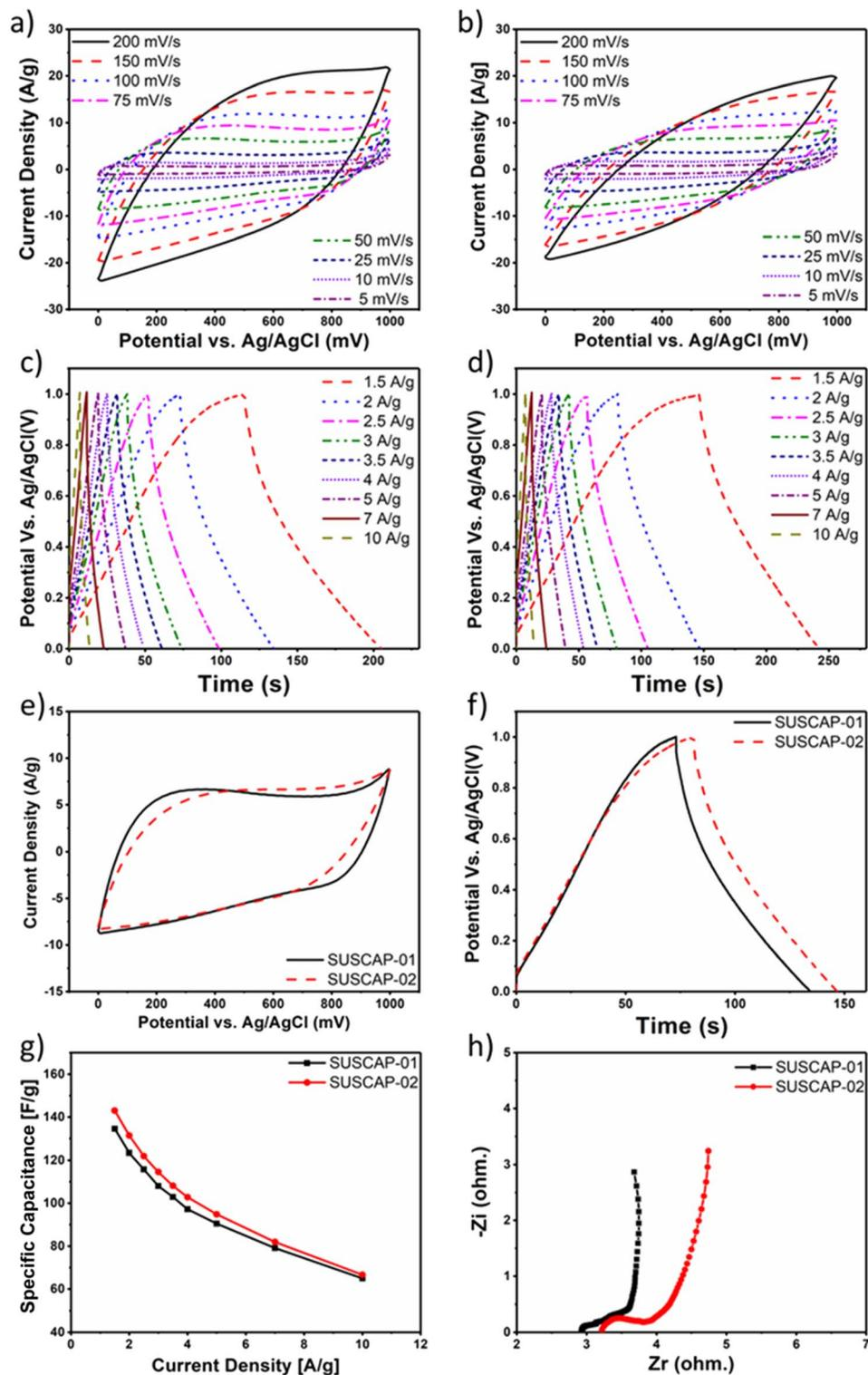
Fig. 5 CV curves at different scan rates for (a) SUSCAP-01 and (b) SUSCAP-02; GCD curves at different current densities (c) SUSCAP-01 and (d) SUSCAP-02; (e) CV curves at a scan rate of  $50 \text{ mV s}^{-1}$ , (f) GCD curves at a CD  $2 \text{ A g}^{-1}$ ; (g) specific capacitance of SUSCAP-01 and SUSCAP-02; (h) EIS of SUSCAP-01 and SUSCAP-02; all performed in aqueous neutral electrolyte ( $\text{Na}_2\text{SO}_4$ ).
