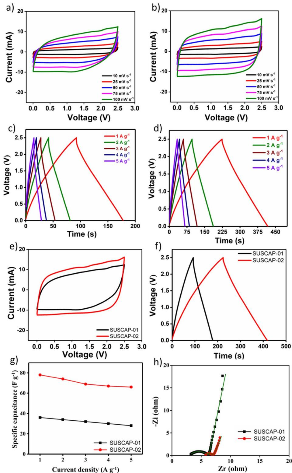
Fig. 6 CV curves at different scan rates for (a) SUSCAP-01 and (b) SUSCAP-02; GCD curves at different current densities (c) SUSCAP-01 and (d) SUSCAP-02; (e) CV curves at a scan speed of  $50 \text{ mV s}^{-1}$ , (f) GCD curves at a CD  $2 \text{ A g}^{-1}$ ; (g) specific capacitance of SUSCAP-01 and SUSCAP-02; (h) EIS of SUSCAP-01 and SUSCAP-02; all performed in organic electrolyte.
