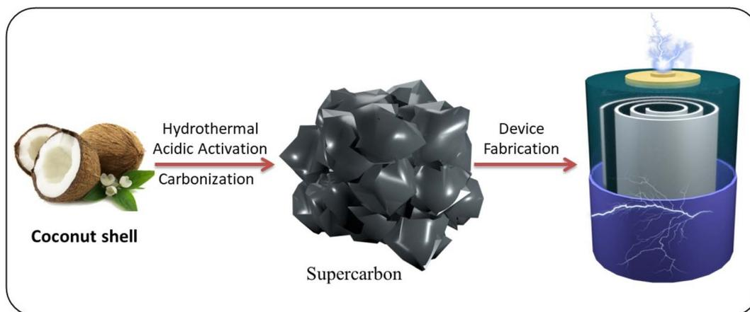
Fig. 1 Schematic illustration of the preparation of activated carbon for supercapacitor.
