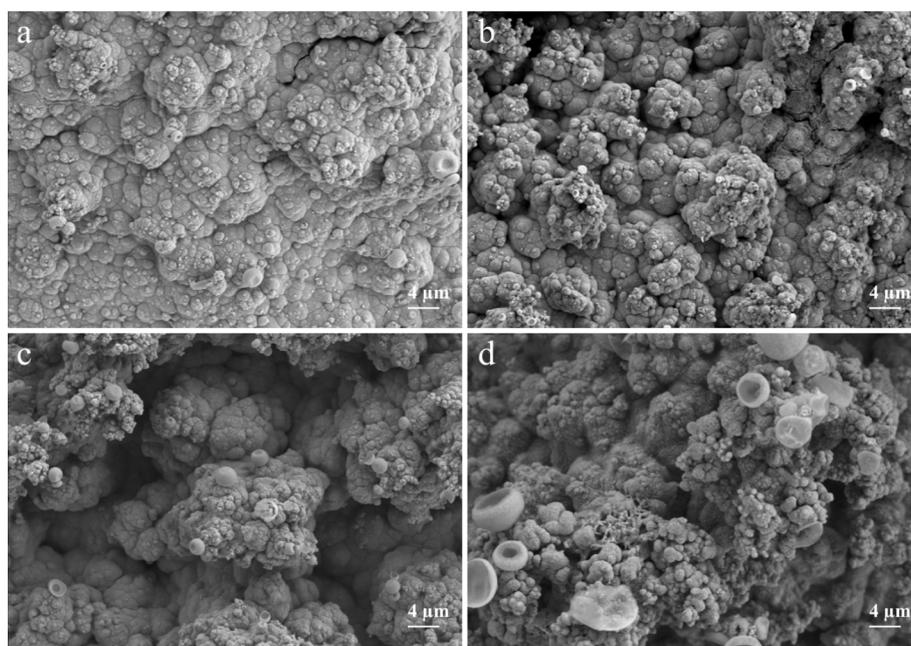
Fig. 4 (a) SEM image of  $\text{Ni}_3\text{S}_2/\text{Ni}$  mesh with a current density of  $20 \text{ mA cm}^{-2}$  for 1200 s; (b) SEM image of  $\text{Ni}_3\text{S}_2/\text{Ni}$  mesh with a current density of  $30 \text{ mA cm}^{-2}$  for 1200 s; (c) SEM image of  $\text{Ni}_3\text{S}_2/\text{Ni}$  mesh with a current density of  $40 \text{ mA cm}^{-2}$  for 1200 s; (d) SEM image of  $\text{Ni}_3\text{S}_2/\text{Ni}$  mesh with a current density of  $50 \text{ mA cm}^{-2}$  for 1200 s.
