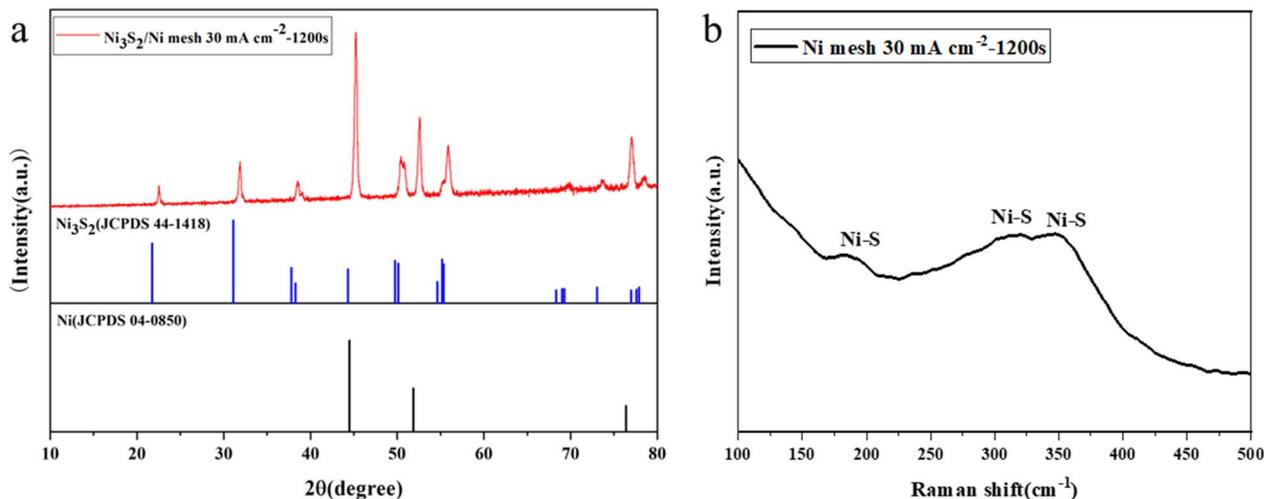
Fig. 1 (a) XRD patterns of  $\text{Ni}_3\text{S}_2/\text{Ni}$  mesh; (b) Raman spectra of  $\text{Ni}_3\text{S}_2/\text{Ni}$  mesh.
