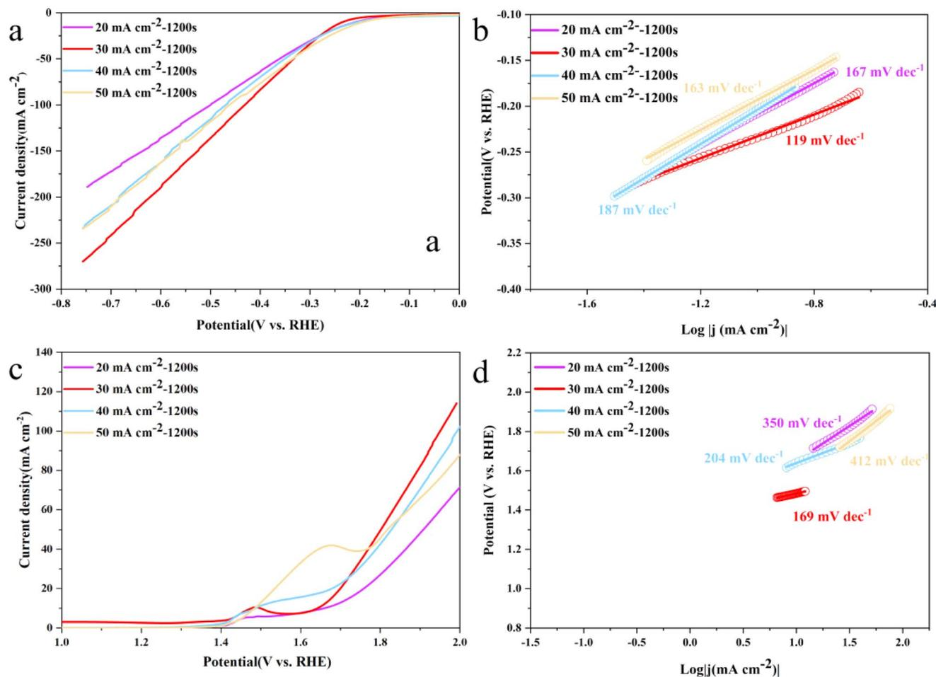
Fig. 5 HER polarisation curves (a) and OER polarisation curves (c) for  $\text{Ni}_3\text{S}_2/\text{Ni}$  mesh electrodes synthesized in 1.0 M KOH at deposition current densities of 20, 30, 40, and 50  $\text{mA cm}^{-2}$ ; Tafel plots for HER (b) and OER (d) for  $\text{Ni}_3\text{S}_2/\text{Ni}$  mesh electrodes synthesized in 1.0 M KOH at deposition current densities of 20, 30, 40, and 50  $\text{mA cm}^{-2}$ .
