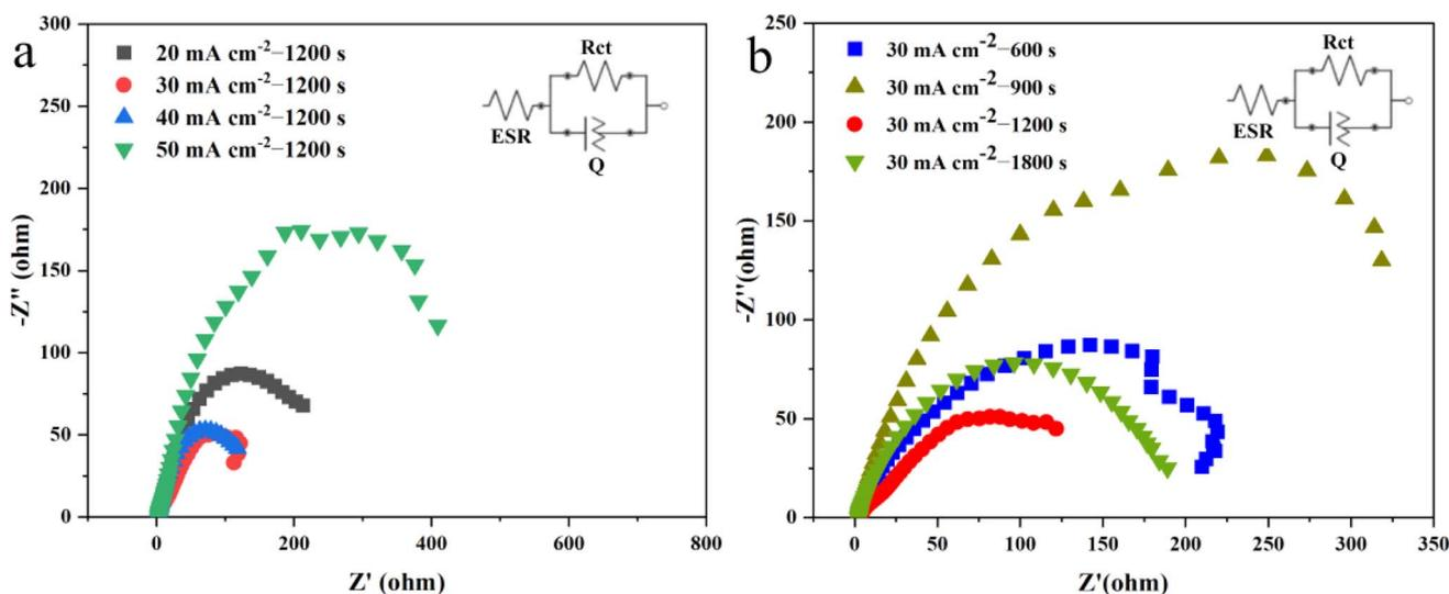
Fig. 8 (a) EIS spectra of Ni<sub>3</sub>S<sub>2</sub>/Ni mesh electrodes synthesized at deposition current densities of 20, 30, 40, and 50 mA cm<sup>-2</sup>; (b) EIS spectra of Ni<sub>3</sub>S<sub>2</sub>/Ni mesh electrodes deposited at 30 mA cm<sup>-2</sup> for 600, 900, 1200, and 1800 s, respectively.
