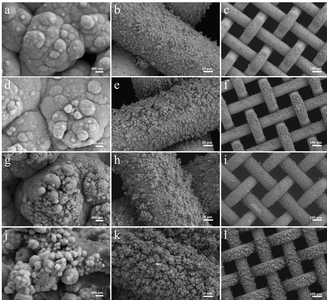
Fig. 6 (a–c) SEM image of  $\text{Ni}_3\text{S}_2/\text{Ni}$  mesh  $30 \text{ mA cm}^{-2}$ –600 s; (d–f) SEM image  $\text{Ni}_3\text{S}_2/\text{Ni}$  mesh  $30 \text{ mA cm}^{-2}$ –900 s; (g–i) SEM image of  $\text{Ni}_3\text{S}_2/\text{Ni}$  mesh  $30 \text{ mA cm}^{-2}$ –1200 s; (j–l) SEM image of  $\text{Ni}_3\text{S}_2/\text{Ni}$  mesh  $30 \text{ mA cm}^{-2}$ –1800 s.
