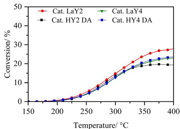
Fig. 8 Conversion of 3-methyl thiophene vs. temperature of reaction.
