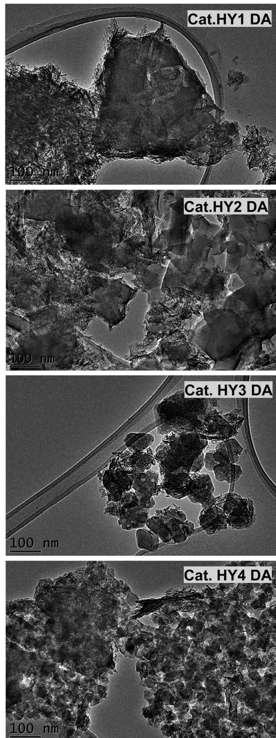
Fig. 2 TEM images of NiMo/(HY DA + Al<sub>2</sub>O<sub>3</sub>) catalysts.
