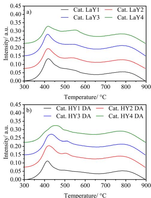
Fig. 7 TPR-H<sub>2</sub> profiles of the catalysts (a) LaY and (b) HY DA.
