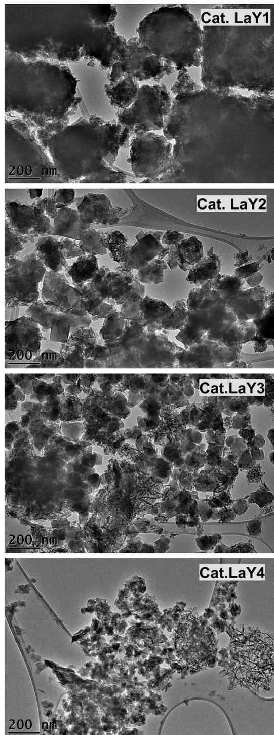
Fig. 1 TEM images of NiMo/(LaY + Al<sub>2</sub>O<sub>3</sub>) catalysts.
