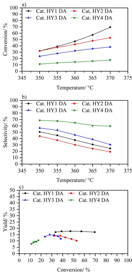
Fig. 10 (a) Conversion wt% vs. temperature, (b) selectivity to middle distillates wt% vs. temperature and (c) yield to distillates wt% vs. conversion to catalysts HY1 DA, HY2 DA, HY3 DA, and HY4 DA.
