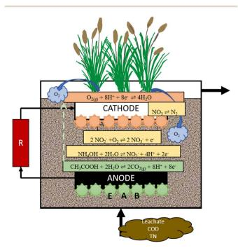
Fig. 2 Mechanism of leachate treatment in CW-MFCs.
