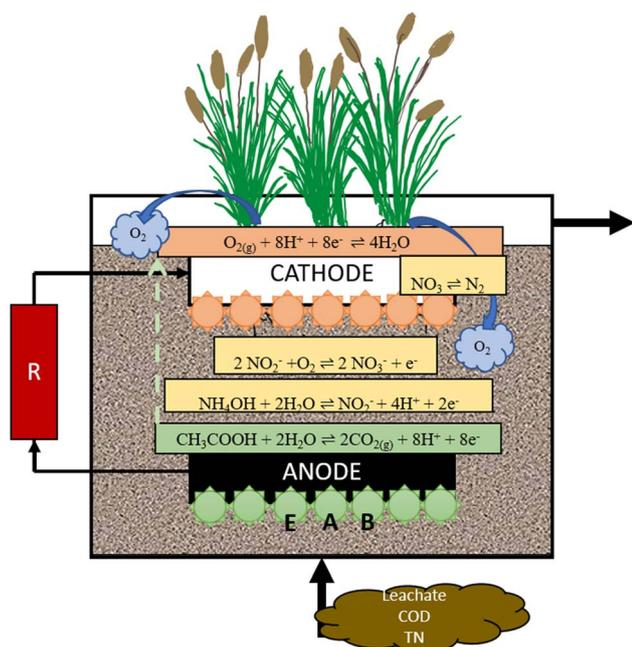
Fig. 2 Mechanism of leachate treatment in CW-MFCs.
