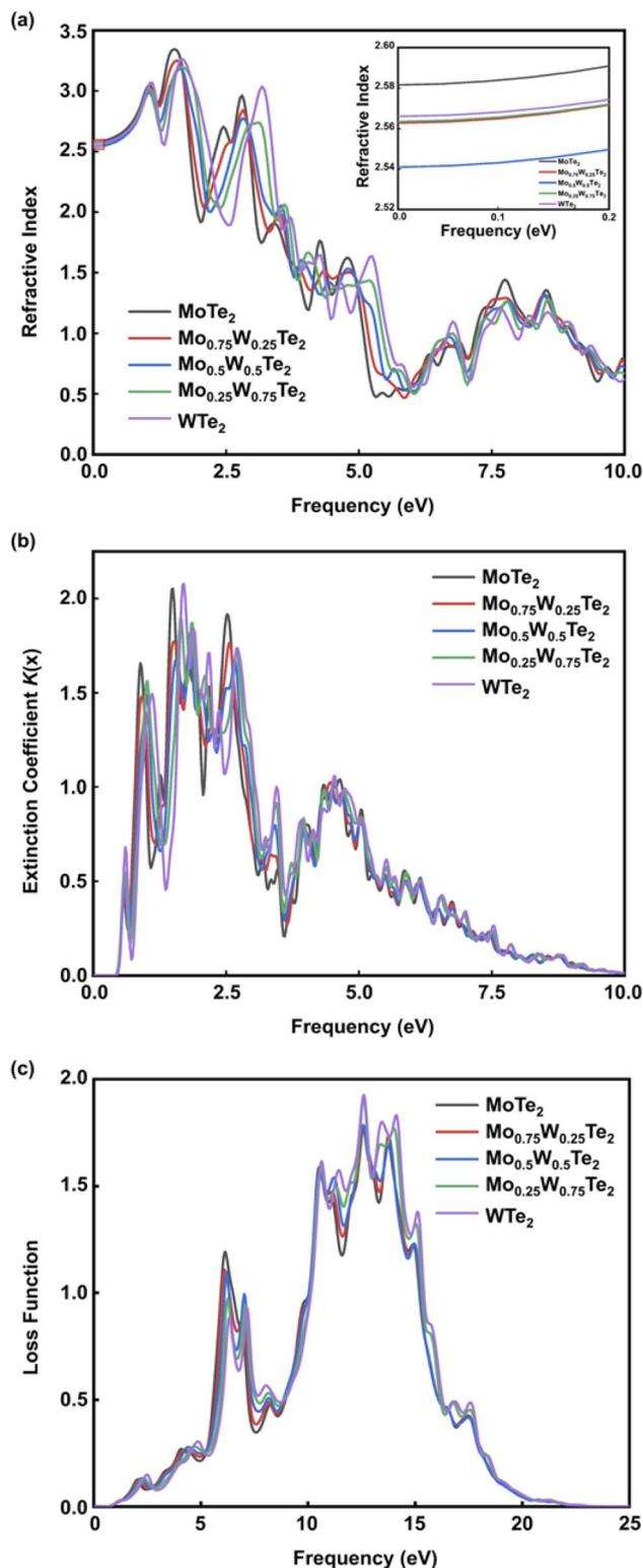
Fig. 7 (a) Refractive index of  $\text{Mo}_{1-x}\text{W}_x\text{Te}_2$  system. (b) Extinction coefficient of  $\text{Mo}_{1-x}\text{W}_x\text{Te}_2$  system. (c) Loss function of  $\text{Mo}_{1-x}\text{W}_x\text{Te}_2$  system.
