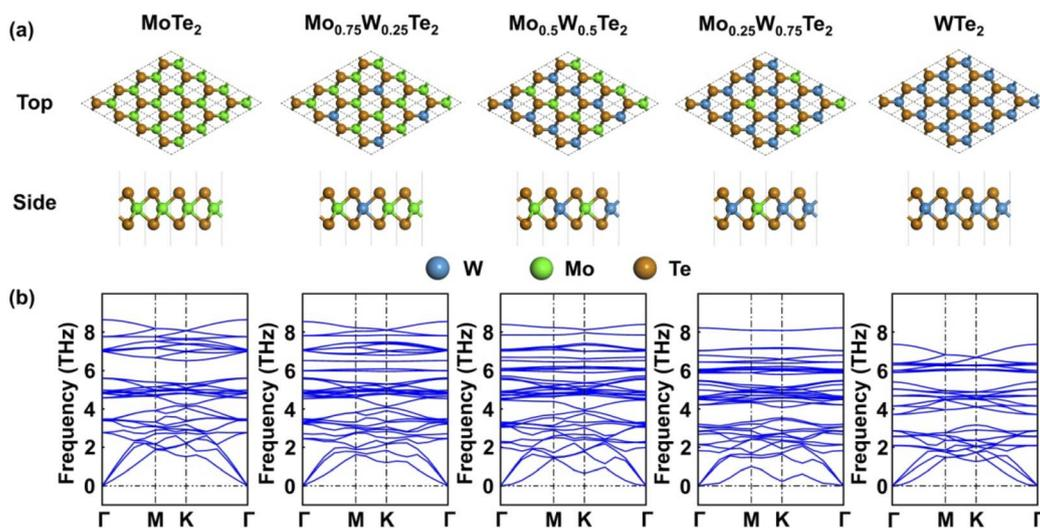
Fig. 2 (a) Top view and side view of the monolayer optimized structure of  $\text{Mo}_{1-x}\text{W}_x\text{Te}_2$  system when  $x = 0, 0.25, 0.5, 0.75, 1$ . (b) Monolayer phonon dispersion curves of the calculated  $\text{Mo}_{1-x}\text{W}_x\text{Te}_2$  system at  $x = 0, 0.25, 0.5, 0.75, 1$  (green, blue, and orange spheres represent Mo, W, and Te elements).
