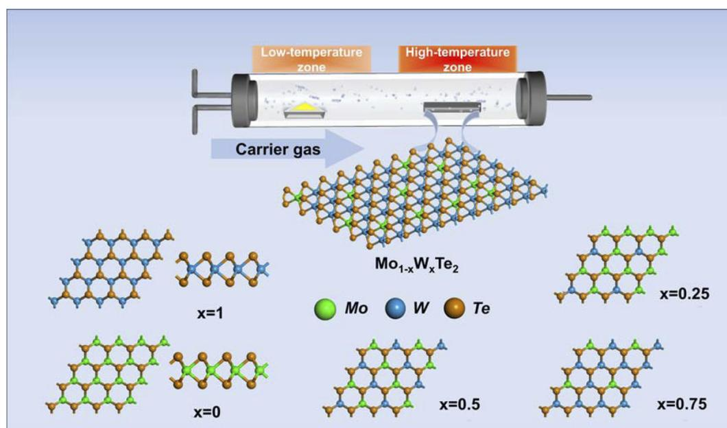
Fig. 1 Preparation diagram of monolayer  $\text{Mo}_{1-x}\text{W}_x\text{Te}_2$  system and structure diagram of  $\text{Mo}_{1-x}\text{W}_x\text{Te}_2$  system at  $x = 0, 0.25, 0.5, 0.75, 1$ .
