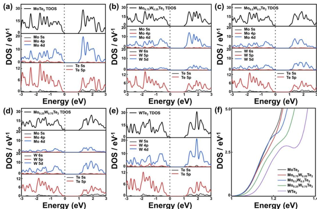
Fig. 4 Calculates the DOS structure of the  $\text{Mo}_{1-x}\text{W}_x\text{Te}_2$  system. (a) PDOS structure of  $\text{MoTe}_2$ . (b) PDOS structure of  $\text{Mo}_{0.75}\text{W}_{0.25}\text{Te}_2$ . (c) PDOS structure of  $\text{Mo}_{0.5}\text{W}_{0.5}\text{Te}_2$ . (d) PDOS structure of  $\text{Mo}_{0.25}\text{W}_{0.75}\text{Te}_2$ . (e) PDOS structure of  $\text{WTe}_2$ . (f) TDOS structure of the  $\text{Mo}_{1-x}\text{W}_x\text{Te}_2$  system.
