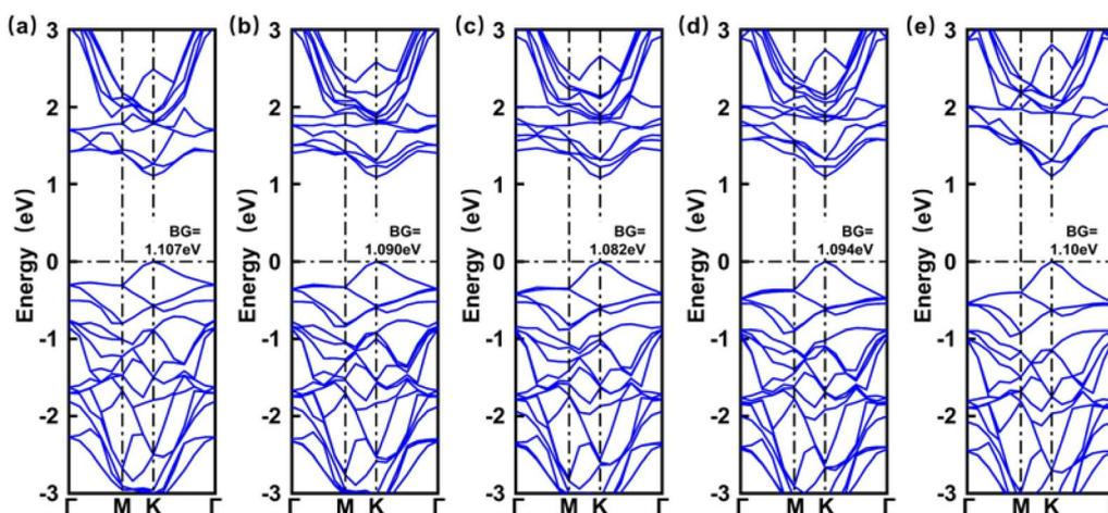
Fig. 3 Calculate the band structure of the  $\text{Mo}_{1-x}\text{W}_x\text{Te}_2$  system. (a) Band structure of  $\text{MoTe}_2$ . (b) Band structure of  $\text{Mo}_{0.75}\text{W}_{0.25}\text{Te}_2$ . (c) Band structure of  $\text{Mo}_{0.5}\text{W}_{0.5}\text{Te}_2$ . (d) Band structure of  $\text{Mo}_{0.25}\text{W}_{0.75}\text{Te}_2$ . (e) Band structure of  $\text{WTe}_2$ .
