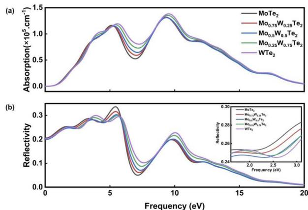
Fig. 6 (a) Absorption spectrum of  $\text{Mo}_{1-x}\text{W}_x\text{Te}_2$  system. (b) Reflection spectrum of  $\text{Mo}_{1-x}\text{W}_x\text{Te}_2$  system.
