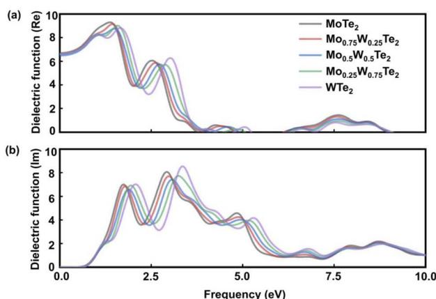
Fig. 5 Calculate the (a) real part and (b) imaginary part of the dielectric function of the  $\text{Mo}_{1-x}\text{W}_x\text{Te}_2$  system when  $x = 0, 0.25, 0.5, 0.75, 1$ .
