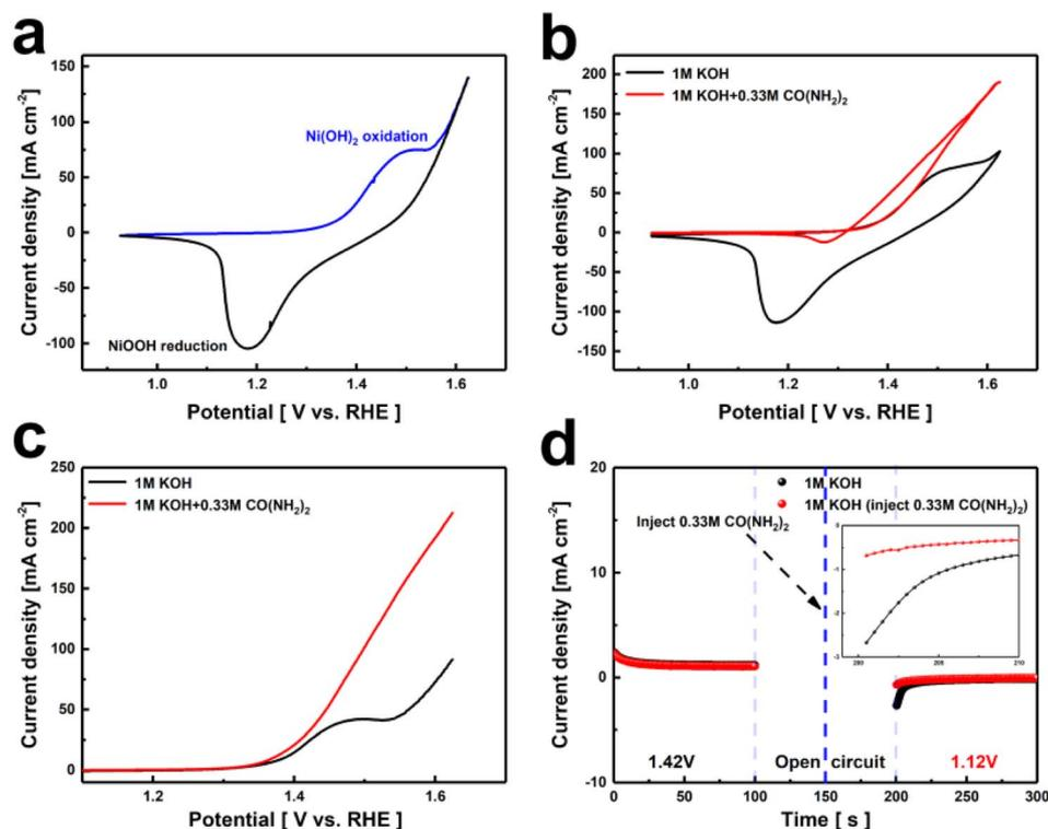
Fig. 1 (a and b) CV curves, (c) LSV curves of the  $\text{Ni}(\text{OH})_2$  electrode film in different media, (d) periodic chronocurrent measurement at 1.42 V (0–100 s), open-circuit state (100–200 s), and 1.12 V (200–300 s).
