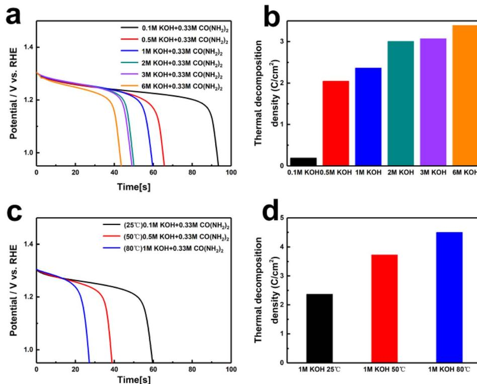
Fig. 3 (a and c) The self-discharge time, and (b and d) rate capability of NiOOH electrode in different OH<sup>-</sup> and different temperature for KOH with 0.33 M urea.
