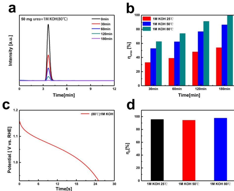
Fig. 5 (a) HPLC of urea decomposition on Ni(OH)<sub>2</sub> electrode in 1 M KOH concentration at 80 °C with the addition of 1 g L<sup>-1</sup> urea over 0–180 minutes. (b) The urea conversion rates at 25 °C, 50 °C, and 80 °C. (c) Discharge curve of Ni(OH)<sub>2</sub> electrode after 180 minutes of urea decomposition in 1 M KOH concentration at 80 °C at 100 mA. (d) The corresponding faradaic efficiencies of urea decomposition at Ni(OH)<sub>2</sub> electrodes with 25 °C, 50 °C, and 80 °C.
