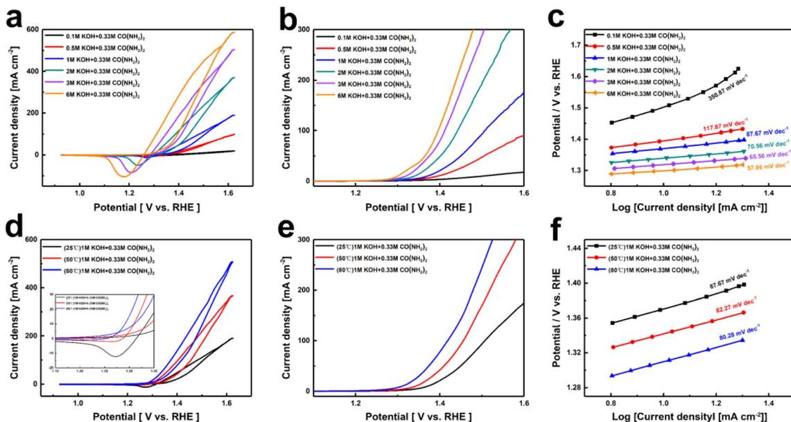
Fig. 2 (a) CV curves, (b) LSV curves, (c) Tafel slopes of Ni(OH)<sub>2</sub> electrode film for different OH<sup>-</sup>, (d) CV curves, (e) LSV curves, (f) Tafel slopes of Ni(OH)<sub>2</sub> electrode film in the 1 M KOH and 0.33 M urea at different temperatures.
