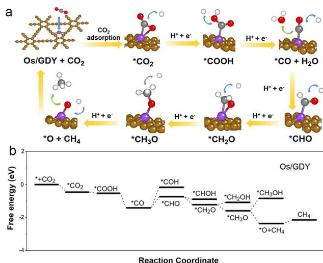
Fig. 6 Reaction mechanism of  $CO_2RR$  to  $CH_4$  on  $Os_1/GDY$ . (a) The structure of the reaction intermediates; (b) different energy profiles. The CHE model and the DFT method of PBE functional are used to calculate the path.
