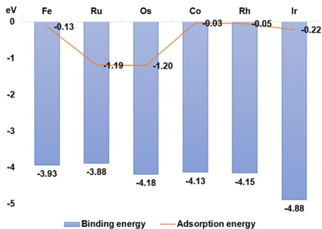
Fig. 3 The binding energy of GDY-loaded Fe, Ru, Os, Co, Rh, and Ir single atoms and CO<sub>2</sub> adsorption energy.
