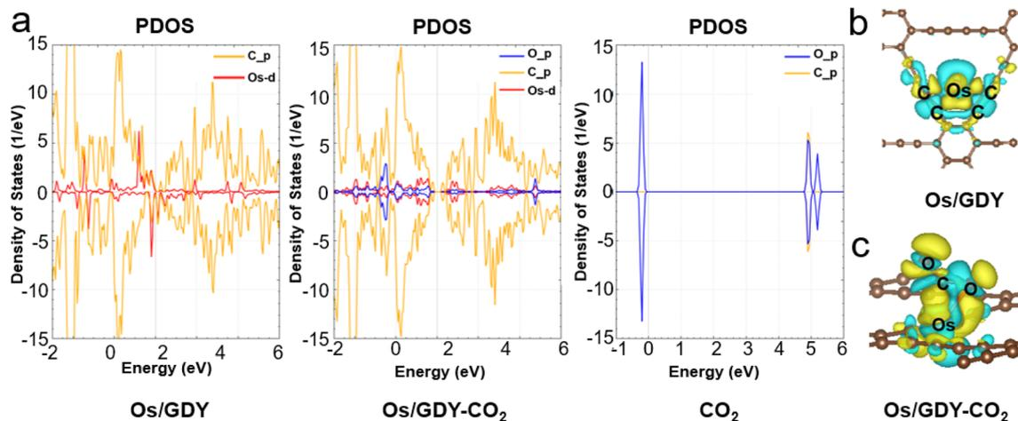
Fig. 4 (a) The schematic diagram of projected electronic densities of states of Os<sub>1</sub>/GDY, Os<sub>1</sub>/GDY-CO<sub>2</sub>, and CO<sub>2</sub>. CDD plots of (b) Os<sub>1</sub>/GDY and (c) Os<sub>1</sub>/GDY-CO<sub>2</sub>.
