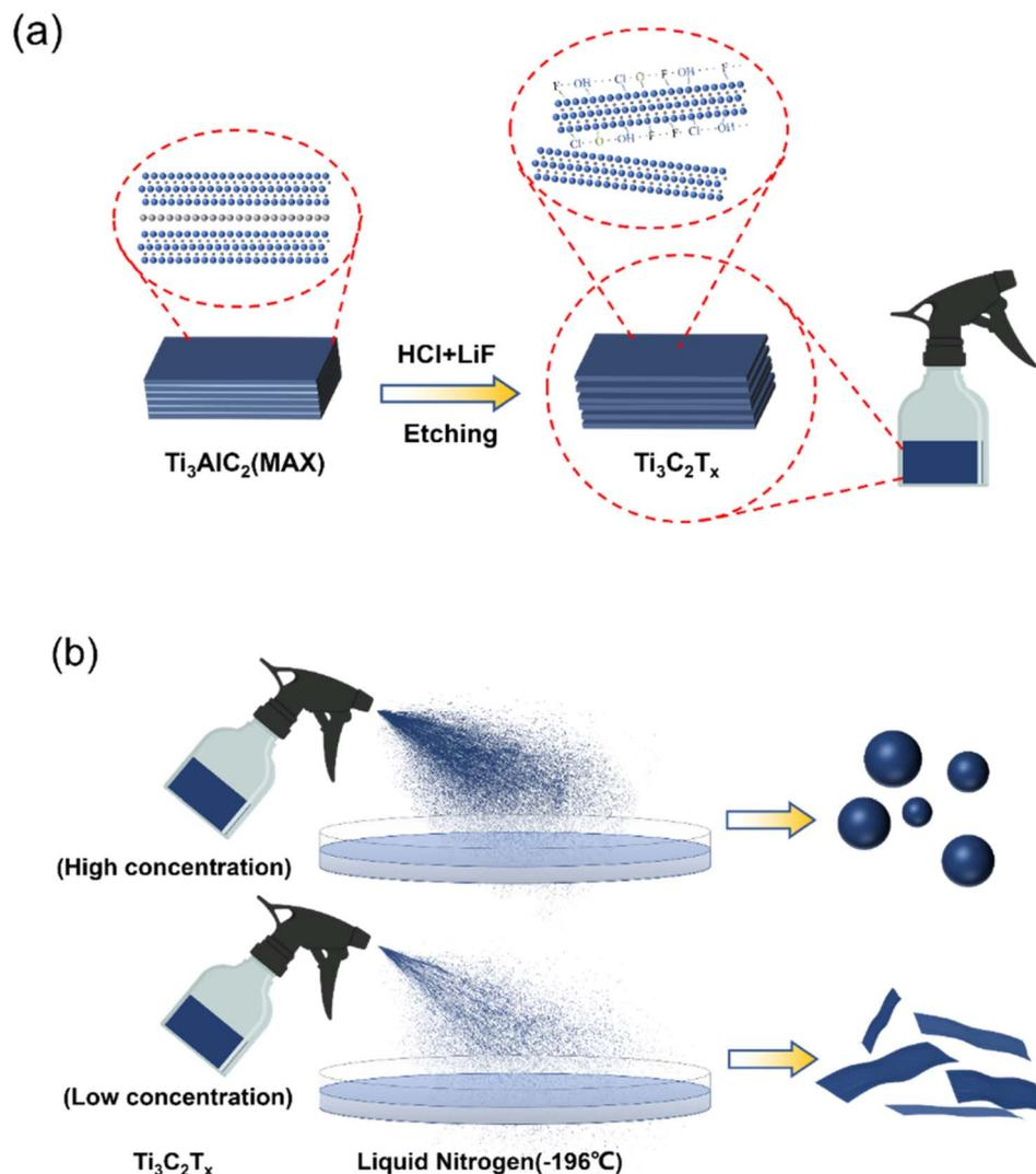
Fig. 1 (a) Preparation process of the few-layer  $\text{Ti}_3\text{C}_2\text{T}_x$ ; (b) preparation of the flaky and spherical  $\text{Ti}_3\text{C}_2\text{T}_x$  by spray freezing method.
