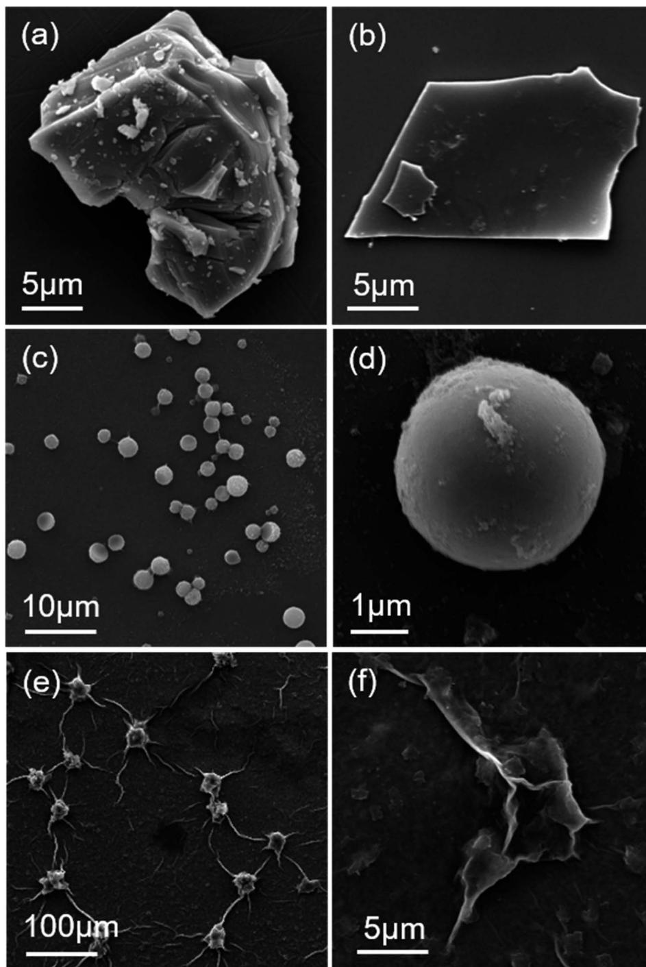
Fig. 3 SEM images of (a) precursor  $\text{Ti}_3\text{AlC}_2$ , (b) few-layer  $\text{Ti}_3\text{C}_2\text{T}_x$ , (c and d) spherical  $\text{Ti}_3\text{C}_2\text{T}_x$ , and (e and f) flaky  $\text{Ti}_3\text{C}_2\text{T}_x$ .
