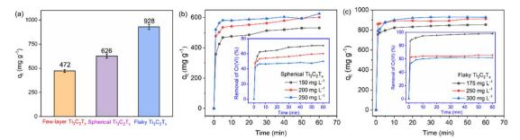
Fig. 4 (a) The change of adsorption capacity and removal rate of spherical  $Ti_3C_2T_x$  with time; (b) the change of adsorption capacity and removal rate of flaky  $Ti_3C_2T_x$  with time; (c) comparison diagram of Cr(vi) maximum adsorption capacity of the few-layer  $Ti_3C_2T_x$ , the spherical  $Ti_3C_2T_x$  and the flaky  $Ti_3C_2T_x$ .
