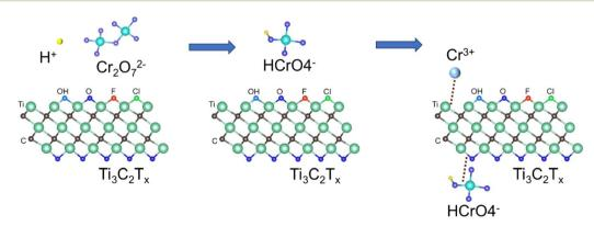
Fig. 10 Schematic diagram of adsorption mechanism of Cr(vi) on Ti<sub>3</sub>C<sub>2</sub>T<sub>v</sub>.
