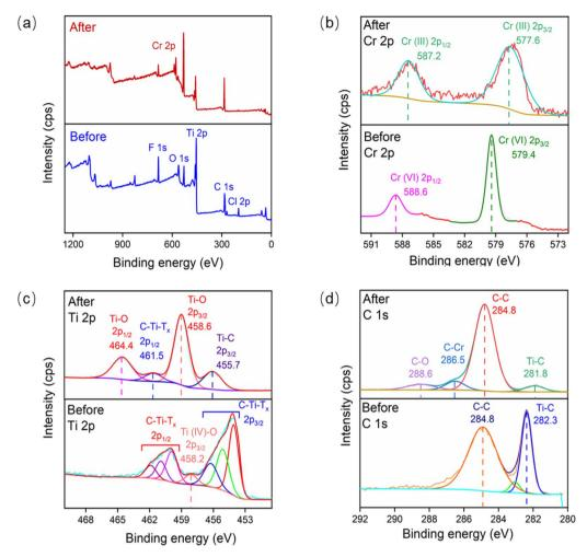
Fig. 9 Comparison of XPS spectra of  $Ti_3C_2T_x$  before and after adsorption: (a) full spectrum, (b) Cr 2p, (c) Ti 2p, (d) C 1s.
