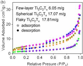
Fig. 2 (a) XRD patterns of precursor  $Ti_3AlC_2$ , few-layer  $Ti_3C_2T_x$ , spherical and flaky  $Ti_3C_2T_x$ ; (b)  $N_2$  adsorption-desorption isotherm diagram of the few-layer  $Ti_3C_2T_x$ , spherical  $Ti_3C_2T_x$  and flaky  $Ti_3C_2T_x$ .
