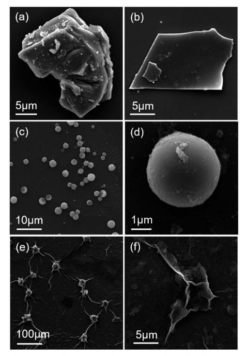
Fig. 3 SEM images of (a) precursor  $Ti_3AlC_2$ , (b) few-layer  $Ti_3C_2T_x$ , (c and d) spherical  $Ti_3C_2T_x$ , and (e and f) flaky  $Ti_3C_2T_x$ .
