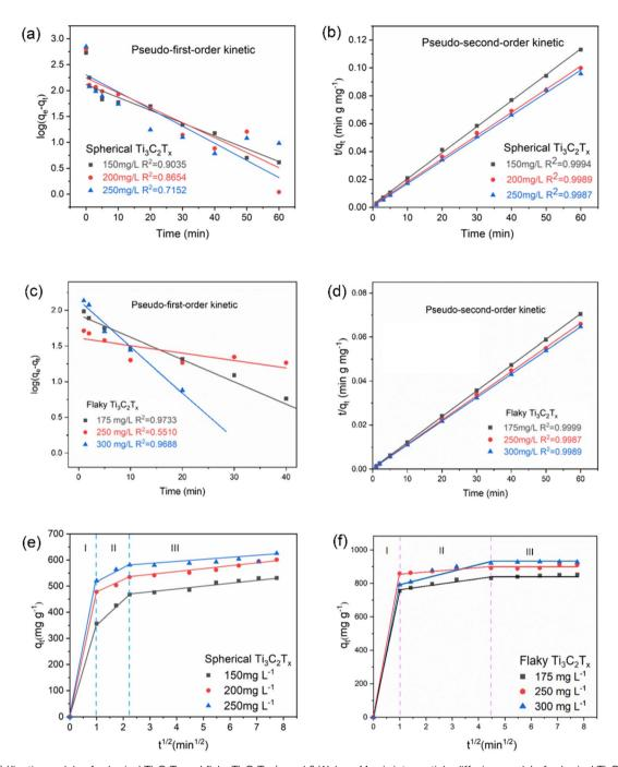
Fig. 5 (a-d) Kinetic models of spherical  $Ti_3C_2T_x$  and flaky  $Ti_3C_2T_{xi}$  (e and f) Weber-Morris intraparticle diffusion model of spherical  $Ti_3C_2T_x$  and flaky  $Ti_3C_2T_{xi}$ .
