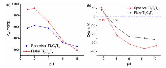
Fig. 8 (a) Maximum adsorption of  $Cr(v_1)$  by spherical and flaky  $Ti_3C_2T_x$  at pH 1, 2, 4, 6, 8 (b) zeta potentials of spherical and flaky  $Ti_3C_2T_x$  at different pH.
