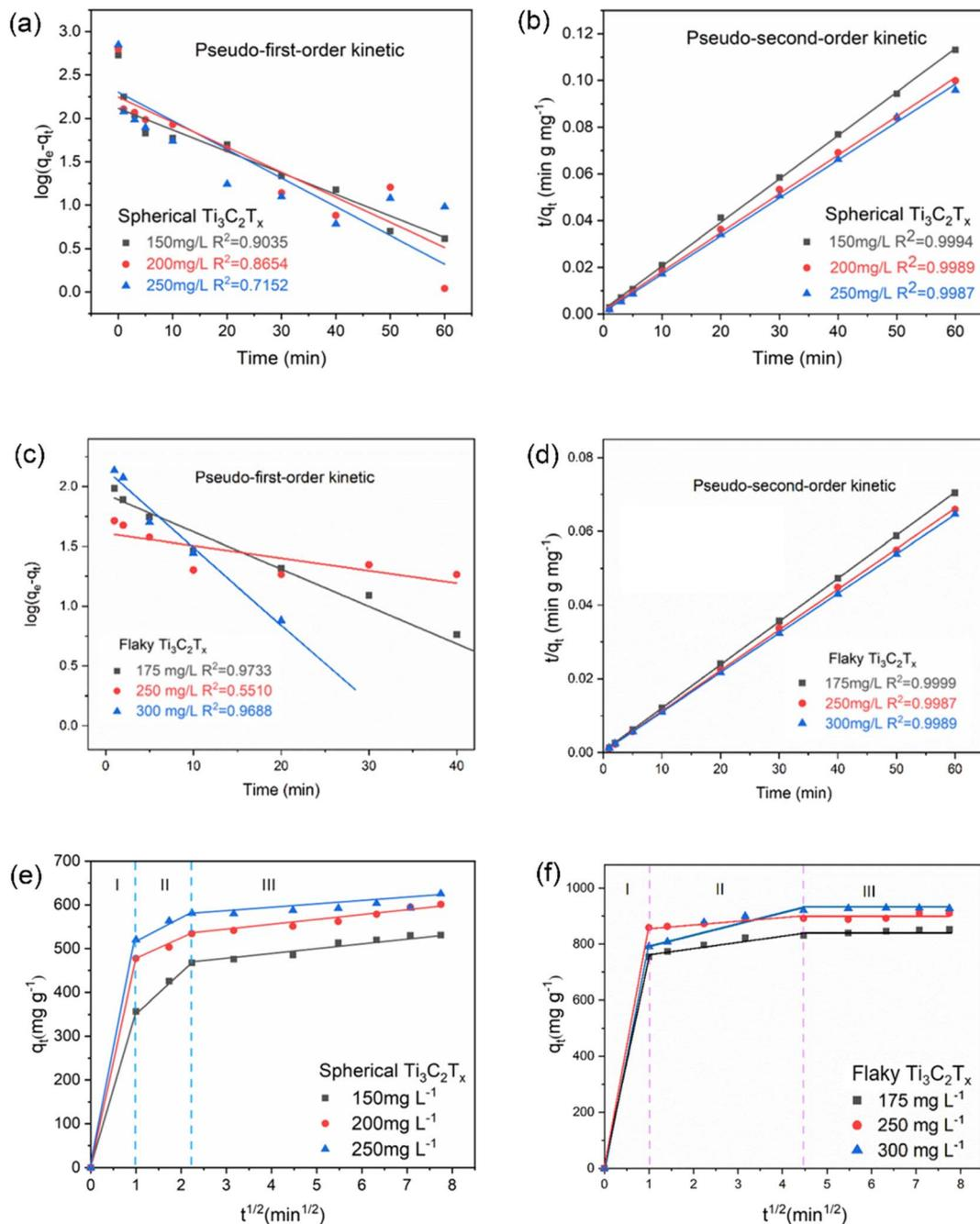
Fig. 5 (a–d) Kinetic models of spherical  $\text{Ti}_3\text{C}_2\text{T}_x$  and flaky  $\text{Ti}_3\text{C}_2\text{T}_x$ ; (e and f) Weber–Morris intraparticle diffusion model of spherical  $\text{Ti}_3\text{C}_2\text{T}_x$  and flaky  $\text{Ti}_3\text{C}_2\text{T}_x$ .
