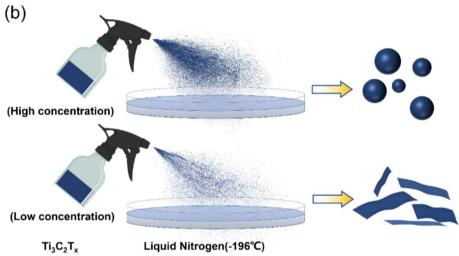
Fig. 1 (a) Preparation process of the few-layer  $Ti_3C_2T_x$ . (b) preparation of the flaky and spherical  $Ti_3C_2T_x$  by spray freezing method.
