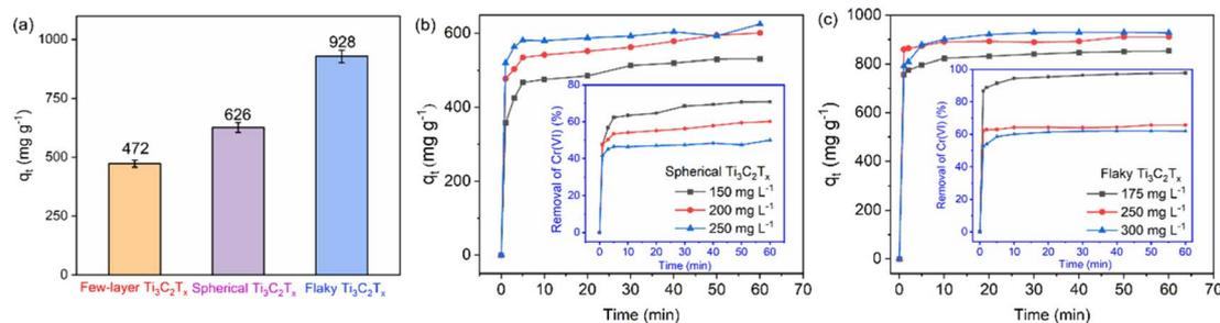
Fig. 4 (a) The change of adsorption capacity and removal rate of spherical  $Ti_3C_2T_x$  with time; (b) the change of adsorption capacity and removal rate of flaky  $Ti_3C_2T_x$  with time; (c) comparison diagram of Cr(vi) maximum adsorption capacity of the few-layer  $Ti_3C_2T_x$ , the spherical  $Ti_3C_2T_x$  and the flaky  $Ti_3C_2T_x$ .
