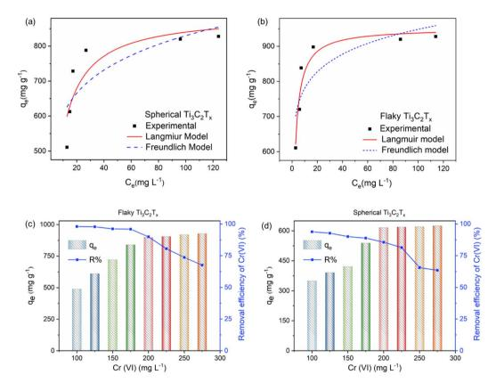
Fig. 6 Langmuir and Freundlich isotherm models of (a) spherical  $Ti_3C_2T_x$  and (b) flaky  $Ti_3C_2T_x$ : (c and d) The removal efficiency and maximum adsorption capacity of spherical  $Ti_3C_2T_x$  and flaky  $Ti_3C_2T_x$  as a function of  $Cr(v_1)$  concentration.
