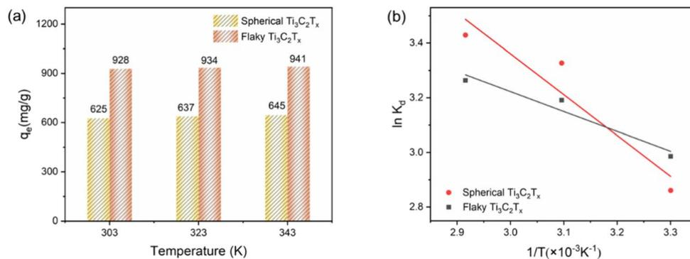
Fig. 7 (a) Graph of adsorption capacity of spherical  $Ti_3C_2T_x$  and flaky  $Ti_3C_2T_x$  with temperature; (b) van der Waals equation fitting graphs of spherical  $Ti_3C_2T_x$  and flaky  $Ti_3C_2T_x$  at different temperatures.
