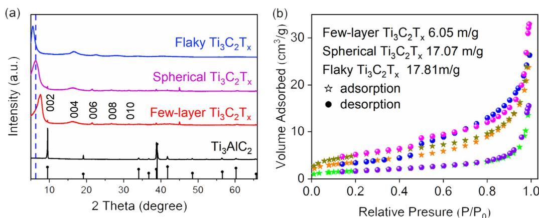
Fig. 2 (a) XRD patterns of precursor  $\text{Ti}_3\text{AlC}_2$ , few-layer  $\text{Ti}_3\text{C}_2\text{T}_x$ , spherical and flaky  $\text{Ti}_3\text{C}_2\text{T}_x$ ; (b)  $\text{N}_2$  adsorption-desorption isotherm diagram of the few-layer  $\text{Ti}_3\text{C}_2\text{T}_x$ , spherical  $\text{Ti}_3\text{C}_2\text{T}_x$  and flaky  $\text{Ti}_3\text{C}_2\text{T}_x$ .
