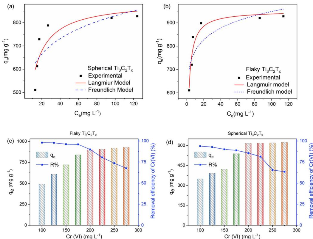
Fig. 6 Langmuir and Freundlich isotherm models of (a) spherical Ti<sub>3</sub>C<sub>2</sub>T<sub>x</sub> and (b) flaky Ti<sub>3</sub>C<sub>2</sub>T<sub>x</sub>; (c and d) The removal efficiency and maximum adsorption capacity of spherical Ti<sub>3</sub>C<sub>2</sub>T<sub>x</sub> and flaky Ti<sub>3</sub>C<sub>2</sub>T<sub>x</sub> as a function of Cr(vi) concentration.
