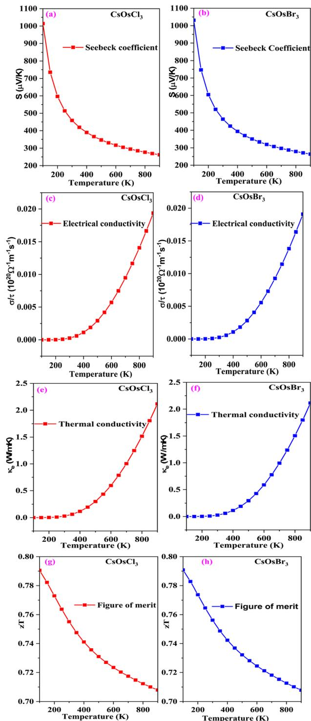
Fig. 6 (a–h) The variation of Seebeck (a and b), electrical conductivity (c and d), thermal conductivity (e and f) and figure of merit (g and h) with temperature for CsOsX<sub>3</sub> (X = Cl, Br) alloys.
