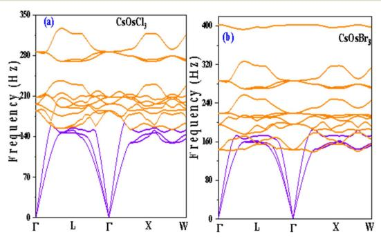
Fig. 3 (a and b) Phonon dispersions along the high symmetric directions of Brillouin zone of CsOs $X_3$  (X = Cl, Br) alloys.
