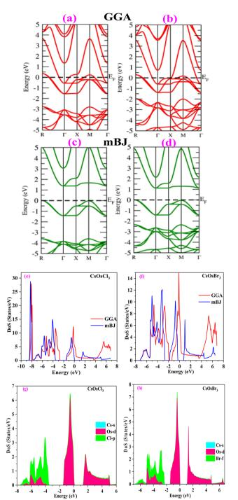
Fig. 4 (a–h) Band structure by GGA (red colour), mBJ (green colour) approximation and density of states [total (e and f) and partial (g and h)] of  $CsOsX_3$  (X = Cl, Br) alloys.
