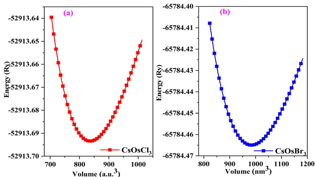
Fig. 2 (a and b) Optimization plot of CsOsX<sub>3</sub> (X = Cl, Br) alloys.
