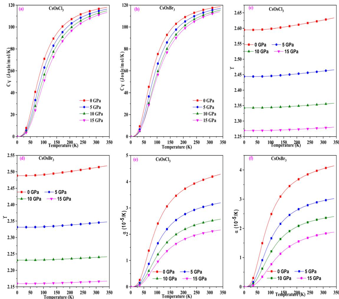
Fig. 5 (a–f) The variation of specific heat, Gruneisen parameter and thermal expansion with temperature for CsOsX<sub>3</sub> (X = Cl, Br) alloys.
