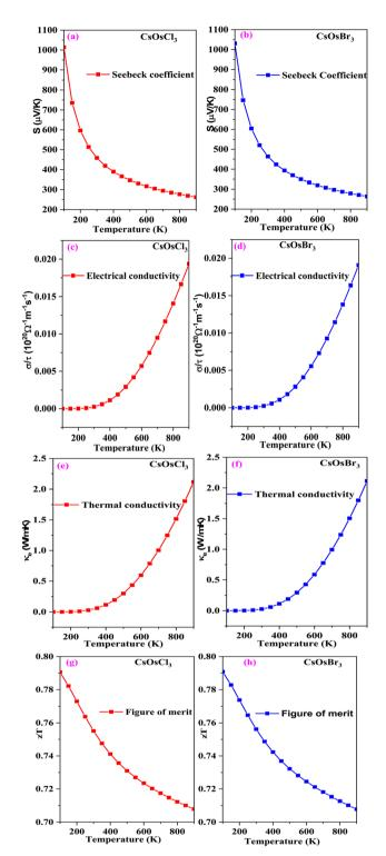
Fig. 6 (a–h) The variation of Seebeck (a and b), electrical conductivity (c and d), thermal conductivity (e and f) and figure of merit (g and h) with temperature for  $CsOsX_3$  (X = Cl, Br) alloys.
