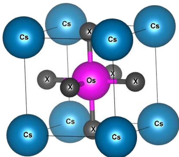
Fig. 1 Crystal structure of CsOsX<sub>3</sub> (X = Cl, Br) alloys.
