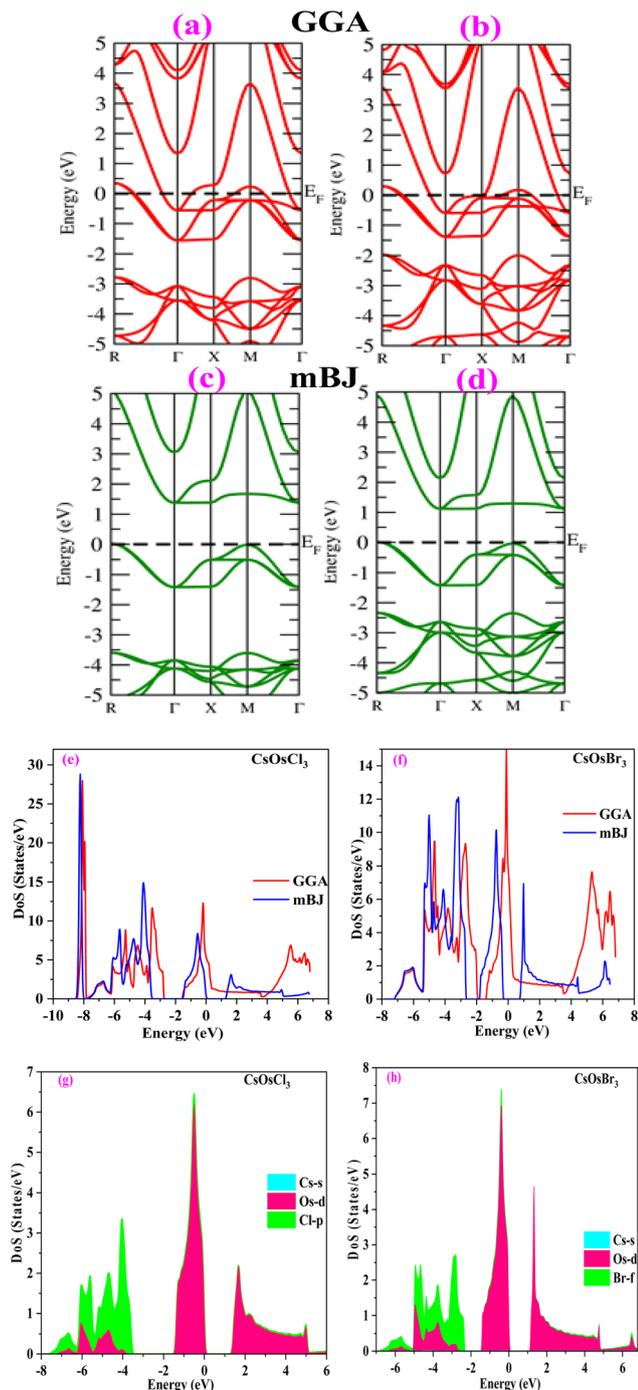
Fig. 4 (a–h) Band structure by GGA (red colour), mBJ (green colour) approximation and density of states [total (e and f) and partial (g and h)] of CsOsX<sub>3</sub> (X = Cl, Br) alloys.
