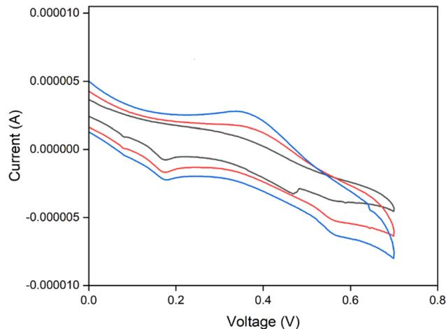
Fig. 20 Cyclic voltammetry curve for CuO nanoparticles.
