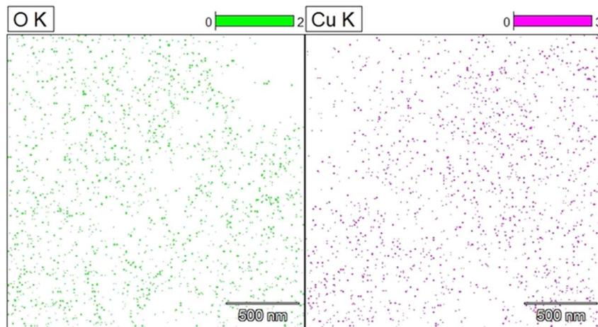
Fig. 7 Elemental mapping of the synthesized CuO nanoparticles.
