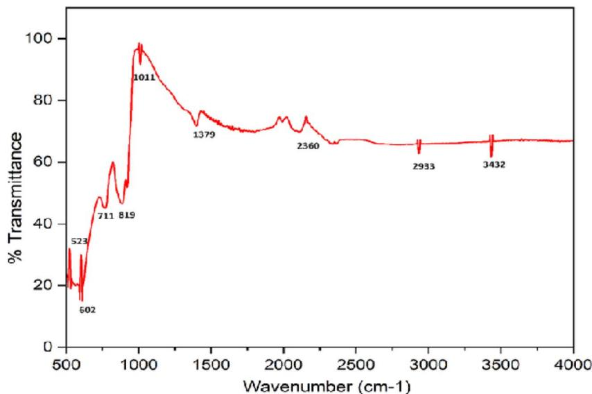
Fig. 4 FTIR spectrum of the synthesized CuO nanoparticles.
