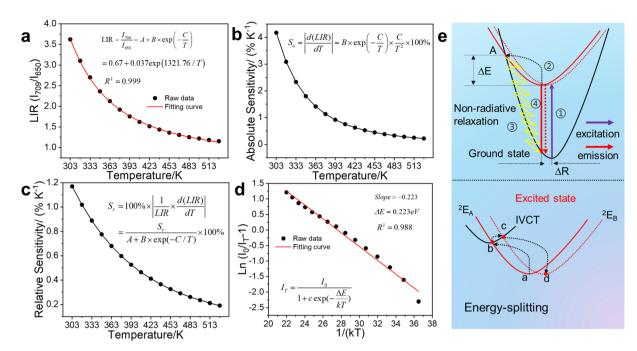
Fig. 5 (a) LIR thermometry as a temperature linear relationship, (b) absolute and (c) relative sensitivity, and (d) the relationship of  $\ln[(I_0/I_T) - 1]$  to 1/(kT) of MGCP under 222 nm excitation at the temperature from 303 to 528 K. (e) The thermal quenching of MGCP explained by configuration coordinate model and intervalence charge transfer.
