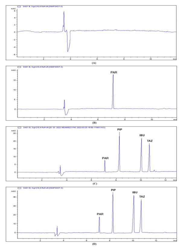
Fig. 3 Capillary electropherogram of (A) blank plasma; (B) plasma sample spiked with 50  $\mu$ g per mL IS, and scanning at 210 nm; (C) plasma sample spiked with 50  $\mu$ g per mL IS, 60  $\mu$ g per mL PIP, 50  $\mu$ g per mL IBU, 20  $\mu$ g per mL TAZ, and scanning at 210 nm; (D) real rat plasma sample spiked with 50  $\mu$ g per mL IS and elution of the studied drugs PIP, IBU, and TAZ, and scanning at 210 nm.
