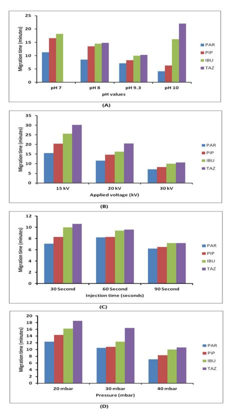
Fig. 2 (A) Effect of borate buffer at different pH values on the compounds' migration time. (B) Effect of applied voltage (kV) on the compounds' migration time. (C) Effect of injection time (seconds) on the compounds' migration time. (D) Effect of pressure (mbar) on the compounds' migration time.
