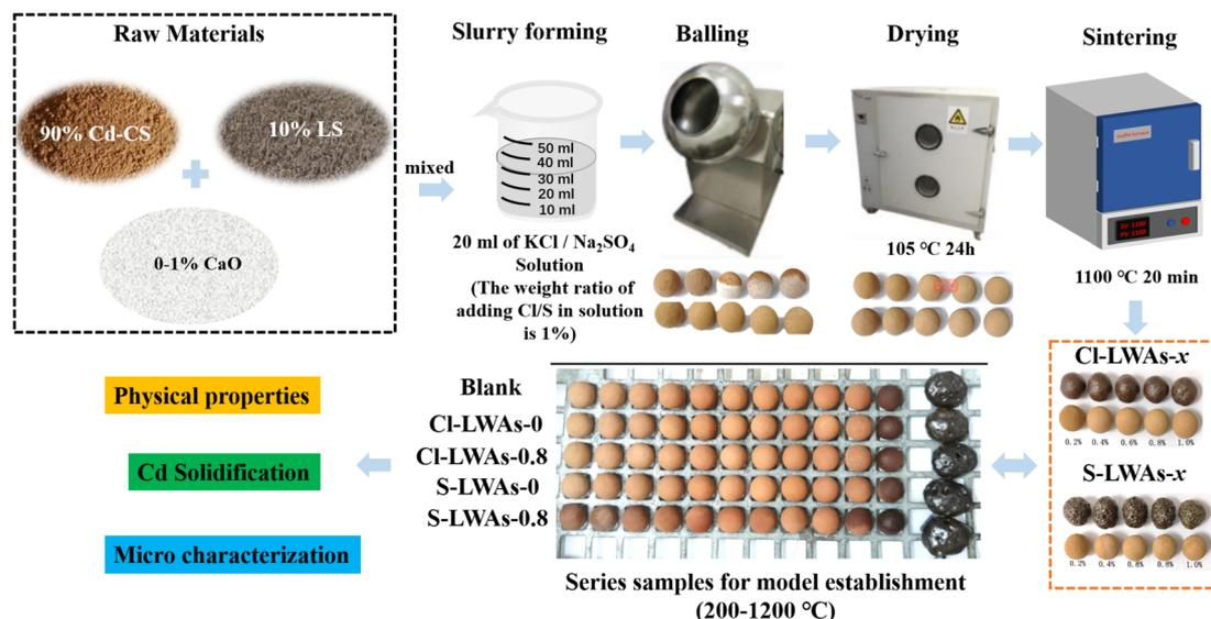
Scheme 1 Schematic diagram of the LWAs preparation process.
