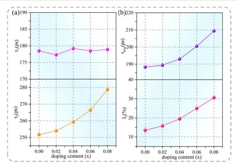
(a) Positron lifetime components,  $\tau_1$  and  $\tau_2$ ; (b)  $\tau_{\text{ave}}$  and  $I_2$  as functions of the Na<sup>+</sup> doping content in Cd<sub>1-x</sub>Na<sub>x</sub>Cu<sub>3</sub>Ti<sub>4</sub>O<sub>12</sub> ceramics.
