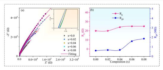
Fig. 8 (a) Complex impedance plots of  $Cd_{1-x}Na_xCu_3Ti_4O_{12}$  ceramics at room temperature; the inset shows an expanded view of the highfrequency data close to the origin; (b)  $R_{\rm q}$  and  $R_{\rm qb}$  parameters as functions of x.
