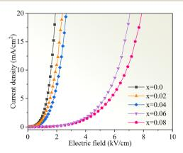
Fig. 11 Nonlinear J-E plots of the  $Cd_{1-x}Na_xCu_3Ti_4O_{12}$  ceramics.
