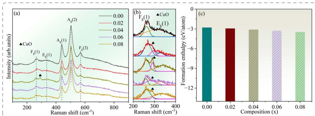
Fig. 2 (a) Raman spectra, (b) the deconvoluted Raman spectra and (c) formation enthalpy of the  $\text{Cd}_{1-x}\text{Na}_x\text{Cu}_3\text{Ti}_4\text{O}_{12}$  ceramics determined via first-principles calculations.
