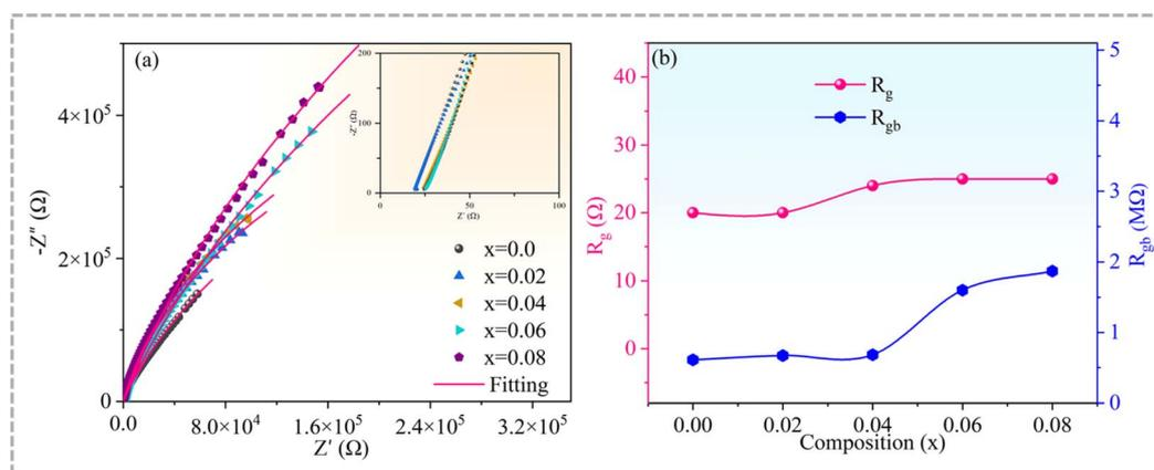
Fig. 8 (a) Complex impedance plots of  $\text{Cd}_{1-x}\text{Na}_x\text{Cu}_3\text{Ti}_4\text{O}_{12}$  ceramics at room temperature; the inset shows an expanded view of the high-frequency data close to the origin; (b)  $R_g$  and  $R_{\text{gb}}$  parameters as functions of  $x$ .
