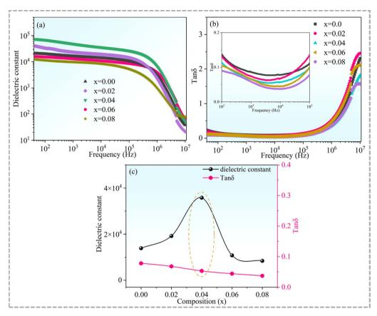
Fig. 7 (a) Dielectric constant and (b) dielectric loss of  $Cd_{1-x}Na_xCu_3Ti_4O_{12}$  ceramics as functions of frequency; the inset presents the magnified view in the frequency range from 100 to 10<sup>5</sup> Hz; (c) dielectric constant and dielectric loss as a function of Na<sup>+</sup> contents at 10 kHz.
