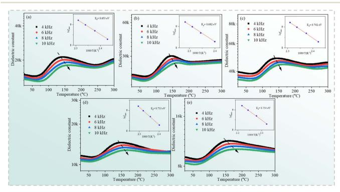
Fig. 10 Temperature dependence of the dielectric constant for the  $Cd_{1-x}Na_xCu_3Ti_4O_{12}$  ceramics (a) x=0.0; (b) x=0.02; (c) x=0.04; (d) x=0.06; (e) x=0.08.
