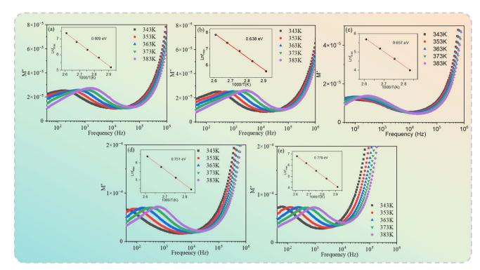
Fig. 9 Electric modulus (M'') as a function of the frequency of  $Cd_{1-x}Na_xCu_3Ti_4O_{12}$  ceramics: (a) x=0, (b) x=0.02, (c) x=0.04, (d) x=0.06, and (e) x=0.08.
