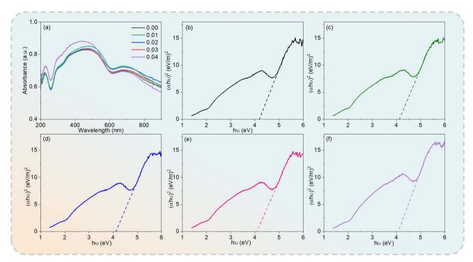
Fig. 6 (a) UV-vis absorption spectra of  $Cd_{1-x}Na_xCu_3Ti_4O_{12}$  ceramics and  $(\alpha h\nu)^2$  versus  $h\nu$  plots at (b) x=0.0; (c) x=0.02; (d) x=0.04; (e) x=0.06; (f) x=0.08.
