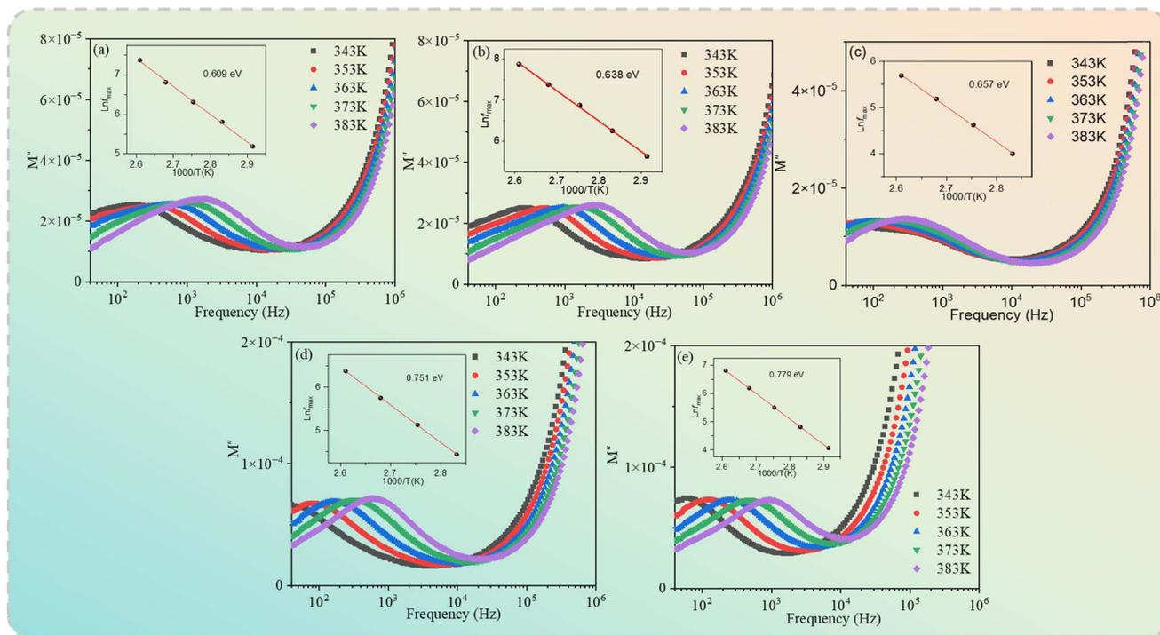
Fig. 9 Electric modulus ( $M''$ ) as a function of the frequency of  $\text{Cd}_{1-x}\text{Na}_x\text{Cu}_3\text{Ti}_4\text{O}_{12}$  ceramics: (a)  $x = 0$ , (b)  $x = 0.02$ , (c)  $x = 0.04$ , (d)  $x = 0.06$ , and (e)  $x = 0.08$ .
