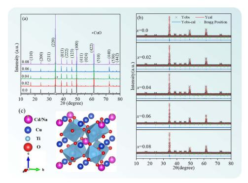
Fig. 1 (a) XRD patterns of  $Cd_{1-x}Na_xCu_3Ti_4O_{12}$  ceramics; Rietveld refinement plots in the case of (b) CdCTO and (c) BCTO; (d) crystal structure of  $Cd_{1-x}Na_xCu_3Ti_4O_{12}$ .
