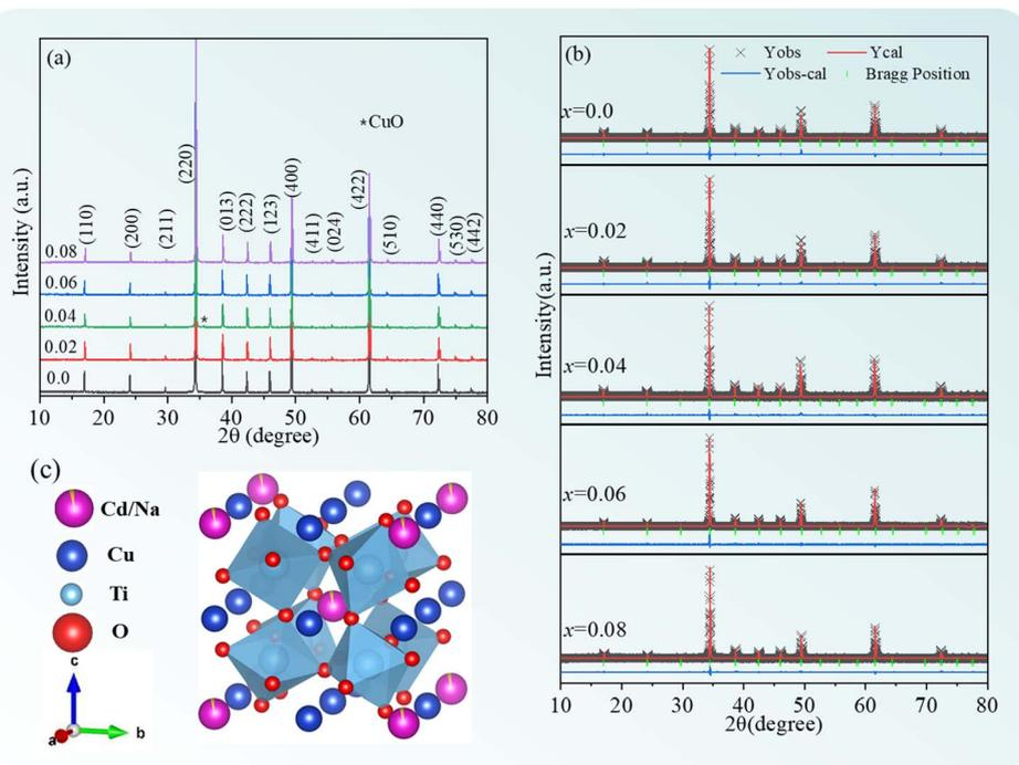
Fig. 1 (a) XRD patterns of  $\text{Cd}_{1-x}\text{Na}_x\text{Cu}_3\text{Ti}_4\text{O}_{12}$  ceramics; Rietveld refinement plots in the case of (b) CdCTO and (c) BCTO; (d) crystal structure of  $\text{Cd}_{1-x}\text{Na}_x\text{Cu}_3\text{Ti}_4\text{O}_{12}$ .
