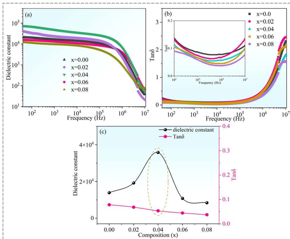
Fig. 7 (a) Dielectric constant and (b) dielectric loss of  $\text{Cd}_{1-x}\text{Na}_x\text{Cu}_3\text{Ti}_4\text{O}_{12}$  ceramics as functions of frequency; the inset presents the magnified view in the frequency range from 100 to  $10^5$  Hz; (c) dielectric constant and dielectric loss as a function of  $\text{Na}^+$  contents at 10 kHz.
