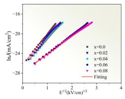
Fig. 12 The  $\ln J$  versus  $E^{1/2}$  plots for the  $Cd_{1-x}Na_xCu_3Ti_4O_{12}$  ceramics.
