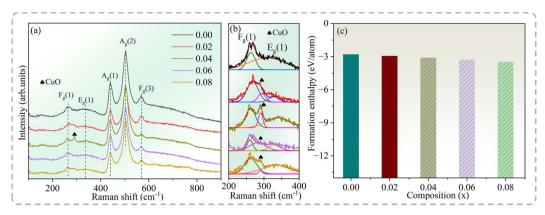
Fig. 2 (a) Raman spectra, (b) the deconvoluted Raman spectra and (c) formation enthalpy of the  $Cd_{1-x}Na_xCu_3Ti_4O_{12}$  ceramics determined via first-principles calculations.
