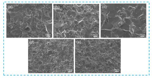
Fig. 3 Cross-sectional SEM images of  $Cd_{1-x}Na_xCu_3Ti_4O_{12}$  ceramics: (a) x = 0; (b) x = 0.02; (c) x = 0.04; (d) x = 0.06; (e) x = 0.08.
