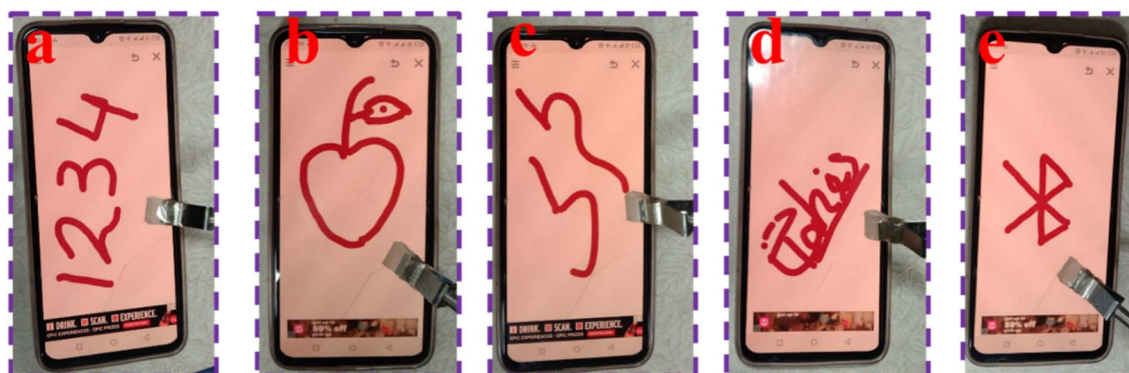
Fig. 9 The use of organohydrogel as an electronic pen for (a) writing (b) drawing (c) language identification (d) signature (e) bluetooth symbol.
