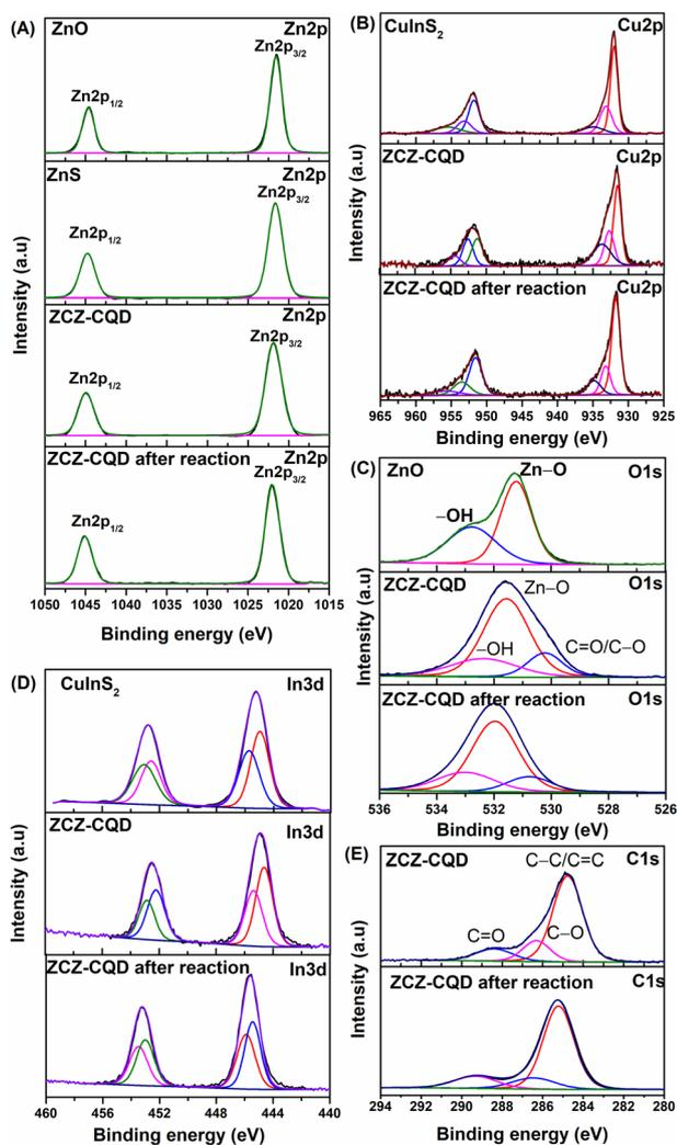
Fig. 3 High-resolution Zn 2p (A), Cu 2p (B), O 1s (C), In 3d (D) and C 1s (E) XPS spectra of ZnO, CuInS<sub>2</sub>, ZnS and ZCZ-CQD and CZC-CQD after 10 cycles.
