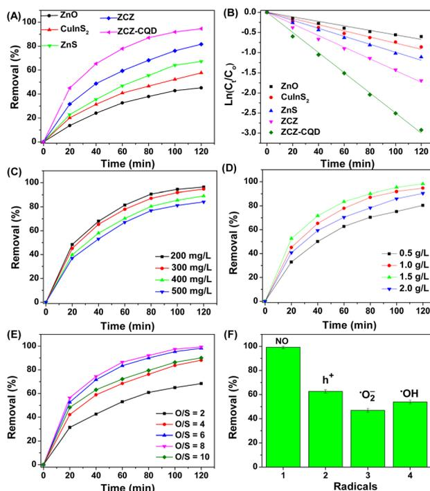
Fig. 7 (A) Removal efficiency of DBT, (B) pseudo-first-order kinetic models of ZnO, CuInS<sub>2</sub>, ZnS, ZCZ and ZCZ–CQD photocatalysts; removal efficiency of DBT over ZCZ–CQD photocatalyst at different DBT concentrations (C), catalysts dose (D), O/S molar ratio (E), reactive radicals (F).
