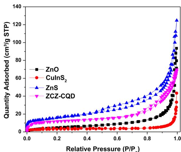
Fig. 4 N<sub>2</sub> adsorption-desorption isotherms of CuInS<sub>2</sub>, ZnO, ZnS, and ZCZ-CQD samples.
