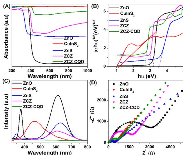
Fig. 6 UV-vis DRS spectrum (A), bandgap energy ( $E_g$ ) (B), photoluminescence spectra (C), EIS spectra (D) of ZnO, CuInS<sub>2</sub>, ZnS, ZCZ and ZCZ-CQD samples.
