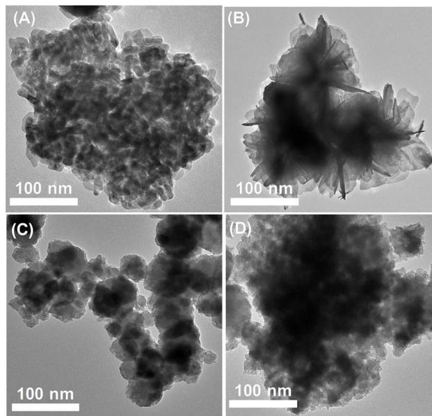
Fig. 5 TEM images of ZnO (A), CuInS<sub>2</sub> (B), ZnS (C) and ZCZ-CQD (D) samples.
