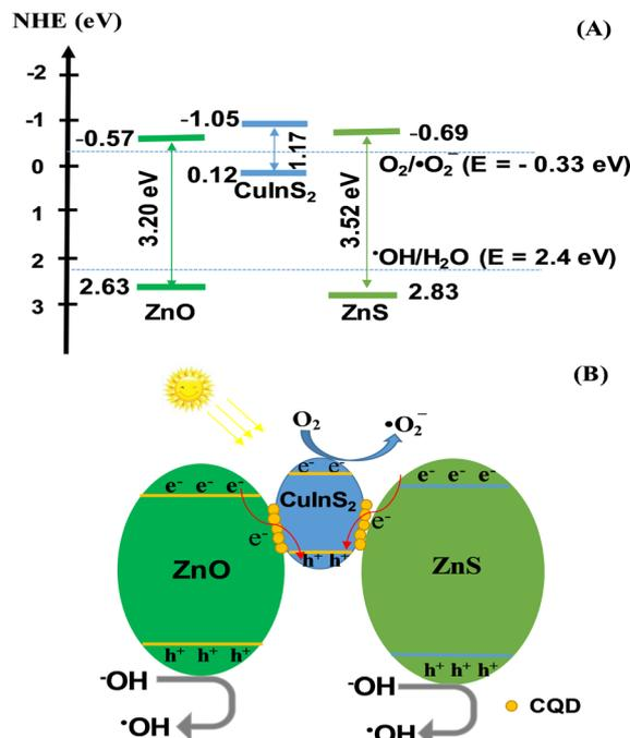
Fig. 8 Mechanism diagram of the charge transfer before contact (A) and possible Z-scheme (B) of ZnO, CuInS<sub>2</sub>, ZnS, and ZCZ-CQD.
