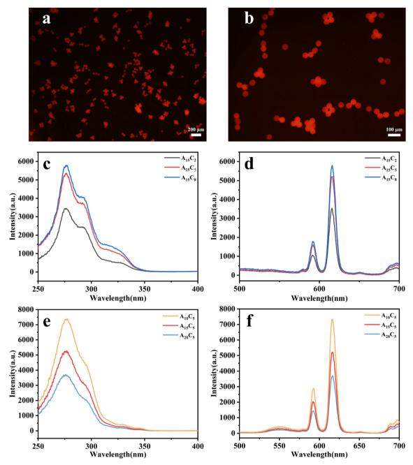
Fig. 5 (a and b) Fluorescence micrographs of porous hydrogel microspheres; (c and e) excitation and (d and f) emission spectra of porous hydrogel microspheres.
