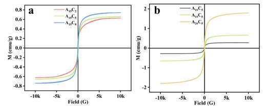
Fig. 4 Hysteresis loops of porous hydrogel microspheres: (a) A<sub>15</sub>C<sub>2</sub>, A<sub>15</sub>C<sub>5</sub>, and A<sub>15</sub>C<sub>8</sub>; (b) A<sub>10</sub>C<sub>5</sub>, A<sub>15</sub>C<sub>5</sub>, and A<sub>20</sub>C<sub>5</sub>.
