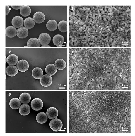
Fig. 2 SEM images of porous hydrogel microspheres: (a and b)  $A_{10}C_5$ ; (c and d)  $A_{15}C_5$ ; (e and f)  $A_{20}C_5$  (three samples were prepared with the same flow rate of the continuous/disperse phase of 20  $\mu$ L min<sup>-1</sup>/5  $\mu$ L min<sup>-1</sup>).
