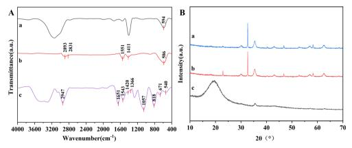
Fig. 3 (A) FTIR spectra and (B) XRD patterns of Fe<sub>3</sub>O<sub>4</sub> (a), OA/NaUA-Fe<sub>3</sub>O<sub>4</sub> (b), A<sub>15</sub>C<sub>8</sub> (c).
