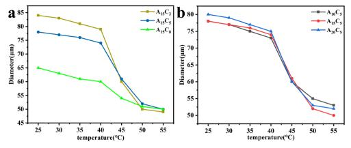
Fig. 6 Effect of temperature on the diameter of porous hydrogel microspheres with (a) different concentration of  $A_{15}$  nanospheres and (b) different nanospheres ( $A_{10}$ ,  $A_{15}$ ,  $A_{20}$ ) of 5 wt% concentration.
