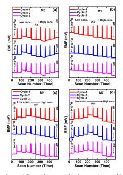
Fig. 13 Cycling stability performance for the membrane (a) M0, (b) M1, (c) M4 and (d) M7.
