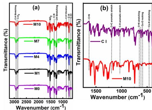
Fig. 4 (a) FTIR spectra (3200–600 cm<sup>-1</sup>) of the membrane with the content of CI (M0, M1, M4, and M7) and without the content of CI (M10). (b) FTIR spectra (1750–450 cm<sup>-1</sup>) of CI and the membrane M10.
