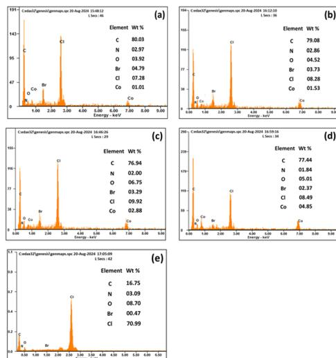
Fig. 7 Quantitative EDS analysis with CI (a) M0, (b) M1, (c) M4, (d) M7 and without the CI membrane (e) M10.
