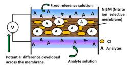
Fig. 14 Sensing mechanism for the membrane.
