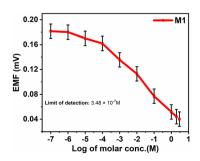
Fig. 10 Graph of emf versus the logarithm of analyte concentration for the M1 membrane.
