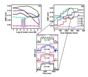
Fig. 9 (a) EMF characteristic and (b) dynamic response time of the nitrite ISE based on variable CI wt% (M0, M1, M4, M7) and virgin M10 (inset).
