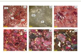
Fig. 8 Optical microscopy images for the membrane (a) with CI and (b) without CI at low magnification scan; (c) M0, (d) M1, (e) M4, (f) and M7 at high magnification scan.
