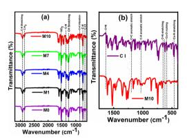
Fig. 4 (a) FTIR spectra (3200-600 cm<sup>-1</sup>) of the membrane with the content of CI (M0, M1, M4, and M7) and without the content of CI (M10). (b) FTIR spectra  $(1750-450 \text{ cm}^{-1})$  of CI and the membrane M10.
