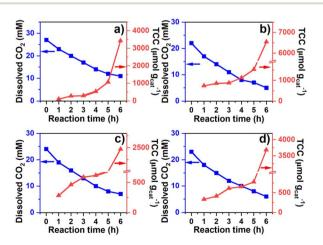
Fig. 4 Effect of reaction time to dissolved CO<sub>2</sub> concentration and TCC corresponding to (a) water, (b) methanol, (c) ethanol, and (d) isopropanol SCRs.
