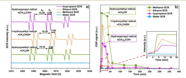
Fig. 7 (a) ESR spectra corresponding to CO<sub>2</sub> photoreduction in the presence of methanol, ethanol, and isopropanol SCRs, and (b) ESR peak intensity changes with respect to time.
