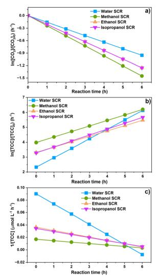
Fig. 5 The kinetics of dissolved CO<sub>2</sub> concentration (a): product generations in water, methanol, ethanol, and isopropanol SCRs as analyzed by (b) the first-order reaction and (c) second-order reaction.
