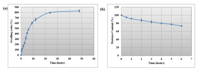
Fig. 3 (a) Swelling ratio of hydrogels as a function of time at 25 °C; each point represents the mean  $\pm$  SD (n=3). (b) Moisture content as a function of time at 25 °C.
