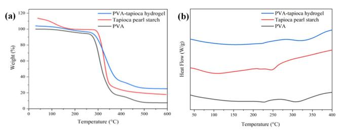
Fig. 5 (a) TGA thermograms of PVA, tapioca pearl starch and PVA-tapioca hydrogels. (b) DSC thermograms of PVA, tapioca pearl starch and PVA-tapioca hydrogels.
