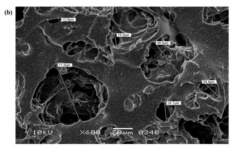
Fig. 2 Scanning electron micrographs of PVA-tapioca hydrogel at different magnifications. Hydrogels have porous structures with interconnected pore network. Scale bars: (a)  $50 \mu m$  (b)  $20 \mu m$ .
