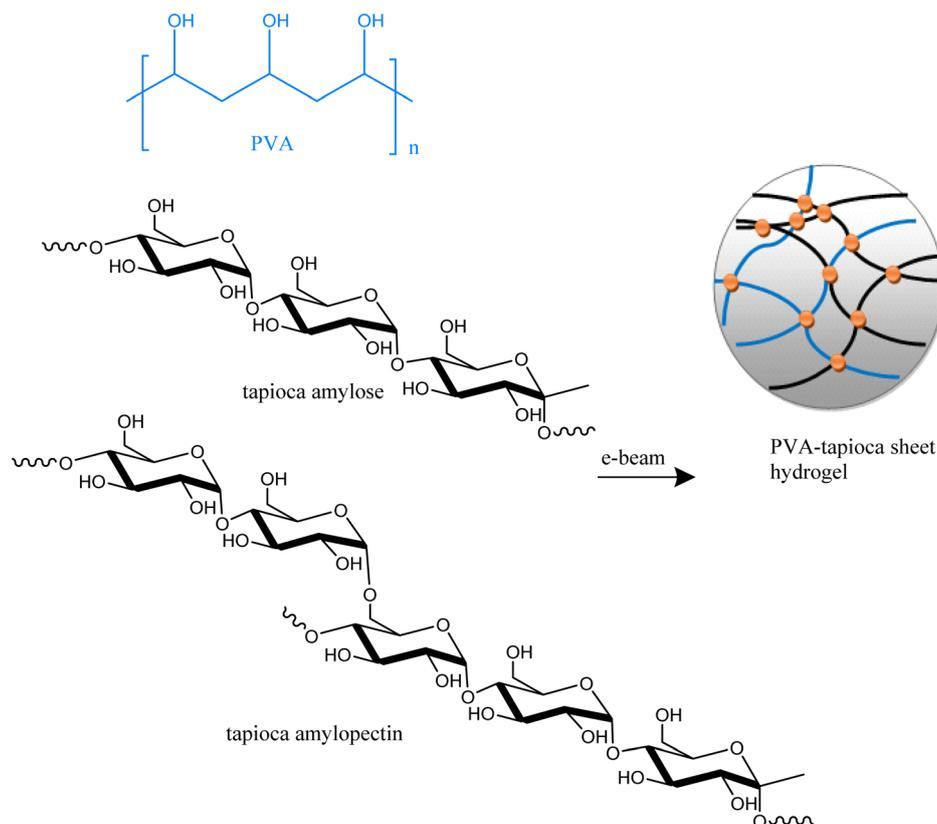
Scheme 1 Fabrication of PVA–tapioca pearl hydrogels via electron beam crosslinking.
