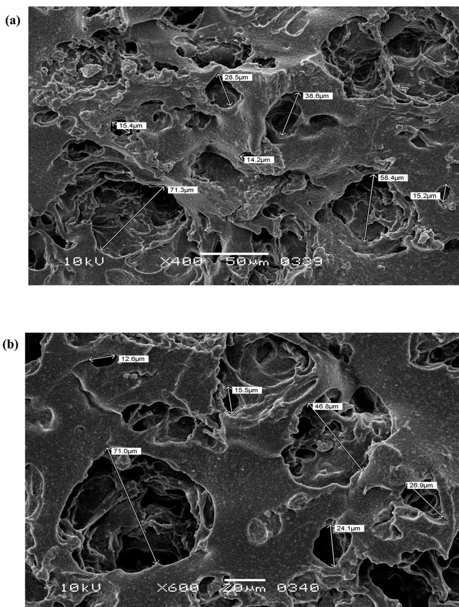
Fig. 2 Scanning electron micrographs of PVA–tapioca hydrogel at different magnifications. Hydrogels have porous structures with interconnected pore network. Scale bars: (a) 50  $\mu\text{m}$  (b) 20  $\mu\text{m}$ .
