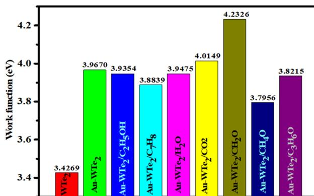
Fig. 11 Comparative analysis of work function for WTe<sub>2</sub> and Au-decorated WTe<sub>2</sub> before and after exposure to volatile organic compounds (VOCs).
