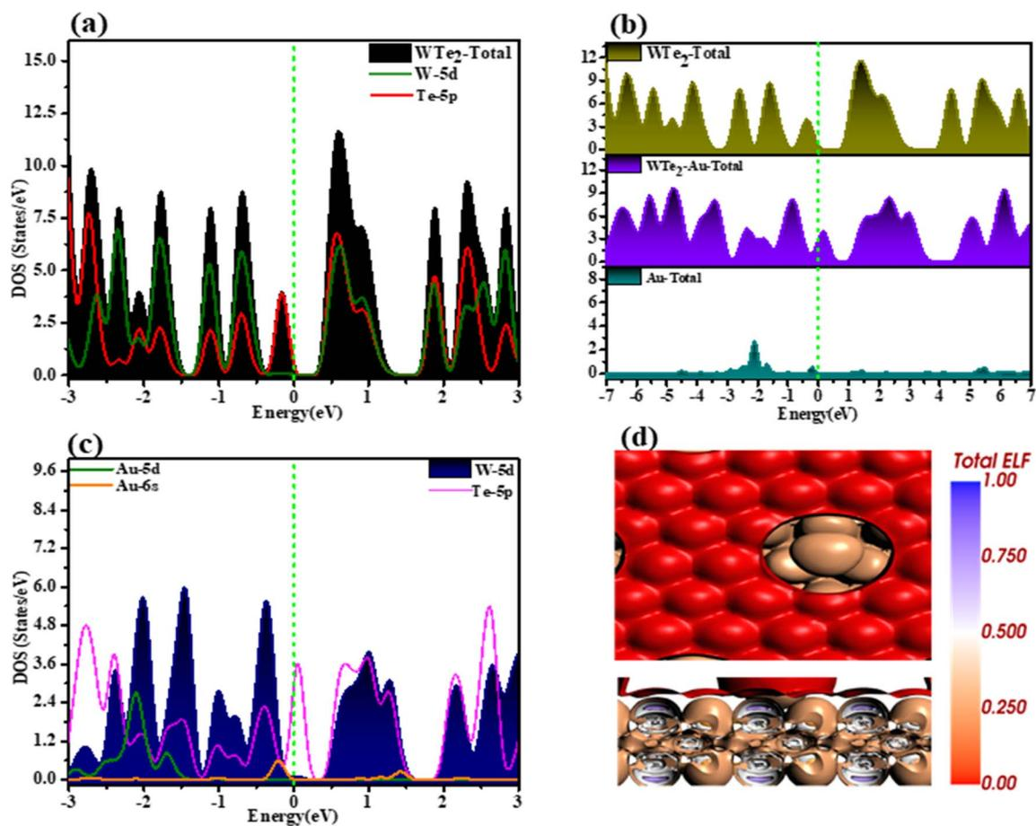
Fig. 2 (a–c) TDOS and PDOS curves of pristine  $\text{WTe}_2$ , Au-decorated  $\text{WTe}_2$ , and green dashed lines are Fermi level, (d) ELF of Au- $\text{WTe}_2$ .
