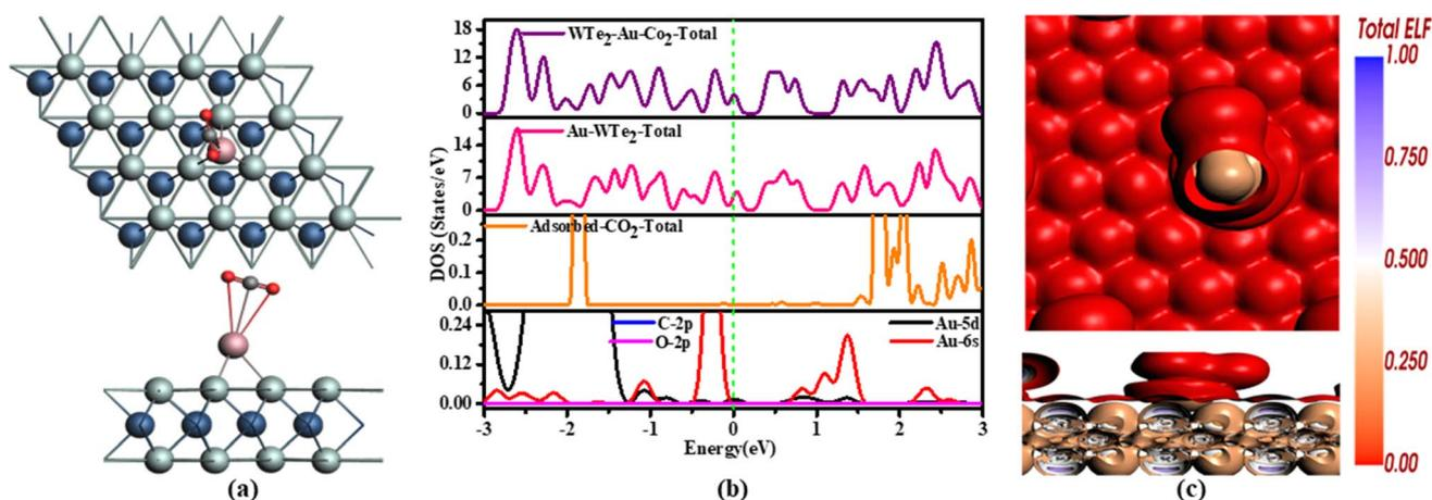
Fig. 7 (a) Configuration of CO<sub>2</sub> adsorption (b) TDOS and PDOS (c) ELF of CO<sub>2</sub>.
