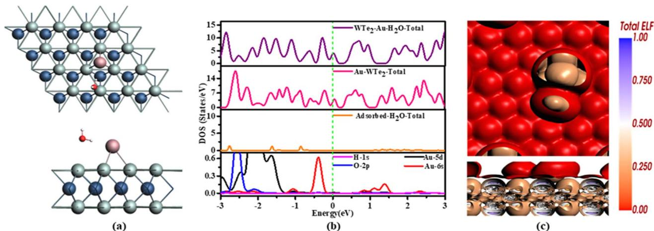
Fig. 6 (a) Configuration of H<sub>2</sub>O adsorption (b) TDOS and PDOS (c) ELF of H<sub>2</sub>O.
