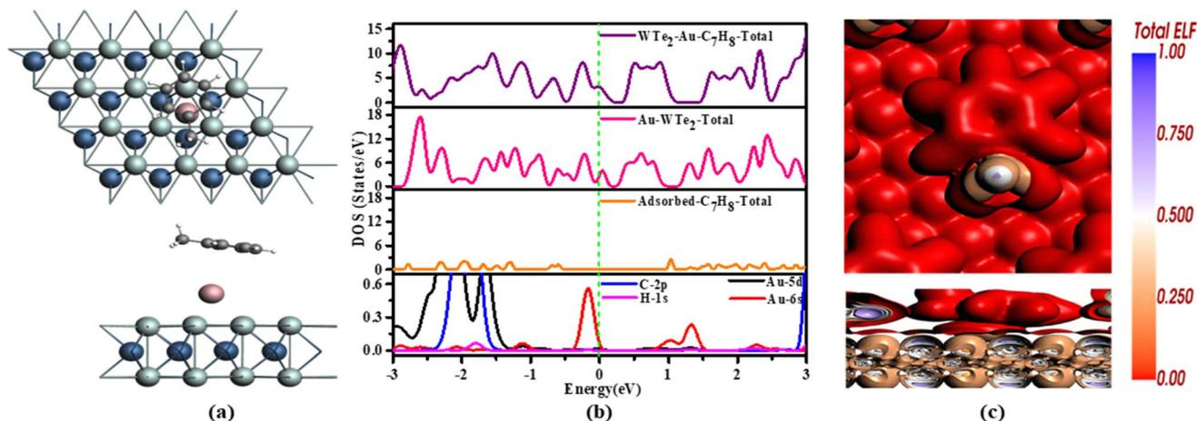
Fig. 3 (a) Configuration of C<sub>7</sub>H<sub>8</sub> adsorption (b) TDOS and PDOS (c) ELF of C<sub>7</sub>H<sub>8</sub>.
