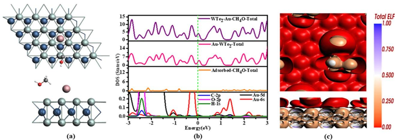
Fig. 8 (a) Configuration of CH<sub>4</sub>O adsorption (b) TDOS and PDOS (c) ELF of CH<sub>4</sub>O.
