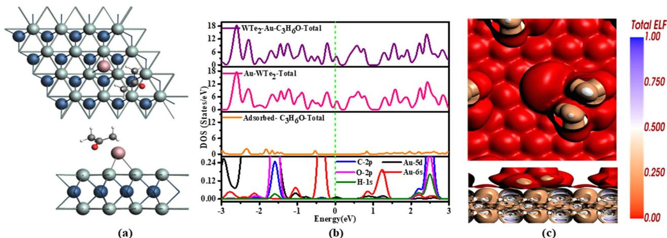
Fig. 5 (a) Configuration of C<sub>3</sub>H<sub>6</sub>O adsorption (b) TDOS and PDOS (c) ELF of C<sub>3</sub>H<sub>6</sub>O.
