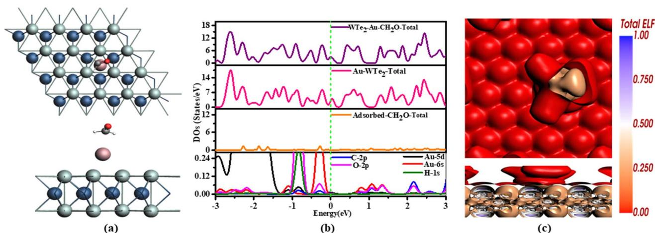
Fig. 4 (a) Adsorption configuration of CH<sub>2</sub>O (b) TDOS and PDOS (c) ELF of CH<sub>2</sub>O.
