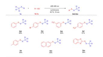
Scheme 3 Cross coupling between trichloromethyl sulfenyl chloride (1a) and different sulfenyl chlorides. a,b a Reaction conditions: substrate (1 mmol), 1a (2 mmol), cyclohexane (3.3 mL), LED 405 nm, 35 °C, 15 minutes. b Isolated yield base on the aryl sulfenyl chloride (R-SCI)
