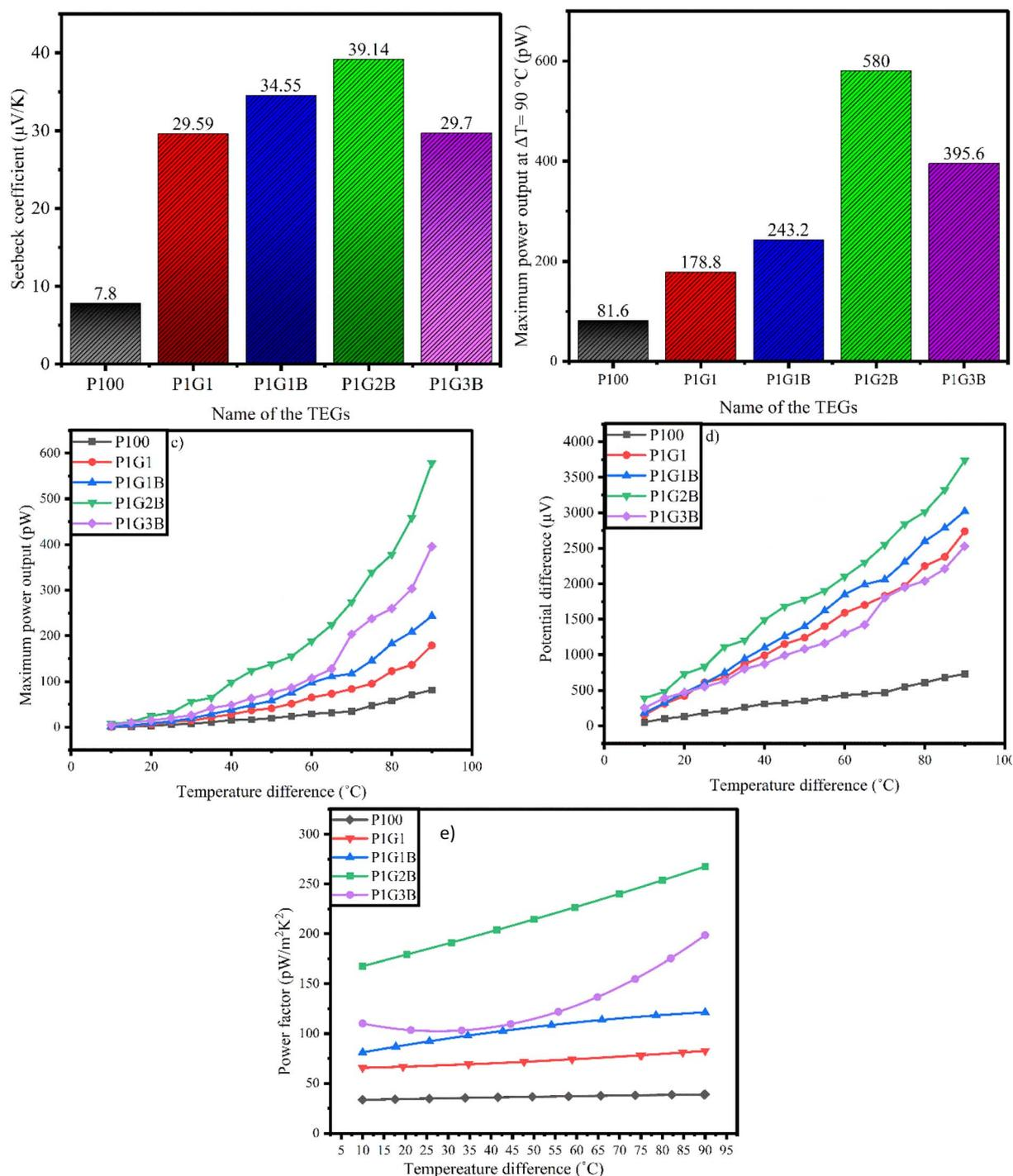
Fig. 8 (a) Seebeck coefficient, (b) maximum power output at  $\Delta T = 90^\circ\text{C}$  of the printed FTEGs, (c) maximum power output, (d) potential difference, and (e) power factor vs. temperature difference of FTEGs.
