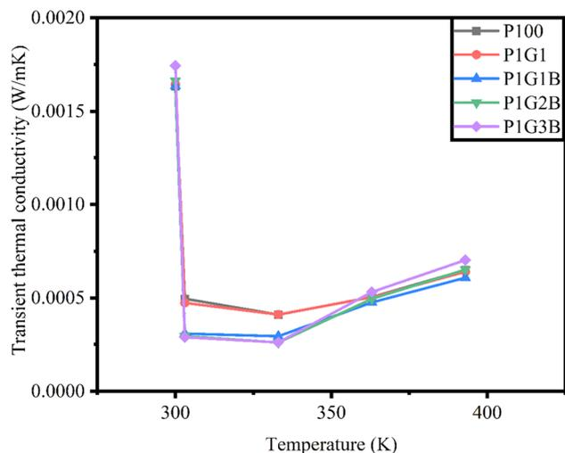
Fig. 7 Transient thermal conductivity of TEGs.
