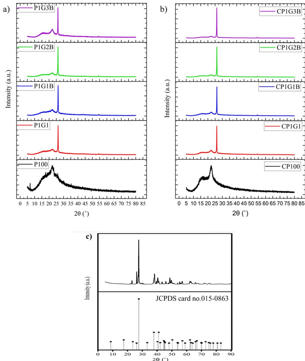
Fig. 2 XRD peak patterns of (a) inks, (b) composites and (c) bismuth telluride.
