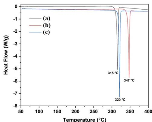
Fig. 12 TG thermograms of compounds **4a** (R<sup>1</sup> = Me), **4b** (R<sup>1</sup> = Br), and **4c** (R<sup>1</sup> = Cl).
