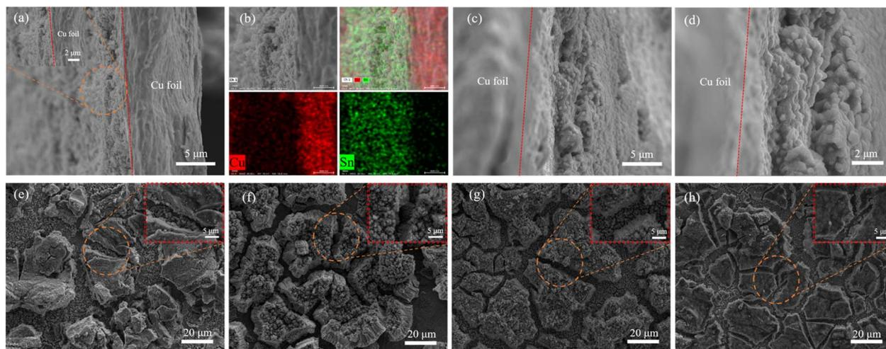
Fig. 8 The before (a and b) and after (c and d) the circulation cross-section SEM images of S2 electrode and SEM images of S1 (e), S2 (f), S3 (g), and S4 (h) after the circulation.
