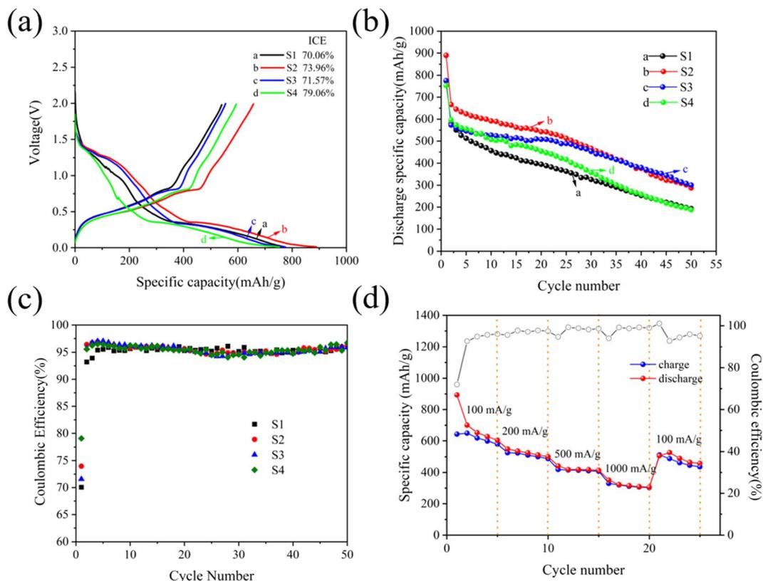
Fig. 4 Initial galvanostatic charge and discharge curves (a) and cycling performance curves (b and c) of S1, S2, S3 and S4 electrodes at  $100 \text{ mA g}^{-1}$ ; rate performance (d) of the S2 electrode at various current densities.
