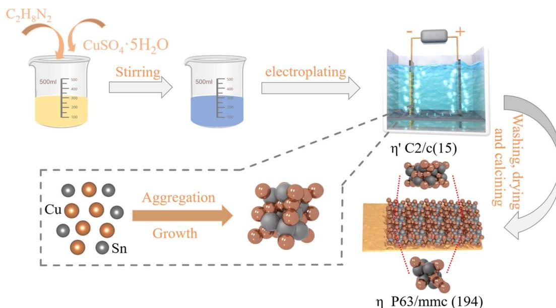
Fig. 1 Schematic diagram of the fabricated Cu<sub>6</sub>Sn<sub>5</sub> alloy electrodes.
