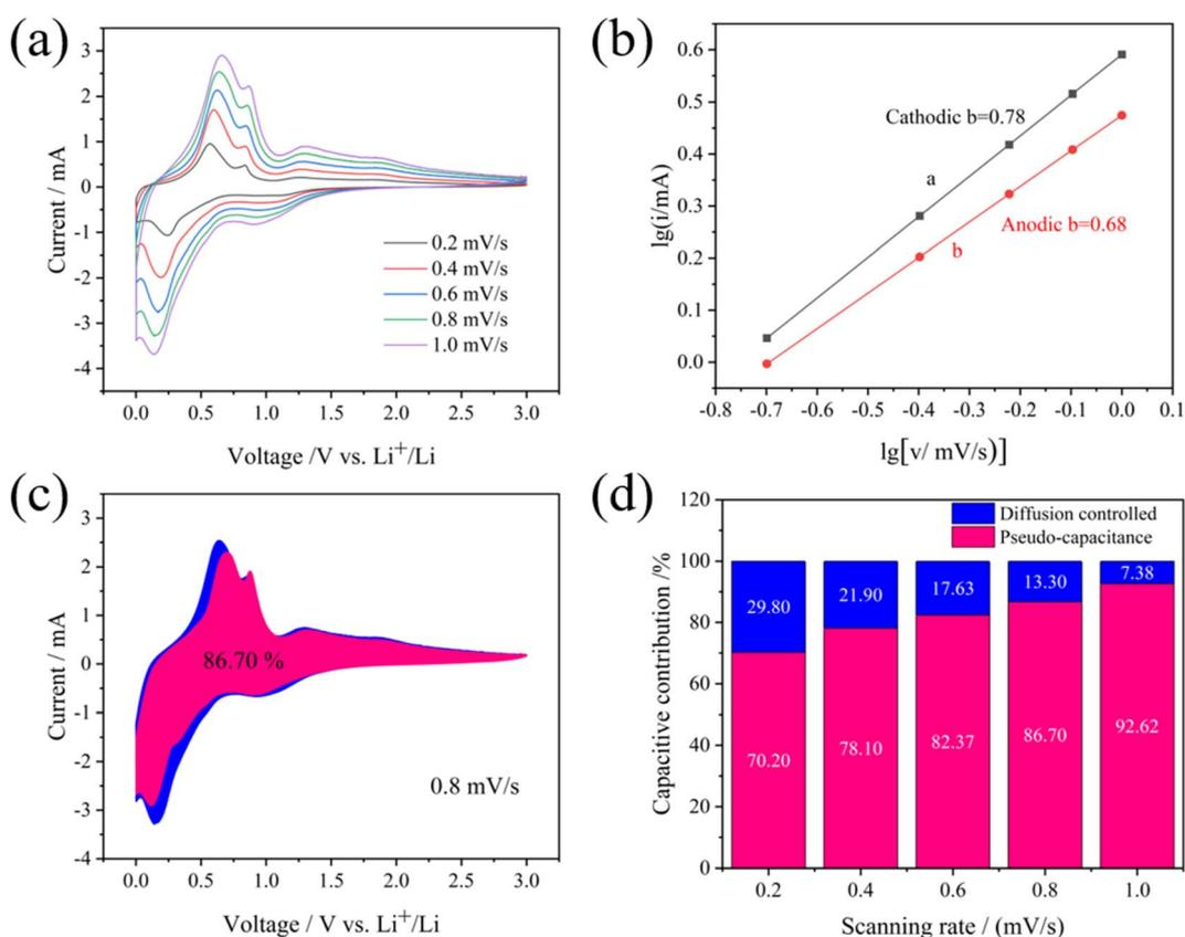
Fig. 6 CV curves at various scan rates from 0.2 to 1.0  $\text{mV s}^{-1}$  (a), logarithmic relationship between peak currents and scan rates (b), the proportion of pseudocapacitance at 0.8  $\text{mV s}^{-1}$  (c) and contribution ratios of pseudocapacitive and diffusion-controlled process at given scan rates (d) of the S2 electrode.
