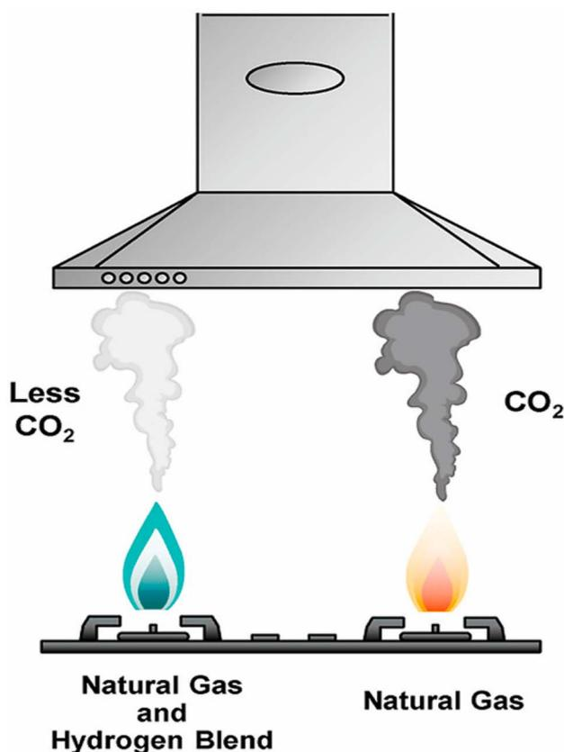
Fig. 7 Illustration of the benefit from blending green H<sub>2</sub> with natural gas.<sup>141</sup>
