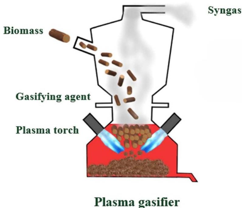
Fig. 3 Representation of the production of green H<sub>2</sub> with plasma route.<sup>75</sup>
