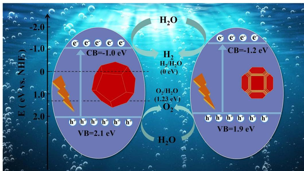
Fig. 6 Schematic diagram of photocatalytic water splitting of samples.<sup>93</sup>
