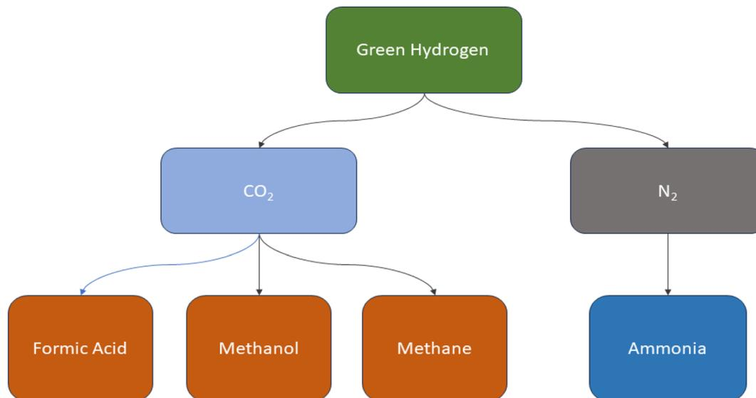
Fig. 9 Showing the different chemical products that can be generated by green H<sub>2</sub>.
