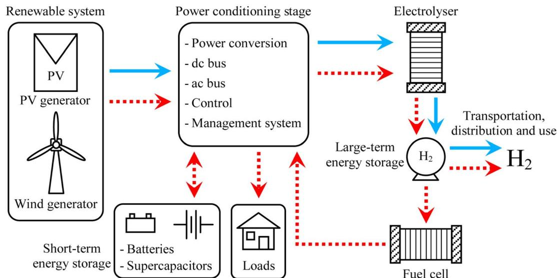
Fig. 4 Configurations for the integration of electrolyzers with renewable energies in stand-alone systems.<sup>86</sup>
