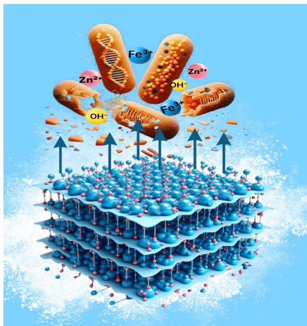
Scheme 3 Mechanism for the antibacterial activity of the ZnFe-LDH.
