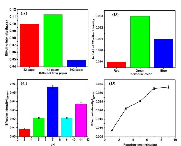
Fig. 4 (A) Selection of the paper using RGB intensity and (B) the selection of the individual intensity (30  $\mu$ M). (C) Graph showing the signal intensity change with the reaction time (selected for pH 7, 30  $\mu$ M). (D) Graph showing the signal intensity change with the reaction time (selected for 9 minutes, 30  $\mu$ M).
