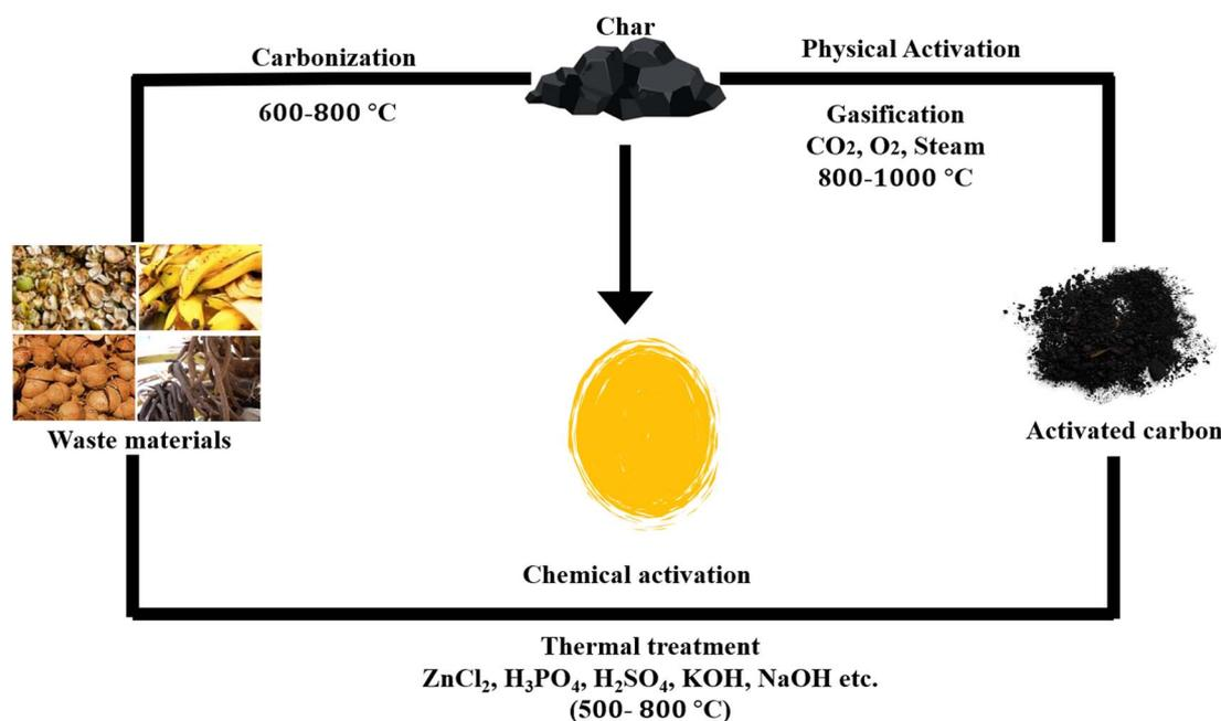
Fig. 9 Process for the synthesis of activated carbon.
