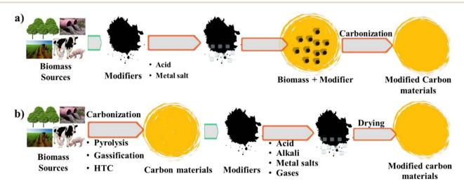
Fig. 7 Schematic illustrating the two primary approaches for modifying carbon materials: (a) pre-treatment and (b) post-treatment methods.
