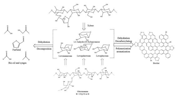
Illustration of the breakdown mechanism of hemicellulose during pyrolysis and subsequent biochar formation.
