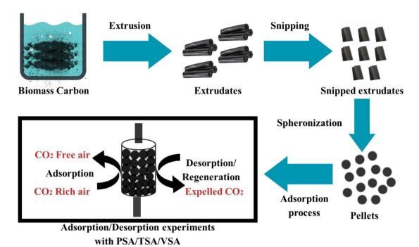
Fig. 16 Diagram illustrating the complete CO<sub>2</sub> capture process, starting from powder form to palletization, and depicting the sorption cycle for real-world application.
