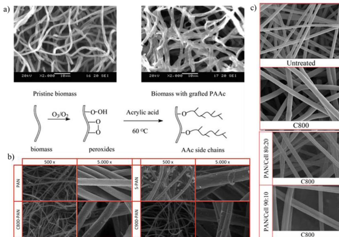
Fig. 15 Surface morphology of biomass and polyacrylonitrile (PAN)-based nanofibers for enhanced CO<sub>2</sub> capture: (a) pristine vs. PAAc-grafted biomass, (b) SEM comparison of untreated PAN, C800, and PAN/C800 composites, and (c) PAN nanofiber morphology under varying treatments and magnifications. Reproduced from ref. 322 and 323.
