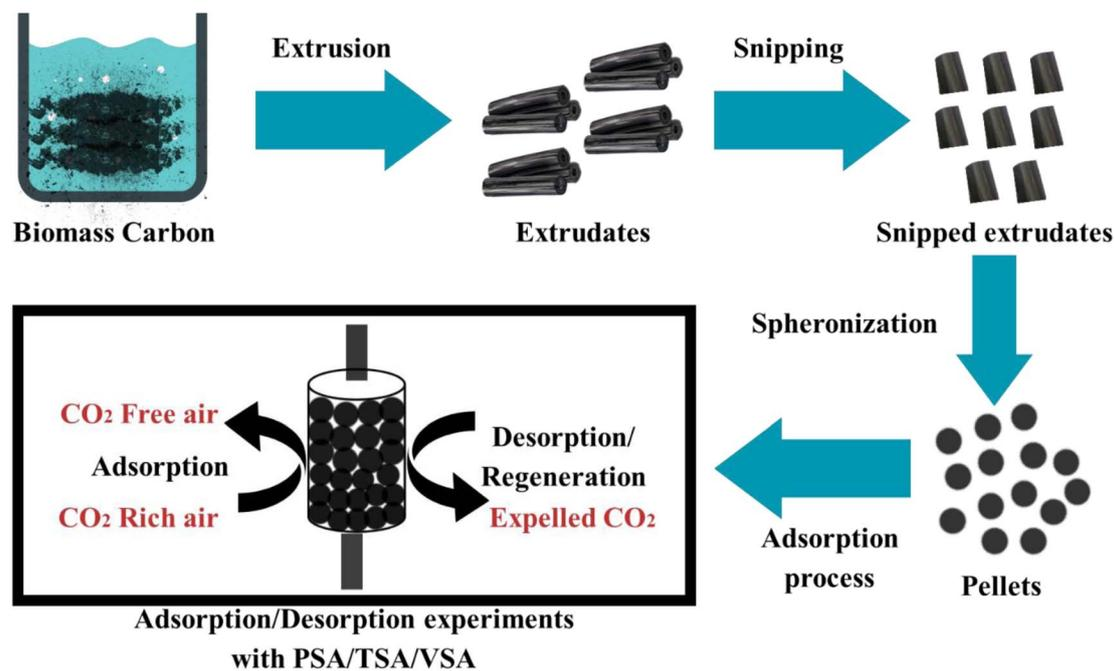
Fig. 16 Diagram illustrating the complete CO<sub>2</sub> capture process, starting from powder form to palletization, and depicting the sorption cycle for real-world application.
