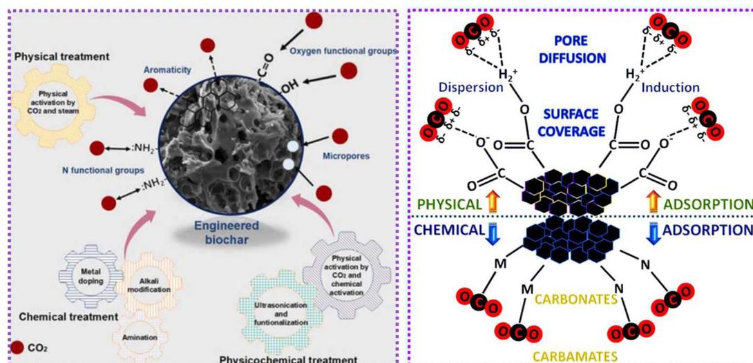
Fig. 14 Processes involved in CO<sub>2</sub> capture by carbon materials. Reprinted with permission.<sup>269,295</sup>
