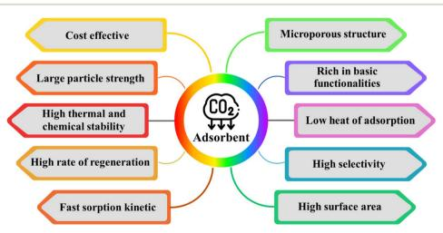
Fig. 1 Properties of activated carbon for carbon dioxide capture.
