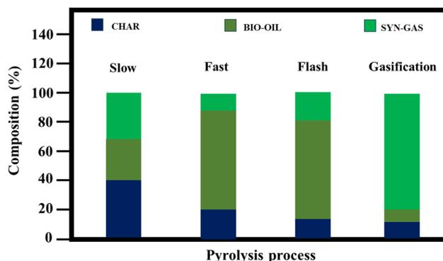
Fig. 4 Proportional breakdown of char, bio-oil, and syngas produced through various pyrolysis methods.
