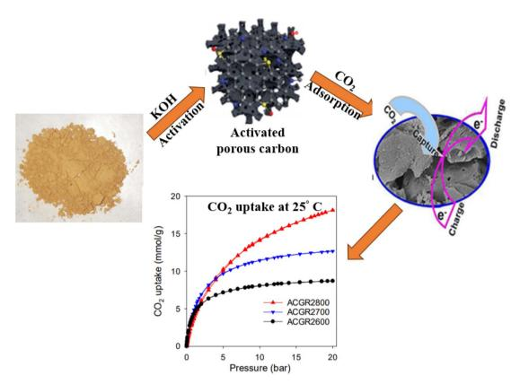
Fig. 11 CO<sub>2</sub> adsorption performance of KOH-activated biomass-derived porous carbon.<sup>276</sup>
