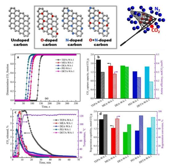
Fig. 12 Heteroatom-doped carbons for  $CO_2$  capture and  $CO_2$  adsorption performance of wood ash (WA-1) activated with various polyamines, showing (a)  $CO_2$  adsorption breakthrough profiles, and (b) adsorption capacity along with amine efficiency. Regeneration performance of WA-1 activated with different polyamines: (c)  $CO_2$  desorption curves, and (d) adsorbent regeneration potential and conversion efficiency. Reprinted with the permission. <sup>265,286</sup>
