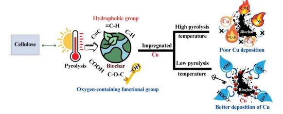
Schematic showing the relationship between hydrophilicity and functional development of biochar. Reproduced from ref. 34
