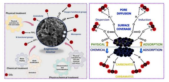
Fig. 14 Processes involved in CO<sub>2</sub> capture by carbon materials. Reprinted with permission.<sup>269,295</sup>
