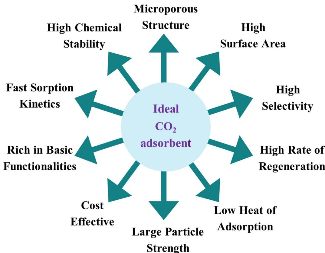
Fig. 10 Characteristic properties required for an ideal adsorbent for CO<sub>2</sub> capture.
