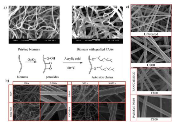
Fig. 15 Surface morphology of biomass and polyacrylonitrile (PAN)-based nanofibers for enhanced CO<sub>2</sub> capture: (a) pristine vs. PAAc-grafted biomass, (b) SEM comparison of untreated PAN, C800, and PANC/cell composites, and (c) PAN nanofiber morphology under varying treatments and magnifications. Reproduced from ref. 322 and 323.
